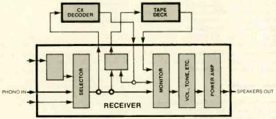
Fig. 1B: Signal path when switched for playing standard non-CX-encoded LPs
