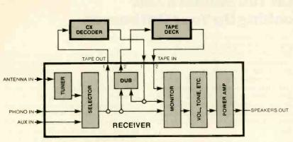
Fig. 1A: A simple receiver-based system with one-way dubbing switch, CX decoder, and one tape deck
