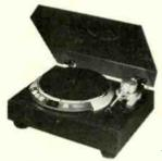
The beautifully finished, massively built Denon DP-60L turntable this year receives a new arm and a new model number, DP-62L. Dubbed Servo Tracer, the arm responds automatically to vertical and horizontal displacements caused by warped LPs, generating a counter force sufficient to prevent excessive infrasonic output. Denon says that just about any phono cartridge can be mated to the arm with little fear of warp-induced mistracking. The upgraded turntable is priced at \$600.
