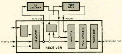
Fig. 1C: Signal path when switched for playing CX-encoded LPs
