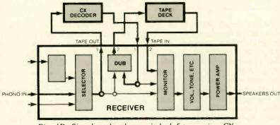
Fig. 1D: Signal path when switched for copying CX-encoded LPs
