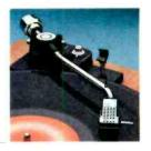
Unlike the tonearm in most direct drive turntables, the slender arm of the DD75 is extremely low in mass—just 16 grams. It rides effortlessly on jewel bearings, with friction so low that it will track the finest cartridges at their minimum rated stylus pressure.
