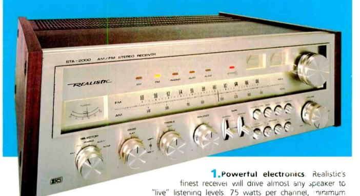
total harmonic distortion. Sensitive dual-gate MOSFET tuner with PLL circuitry. The phono preamp has differential circuitry for a high overload margin.
