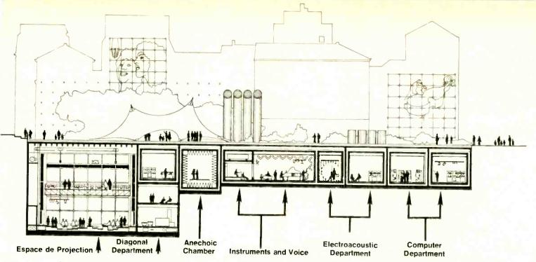
A cutaway view of IRCAM. Note the hoists for the Espace de Projection ceiling, adjustable in three independent sections. The Instruments and Voice rooms include recording studios, depicted here during a session. Above the recording console area are vent pipes. The artist has included ideas for decorating the barren walls that will enclose the IRCAM plaza.
