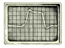
This special pulse is used in the Time-Align™ Technique to create the most accurate acoustic reproducers you've ever heard. Each of the components of a complex acoustical wave are presented to the listener with exactly the same time relationships they had in the original sound.
