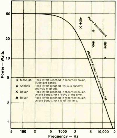
This curve shows the maximum power output of a 50-watt amplifler when fed from conventional FM. The power curve and the power requirement points are all shown with respect to full mid-frequency modulation at the transmitter and 50 watts peak power from the amplifier.
