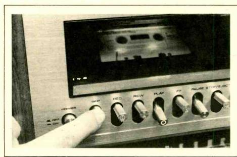
Unusual feature is SKIP button, which approximately doubles playback speed as an aid in searching for desired passage. Feature is inoperative in recording.
