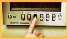
Switch from one mode to another, bypassing the Stop-lever.
