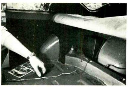
Left, author installing four-channel/two channel player in his sportscar. The Toyo CS 721 player comes with a full-length negative lead which simplifies its installation in vehicles in which the structure is not used as ground side of electrical circuitry (some cars, all boats, and aircraft). Two speakers were mounted under the car's rear deck (above photo), and two more were installed under the dashboard.
