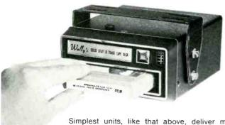
Simplest units, like that above, deliver mono sound from stereo cartridges via the amplifier and speaker of car's AM radio. Most units mount on a bracket below the dashboard. . .
