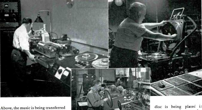
Above, the music is being transferred from tape to disc. Microscope at the operator's hand permits precise inspection of the record grooves. In the center illustration, a master
