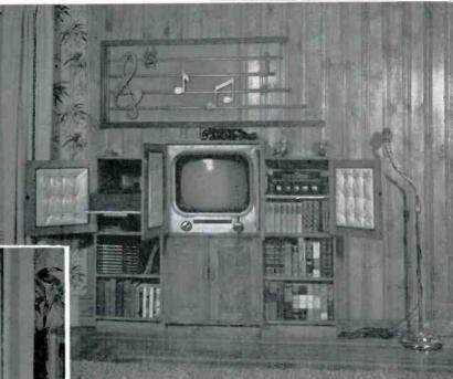
provided housing for the Altec 604-B with about 30 cu. ft. of closed baffle space and, directly below, enough space for the Radio Craftsmen TV tuner. The remaining equipment consists of a Garrard changer, RC-10 tuner, Ampex 400 recorder, Brook 10-watt amplifier, and a Shure 55-S microphone. Needless to say, the expanse of leather armchair next to the Ampex houses yours truly at practically every leisure moment."
