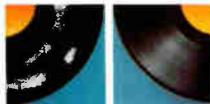
(Left) Styrofoam heads are attracted to static charge left on record after cleaning with Discwasher D3 ®
