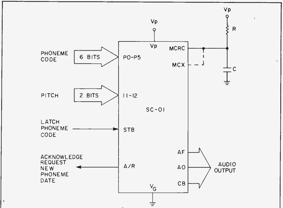
Fig. 1. This flow diagram of the Votrax SC-01 chip illustrates the complexity of this talking IC. Phoneme, pitch, latch and other codes are used to get a good audio output.
