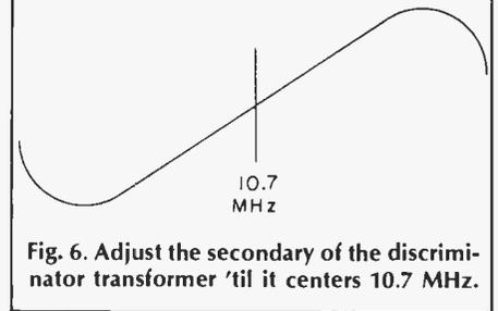
Fig. 6. Adjust the secondary of the discriminator transformer 'til it centers 10.7 MHz.
