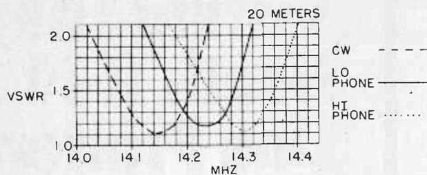
Fig. 1. The lowest standing wave ratio is 1.1 to 1 increasing to 1.5 to 1 at 14.16 and 14.3 MHz. A-1 sounds can be heard with this.
