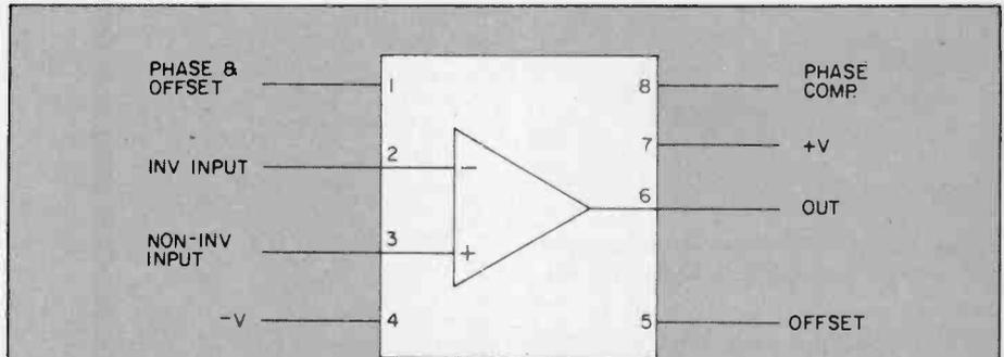
Fig. 1. The CA080E configuration is mounted in an eight-lead mini-dip case, with inverting at pin 2, non-inverting at pin 3.
