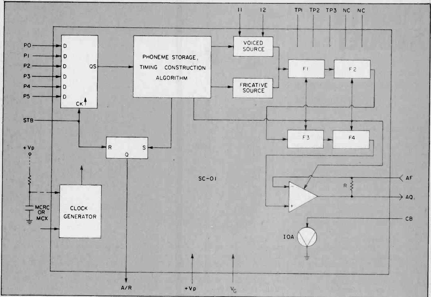
The above block diagram illustrates the various interconnections in the Votrax SC-01 speech synthesizer chip. Through a very complicated process, electronic commands are sorted, amplified and given tonal characteristics. The chip emits a versatile voice.
