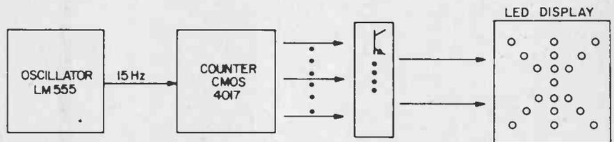
Fig. 1. Only two integrated circuits are used to create this colorful flashing display. A counter, an oscillator and 19 LEDs are all that are really needed. An inexpensive project, Star-nament adds life to any holiday. This project can be constructed by using either wire winding techniques or by purchasing the PC board from Niccum Electronics.
