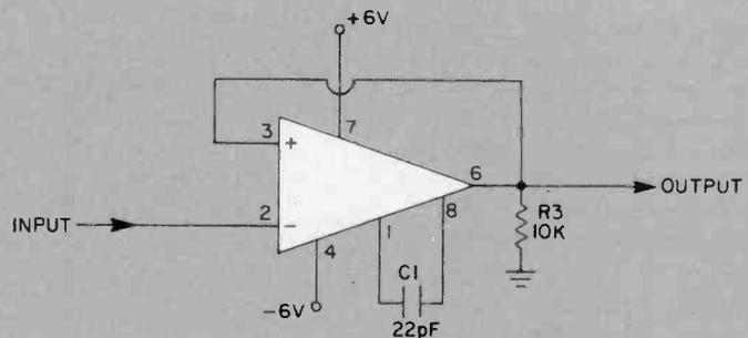
Fig. 2B is the amplifier circuit design most commonly used with the RCA BiMos. It saves space, is more flexible in organization.
