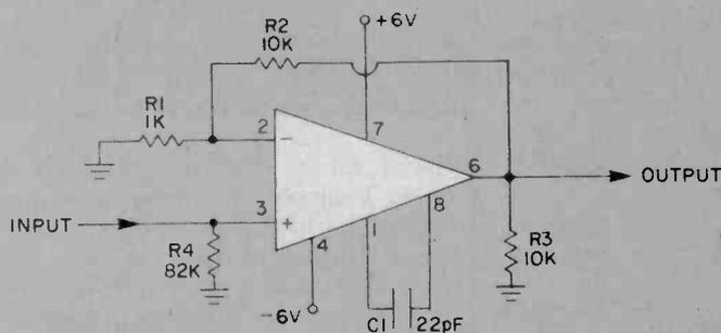
Fig. 5. Note that input signal is now applied to the non-inverting input + pin 3 on IC chip.
