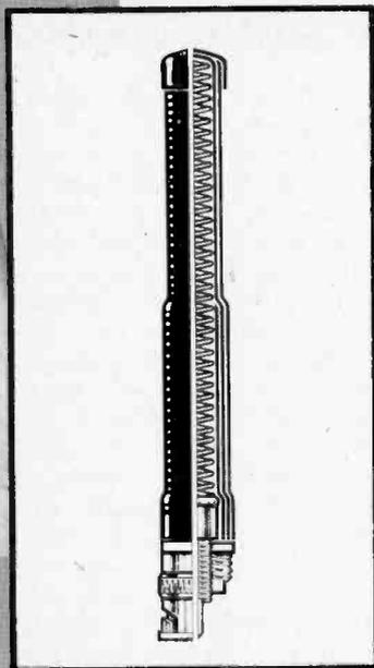
By using air wound copper wire, Poly-Olifin shrinktubing as insulation and many other clever features, Larsen Electronics has built a superb antenna.
