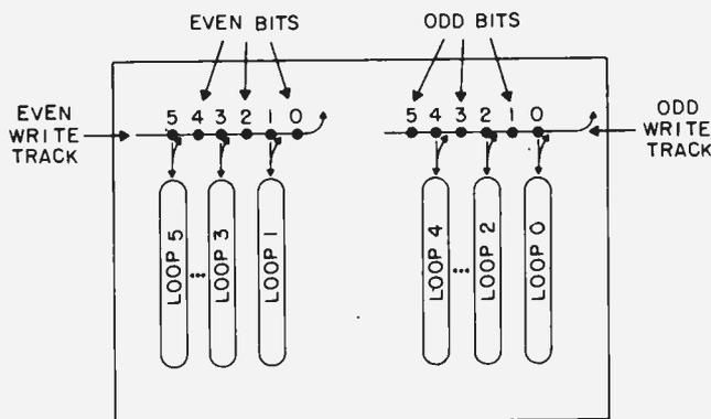
Fig. 6. The data storage area is divided into odd and even storage banks.
