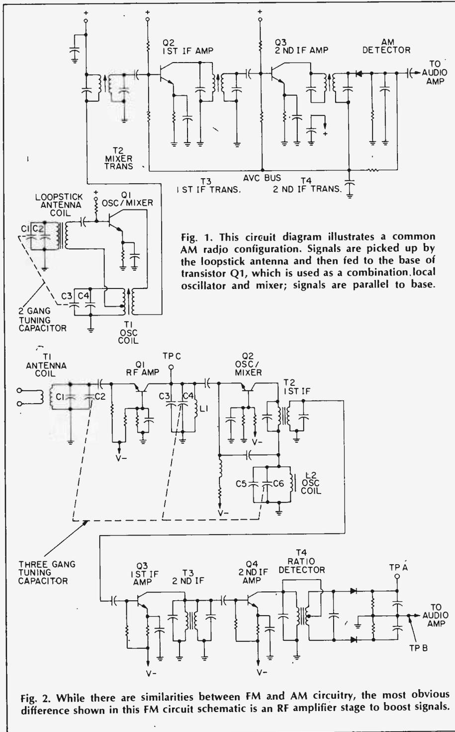
Fig. 1. This circuit diagram illustrates a common AM loopstick configuration. Signals are picked up by the loopstick antenna and then fed to the base of transistor Q1, which is used as a combination local oscillator and mixer; signals are parallel to base.
