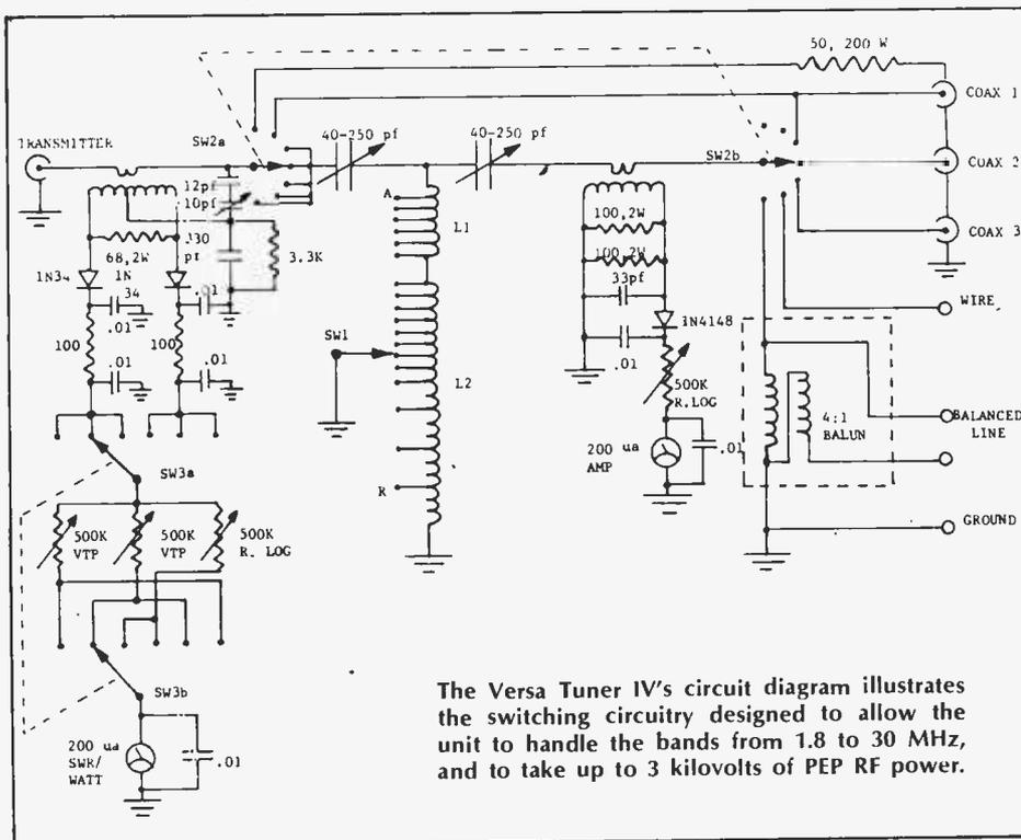
The Versa Tuner IV's circuit diagram illustrates the switching circuitry designed to allow the unit to handle the bands from 1.8 to 30 MHz, and to take up to 3 kilovolts of PEP RF power.
