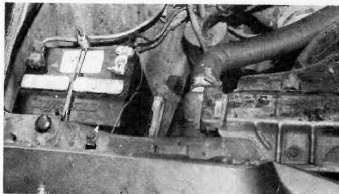
screws gave the battery a snug seat in the tray. The original tie-down rods were used again because they were serviceable. However, the tie-down rod that rested on top of the battery was not, so we fashioned some 3/16 in. steel rod to replace the unusable part.
