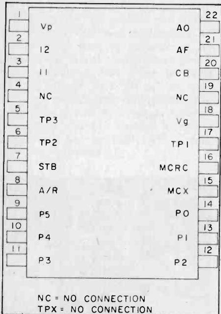
Fig. 2. This shows the placement of each pin in the Votrax SC-01. P0-P5 are the phoneme command points. I1-I2 give the electronic word tones or inflections. Input STB controls latching. AF, AO and CB are audio outputs. MCX and MCRC are timing controls. A/R acknowledges receipt of phoneme data.
