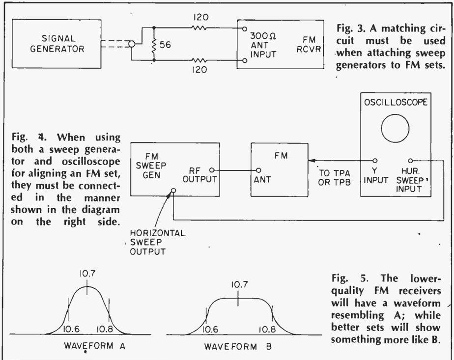
Fig. 4. When using both a sweep generator and oscilloscope for aligning an FM set, they must be connected in the manner shown in the diagram on the right side.
