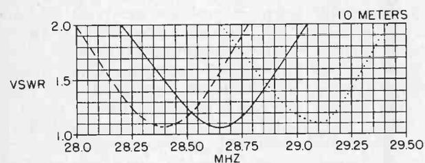
Fig. 3. For 10 meters, the curve spreads out more than the other curves do and hits its lowest point of 1.07. By far this is the best.
