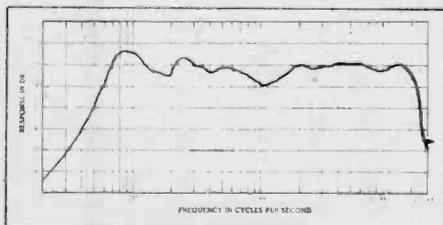
This diagram shows frequency response of the poly-Planars from 40 Hz to 20 kHz.
