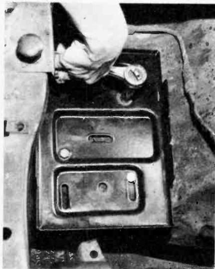
Putting in a battery pan is easy but do it right. Make sure the pan is level and secure.
