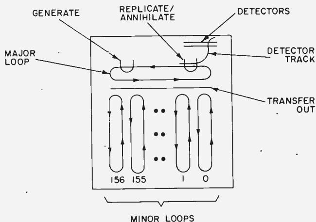
Fig. 5. This is a block diagram of the major/minor loop organization of Texas Instruments' T1B0203 92 kbit bubble memory. For reading, data is transferred from the minor to the major loops.
