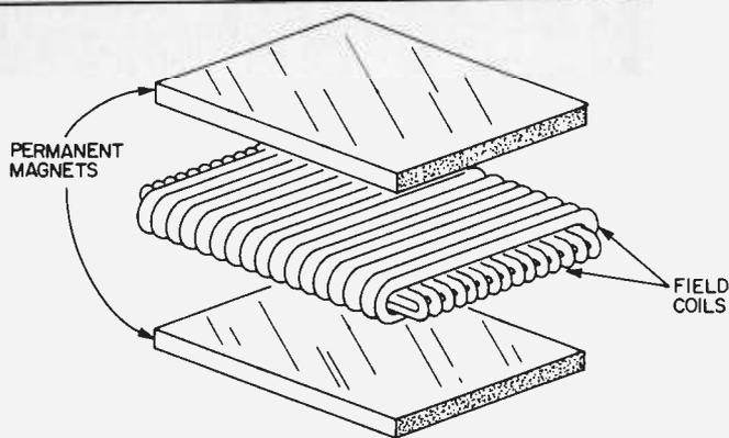
Fig. 4. Field coils and permanent magnets determine the direction of the bubbles as they move. Thus, a serial shift register is created.
