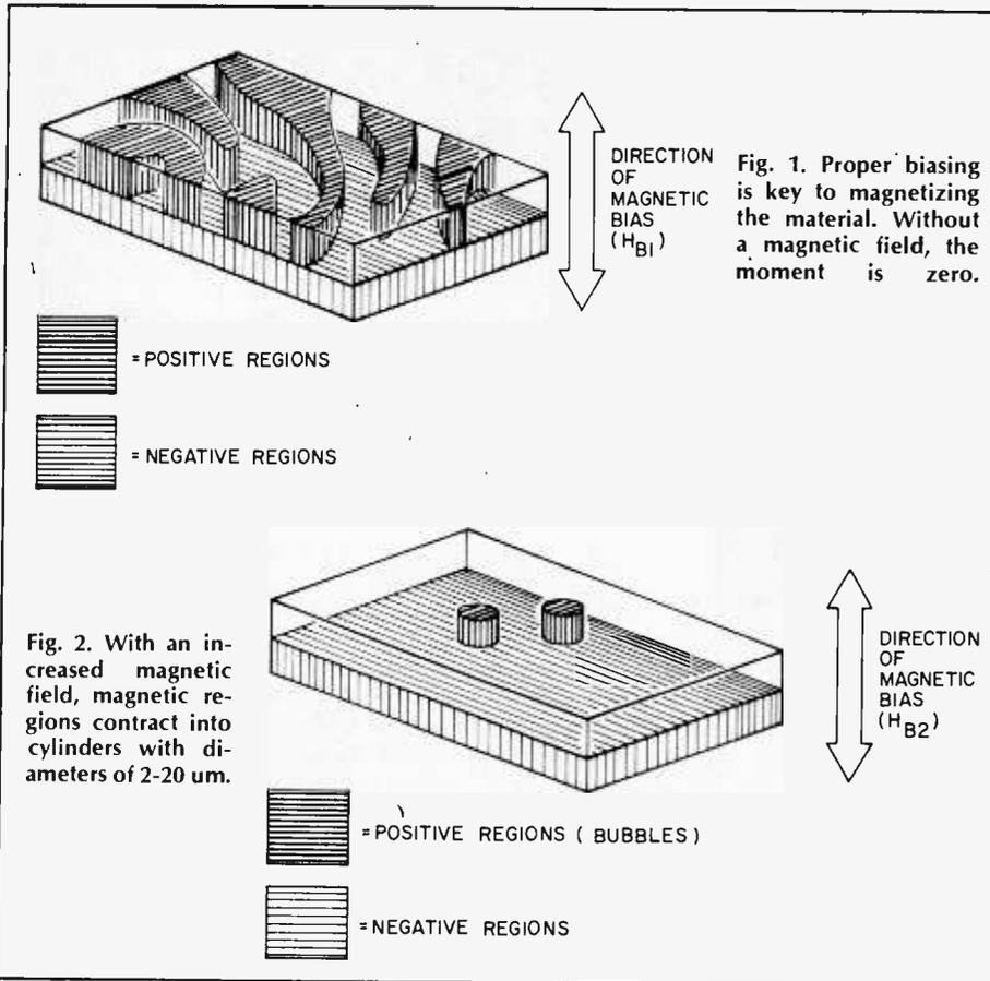
Fig. 1. Proper biasing is key to magnetizing the material. Without a magnetic field, the moment is zero.
