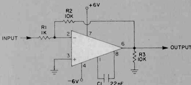
Fig. 3B. Gain is determined by placing resistors R1 and R2 between the input and output.
