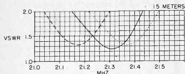
Fig. 2. The curve for the standing wave ratio at 15 meters also bottoms out at 1.1 to 1. It hits 1.5 to 1 at frequencies 21.23 MHz and 21.38 megahertz.
