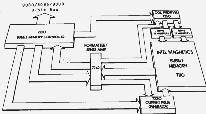
Fig. 7. Support large scale integration (LSI) circuits available with the Intel 7110 megabit bubble memory chip turn the memory module into a complete storage system.
