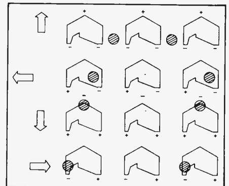
Fig. 3. By applying a rotating magnetic field, bubbles can be made to move. To be useful bubbles must be totally manipulated.
