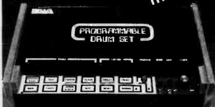
Our Popular Programmable Drum Set's simple programming system allows even first time users to structure bass, tom, snare, wood-block and cymbal sounds into any rhythm in any time signature. Versatile memory organization provides simultaneous storage of two separate rhythm patterns each with its own bridge rhythm. Bridges are activated from either the control panel touch plate or optional foot switch and are automatically synchronized to the main rhythm.
