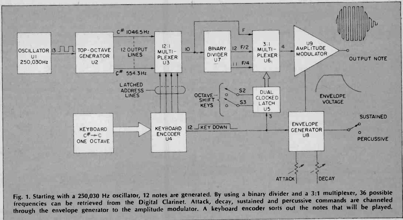
Fig. 1. Starting with a 250,030 Hz oscillator, 12 notes are generated. By using a binary divider and a 3:1 multiplexer, 36 possible frequencies can be retrieved from the Digital Clarinet. Attack, decay, sustained and percussive commands are channeled through the envelope generator to the amplitude modulator. A keyboard encoder sorts out the notes that will be played.
