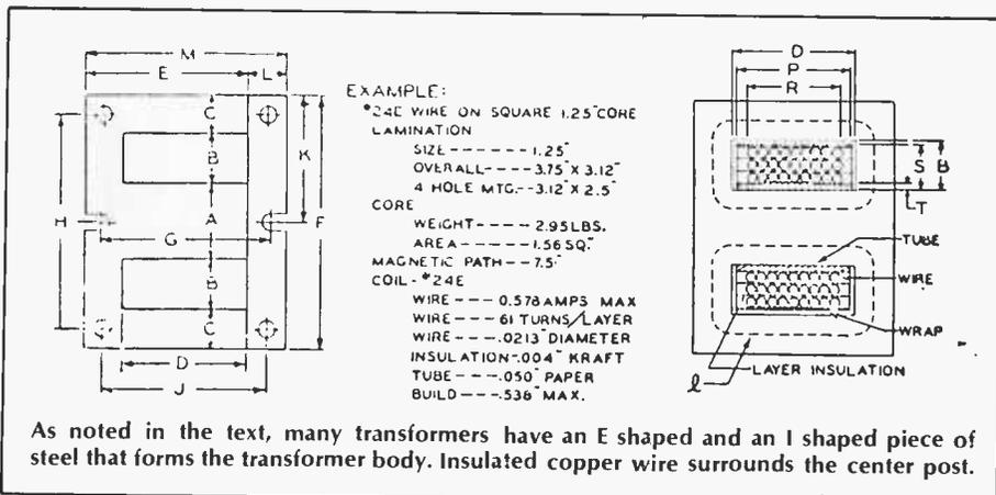
As noted in the text, many transformers have an E shaped and an I shaped piece of steel that forms the transformer body. Insulated copper wire surrounds the center post.
