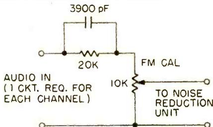
Adding Dolby without quite having enough cash or credit to get a new Dolby tuner, like the Lafayette, is possible with one of the "outboard" Dolby units and this simple home-made network. "FM Cal" is to be set so "Dolby Tone" from station gives "Dolby Level" reading on meter(s) of the noise reduction unit you are utilizing.
