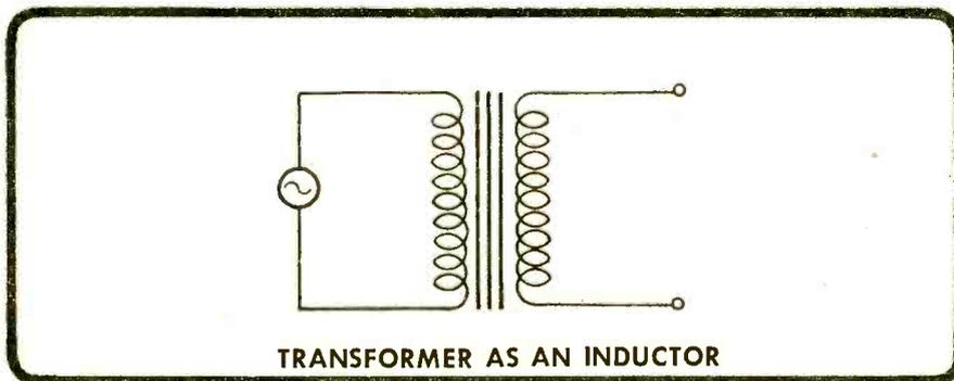
The difference in the number of turns is known as the *turns ratio* of the transformer. If the primary winding has  $N_1$  turns and its voltage is  $E_1$ , the secondary winding with  $N_2$  turns produces voltage  $E_2$ .
