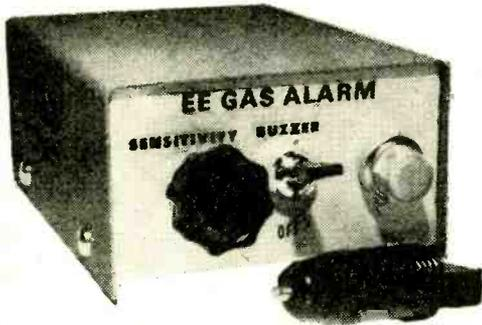
Author's model for portable use. A remote location for both the semiconductor "nose" and Sonalert alarm is an option to consider.
