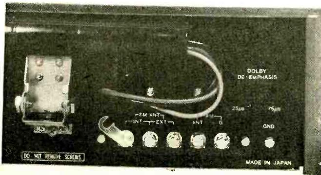
Lafayette's forward thinking engineers made this Dolby equipped FM tuner complete with 25  $\mu$  sec/75  $\mu$  sec de-emphasis switch. Since then, FCC regulations have changed to permit the 25  $\mu$  second de-emphasis characteristic in U.S. FM transmitters. For more information, see next page and circle No. 41 on the Reader Service page.
