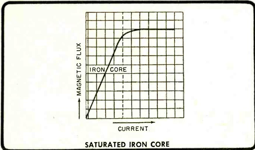
As the current and the flux increase, a point is reached where the curve bends. A further increase in the current produces less and less of a flux increase until, finally, further increase in current produces no additional flux. At this point the core contains as many lines of flux as it can possibly receive; it is said to be *saturated*.
