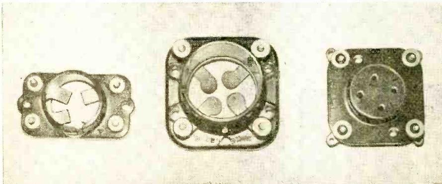
Four-pin tube sockets of very early radio—UV small, UV large, and UX.
