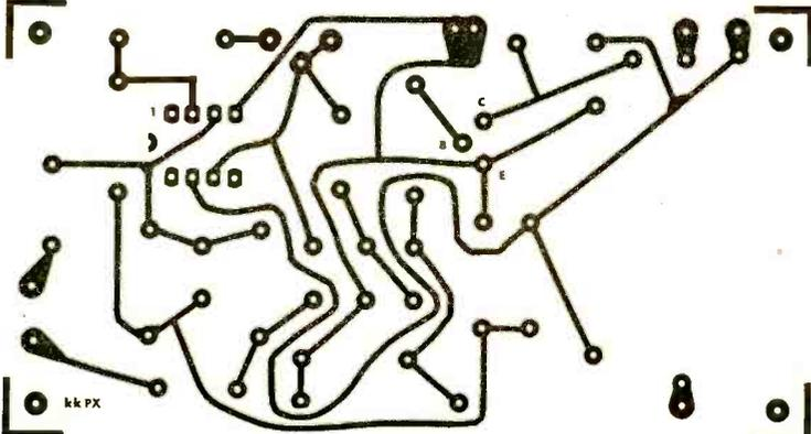
Flip the PC board (shown above) and the copper wiring pattern looks like the drawing at left. In fact, it's an exact size duplicate for those builders inclined to make their own.
