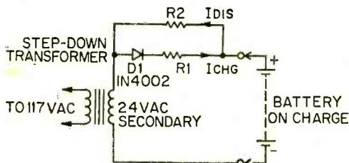
Find all the parts you need for a simple charger like this in a well-equipped junk box. Table below shows R1/R2 values to use.
