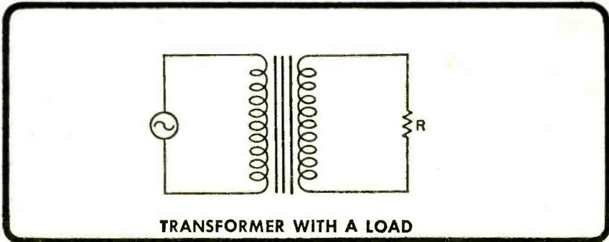
In the example, the current was stepped down in exactly the same proportion as the voltage was stepped up. The power transferred from the primary to the secondary does not change, however, regardless of the turns ratio. This is true providing the rating of the transformer has not been exceeded and assuming 100 percent efficiency.
