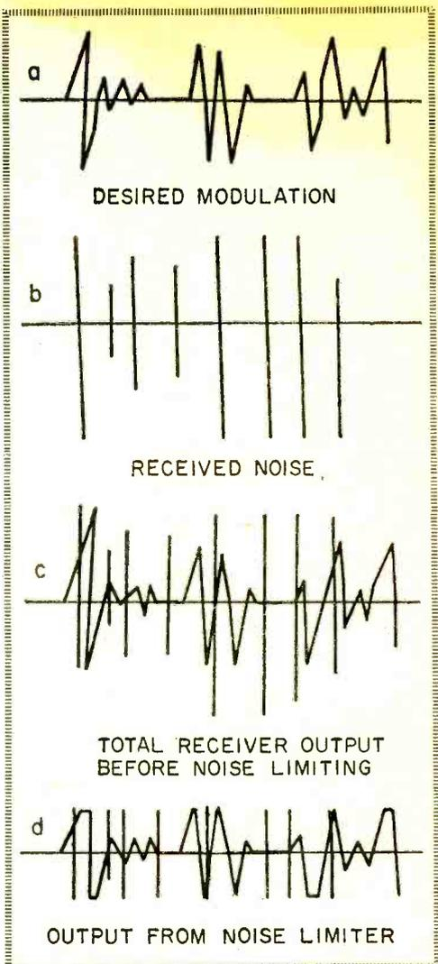
Impulse type noise depicted here in (b) is formed by both man-made sources (auto high voltage ignition) and natural (lightning).
