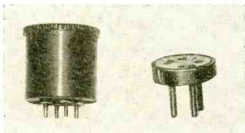
Adaptors such as the one at left allowed a set to operate with tubes at hand (UV small to UV large); on right, UX base tubes can sub for WD-11 type used in Radiola III set.
