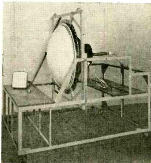
World's largest cathode ray tube (shown with a 10-in. model) will be used by the U.S. Air Force during research for undergraduate pilot training.
