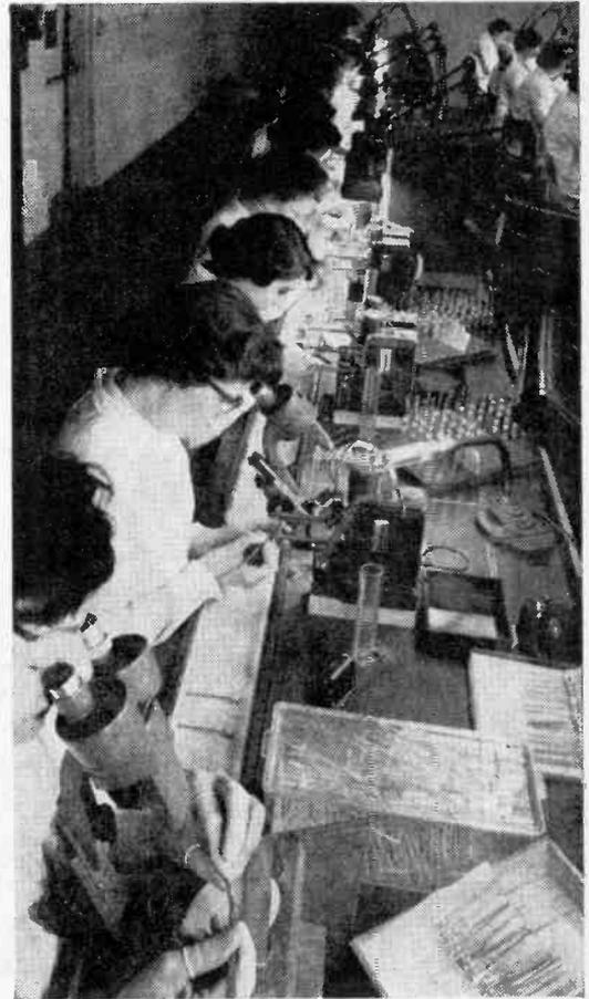
**ASSEMBLING SUBMINIATURE** tubes is done under microscopes. Each operator is equipped with microscope and miniature welder. Note rubber fingers.
