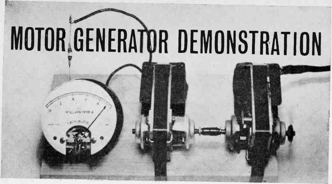
**T**WO old phono motors, salvaged from junked 78-rpm record players, can be used to demonstrate the fundamentals of a motor-generator set. Two motors are strapped to a piece of board, and the shafts are coupled with tape so that one motor drives the other. The captive motor generates a small ac current which is rectified to dc by a germanium diode and then registered on a dc milliammeter.
