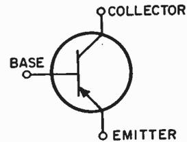
ONE SYMBOL USED FOR THE TRANSISTOR IN SCHEMATIC DIAGRAMS
