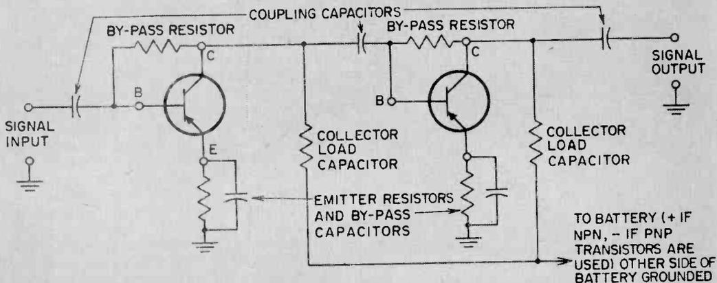
RESISTANCE-COUPLED TWO STAGE TRANSISTOR AMPLIFIER
