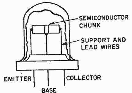
CUTAWAY VIEW OF ONE TYPE OF TRANSISTOR
