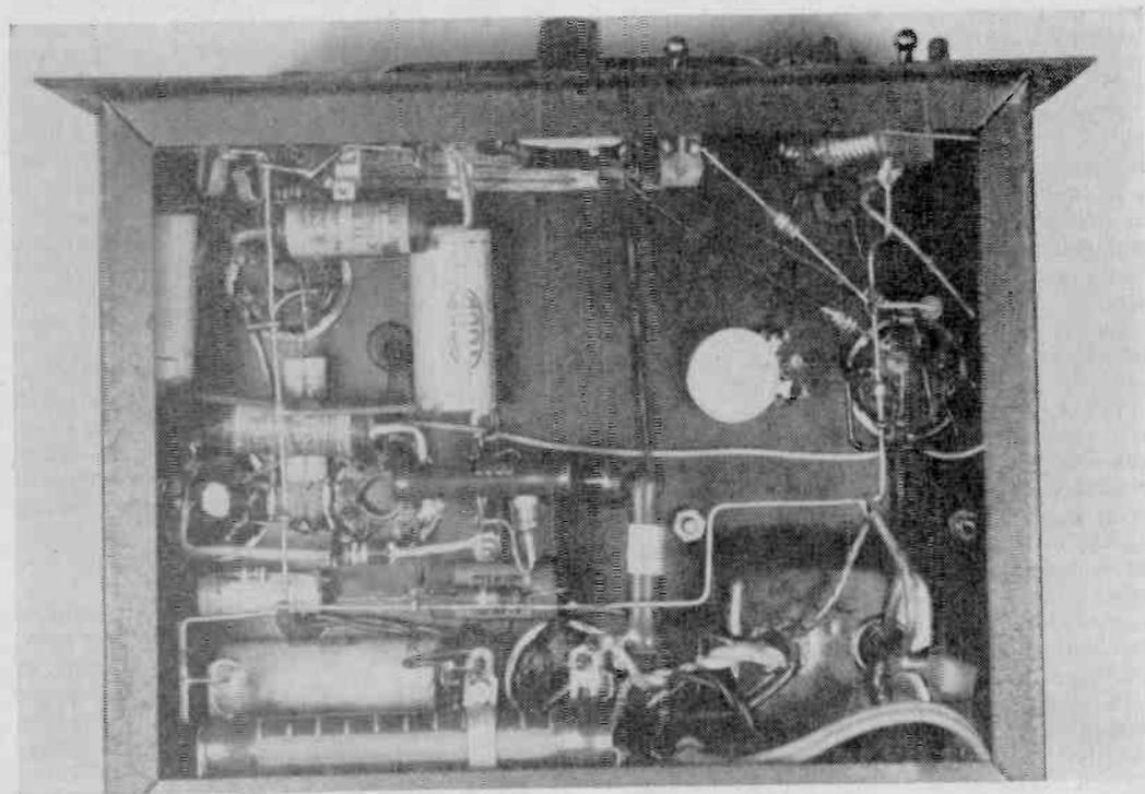
**NEATLY WIRED CHASSIS** may look like a rat's-nest maze to a neophyte, but notice that all wiring is neatly dressed, and squared off. No loose components to flop around here! All filament wires twisted help avoid hum.
