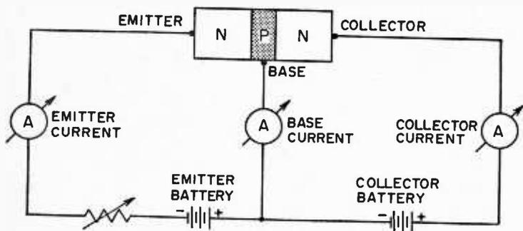
BASIC CIRCUIT FOR NPN JUNCTION TRANSISTOR (FOR PNP UNIT, REVERSE BATTERY POLARITIES)
