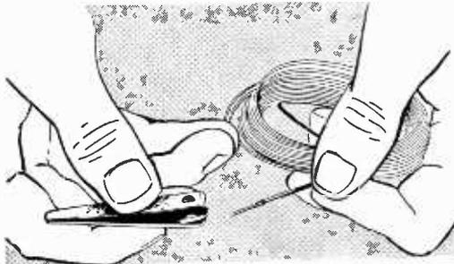
ever, remove the pressure-handle to avoid exerting too much force and cutting right through the wire.—R. J. DeCRISTOFORO.
