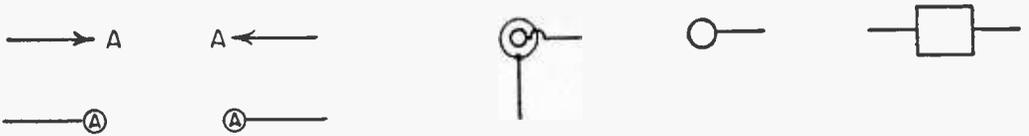
WIRES CONNECTED BY REFERENCE RATHER THAN BY LINES
