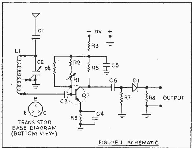
**Our experimental one-transistor tuner picks up short wave broadcasts. With a broadcast coil it is red hot. Parts cost about \$5**
