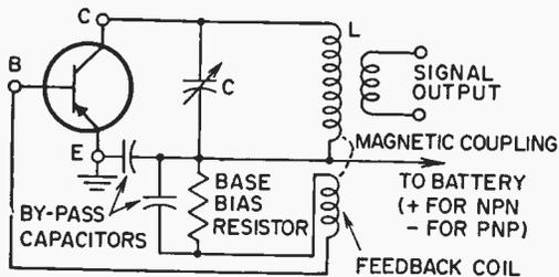
ONE TYPE OF TRANSISTOR OSCILLATOR
