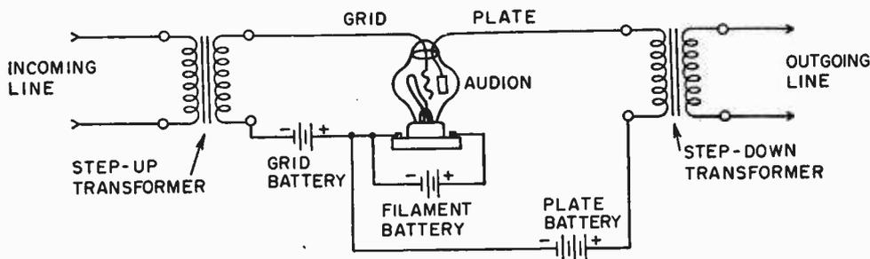
HOW THE AUDION WAS FIRST USED AS A SUCCESSFUL TELEPHONE REPEATER AMPLIFIER
