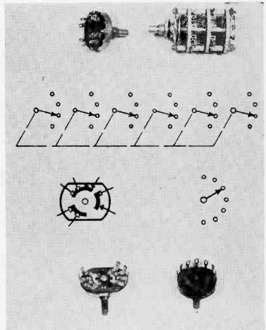
Fig. 9: Various rotary switches are usually shown by breaking out the circuit functions the sections perform.
