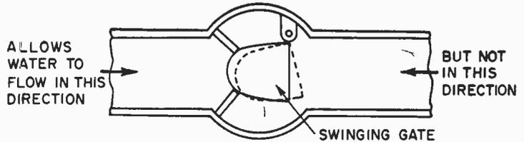
CHECK-VALVE IN WATER LINE
