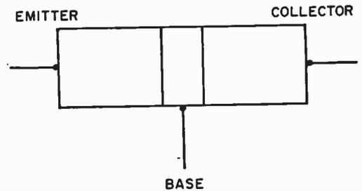
CONNECTING-POINTS, OR "ELEMENTS" OF THE TRANSISTOR. (THESE ARE THE SAME FOR BOTH NPN AND PNP UNITS)
