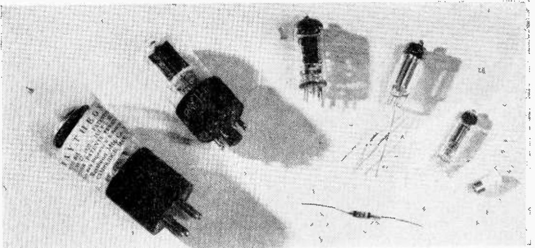
**FAMILY PORTRAIT.** Here is a sum total of 25 years of tube development. At the far left is a BH Rectifier tube, then an octal-base tube followed by a miniature, two sub-miniatures and a germanium diode. At far right is transistor.
