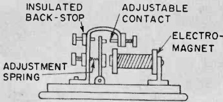
THE TELEGRAPH RELAY ; SUITABLE FOR "AMPLIFYING" ON-OFF SIGNALS, BUT NOT FOR VOICE CURRENTS.
