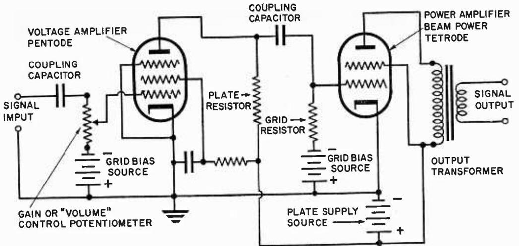
AMPLIFIER CIRCUIT EMPLOYING PENTODE AND BEAM POWER TETRODE
