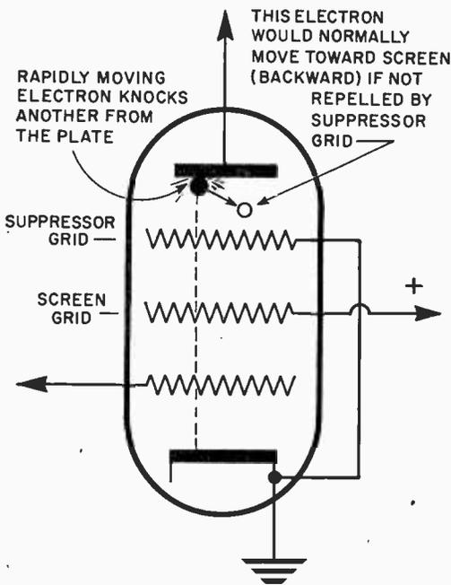
**HOW THE SUPPRESSOR GRID SUPPRESSES REVERSE CURRENT WITHIN THE TUBE**
