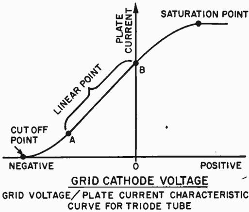
serve that the output voltage waveform, like the plate current waveform, is rather badly distorted. Complex speech or music signals put through such an amplifier would come out sounding like the wrath of heaven through a tin-horn phonograph!
