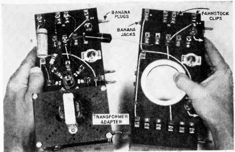
Fig. 8: With one stage complete on the left chassis, a second chassis is plugged in for development of next stage.
