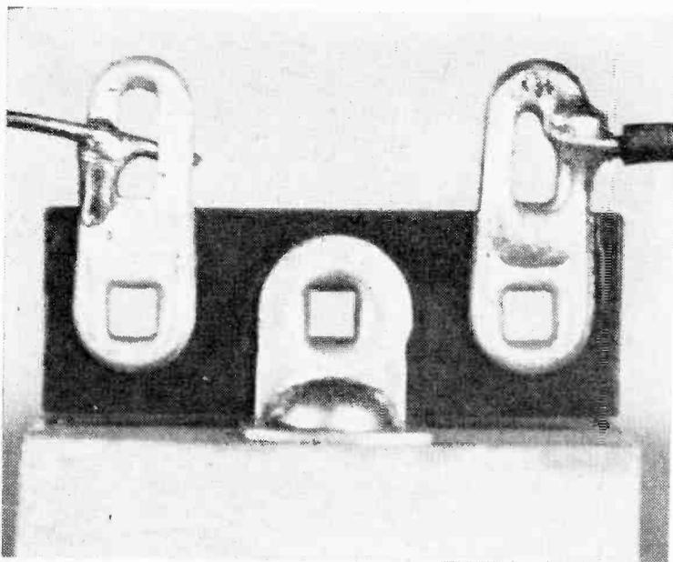
**GOOD AND BAD** soldering techniques illustrated. Wire at left is simply poked through and tacked. Wire at right is first made mechanically sound, soldered.
