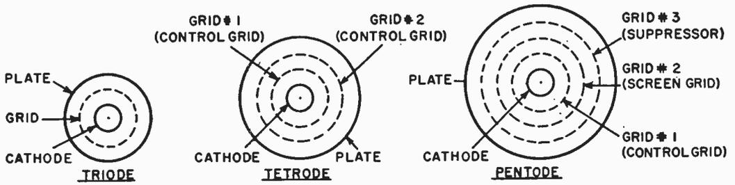
**TOP VIEW OF MULTIELEMENT TUBE ELECTRODES**
