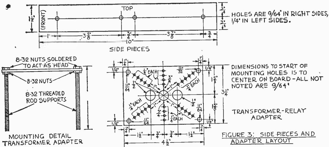
FIGURE 3: SIDE-PIECES AND ADAPTER LAYOUT
