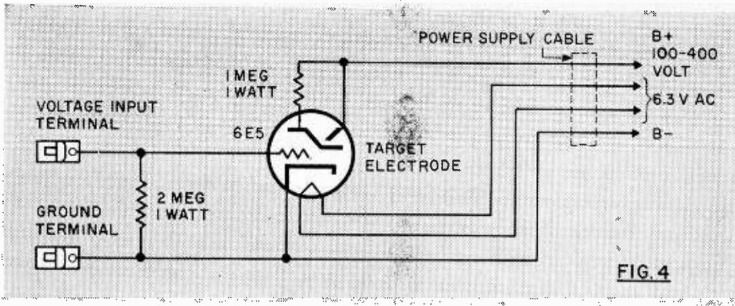
ring to the diagram will show the connections, and it may be used with any amateur transmitter that employs coaxial cable output. The power consumed by this indicator is in the microwatts, and negligible by any ordinary standards, so it does not waste valuable RF watts. It also indicates relative degree of modulation.
