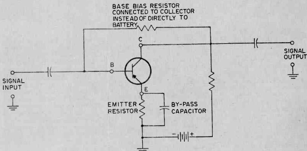
AC AMPLIFIER STAGE DESIGNED TO MINIMIZE "THERMAL RUNAWAY"
