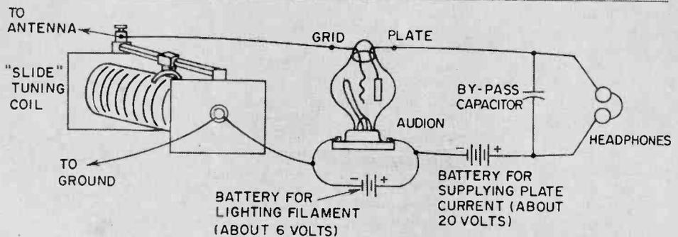
CIRCUIT SUCH AS USED BY DR. DeFOREST IN EARLY AUDION WIRELESS RECEIVER, AROUND 1905
