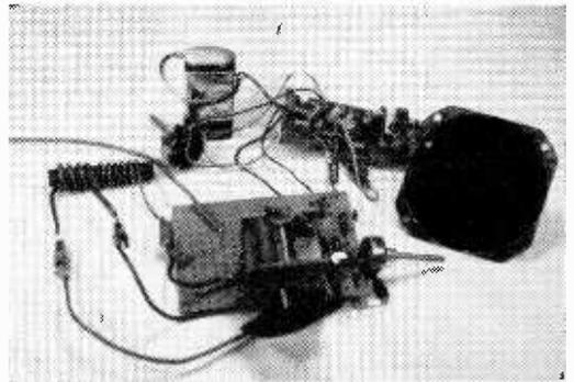
Fig. 5: The finished unit looks unfinished, but is actually shown hooked up with an amplifier and speaker. Battery serves both.
