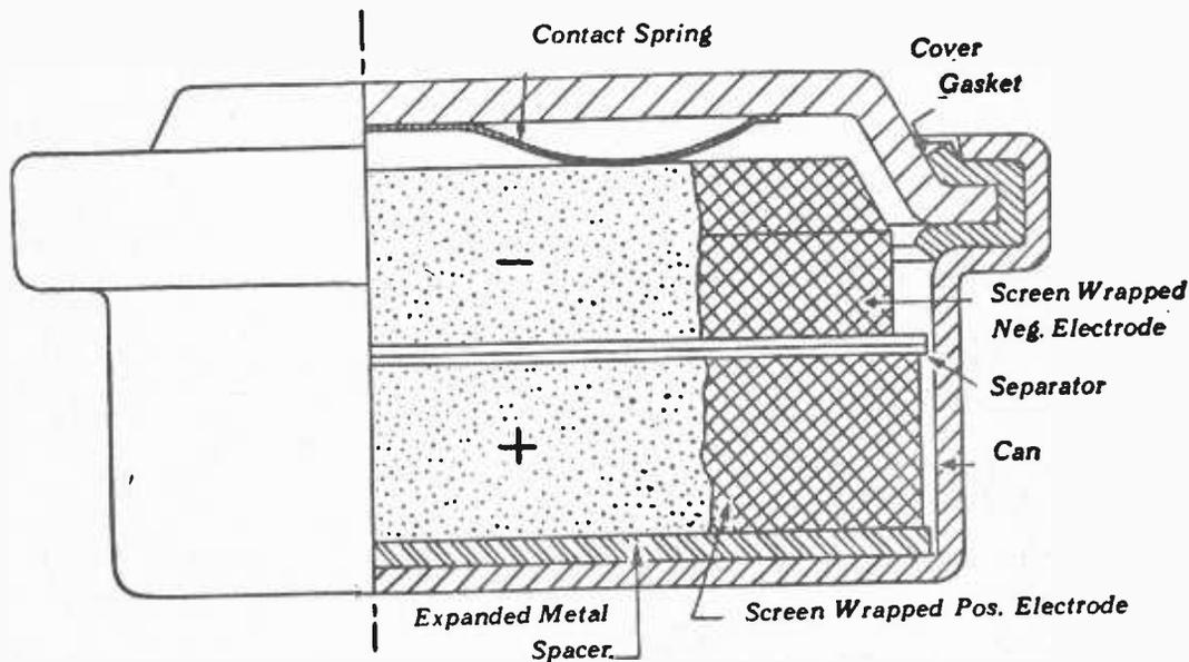
Cutaway of Typical Button Cell
