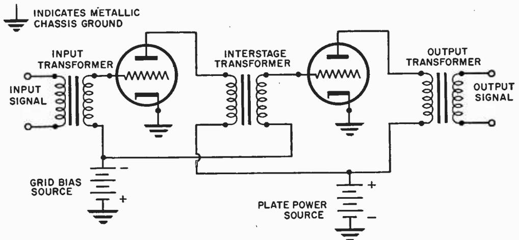
**TWO STAGE TRANSFORMER COUPLED AMPLIFIER**
