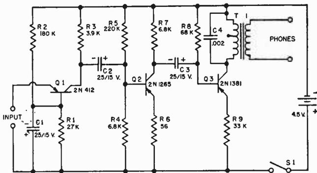
2. SCHEMATIC for transistor amplifier which boosts sound.
