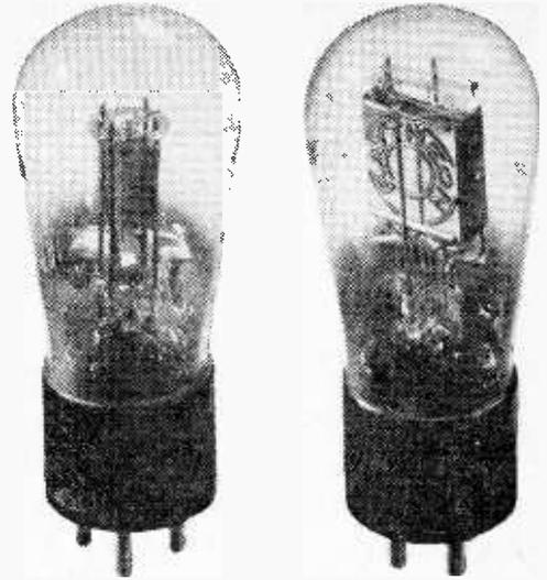
**FAMOUS FIRST** is this Type 27, believed to be the earliest of the indirectly heated cathode types (left) and Type 71, a directly-heated cathode type circa 1926. Note the addition of the base.
