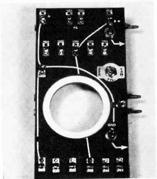
Fig. 10: Basic unit seen from the top with no insert. Lines indicate commonly-connected clips. Note plug and jack positions.
