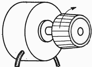
THE RESISTANCE OF THE ORDINARY VARIABLE RESISTOR IS VARIED BY TURNING A KNOB
