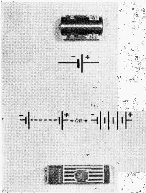
Fig. 12: A battery is a group of cells. Therefore, if you simply draw a group of cells, you have drawn a battery.
