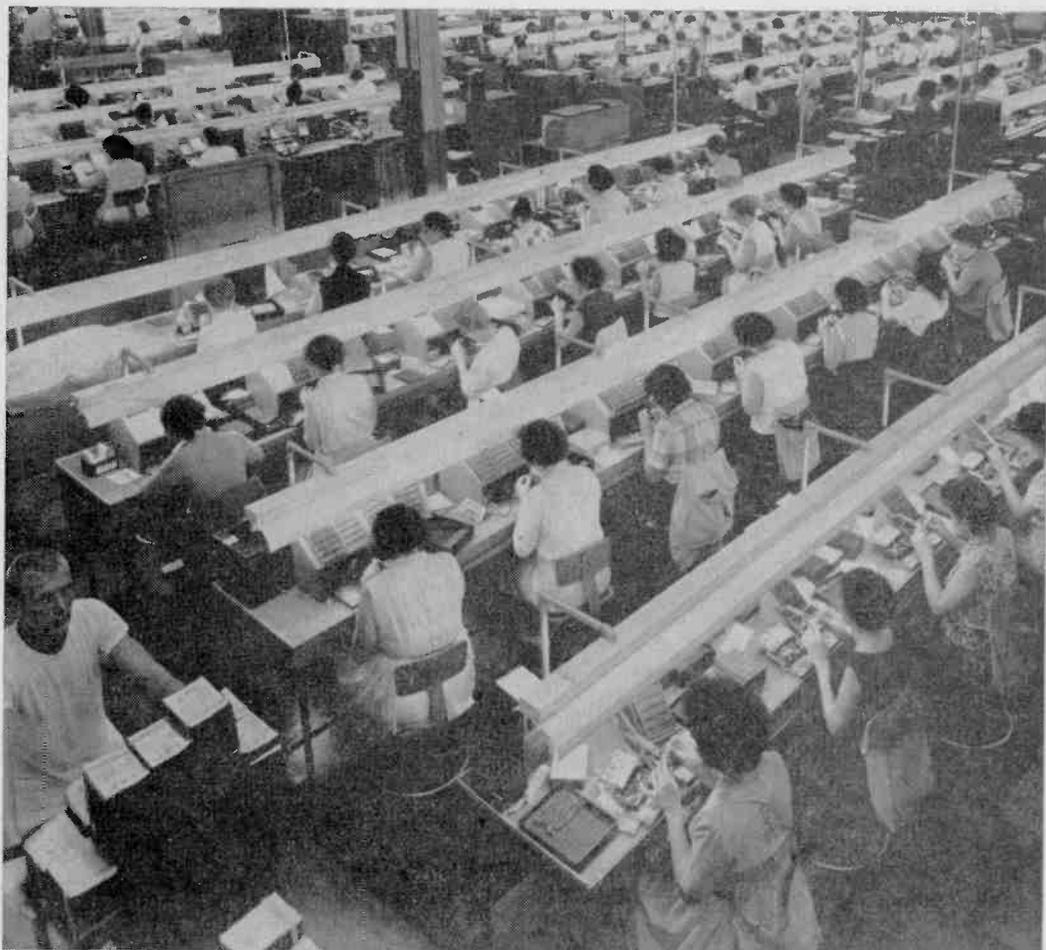
**MINIATURE TUBE PRODUCTION** is carried on in almost sterile conditions. Tubes are assembled from the inside-out, using small tack-welders. After assembly of parts, all metal parts are heat-cleaned, then assembled in glass.
