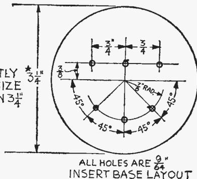
FIGURE 7: POWER TRANSISTOR INSERT
