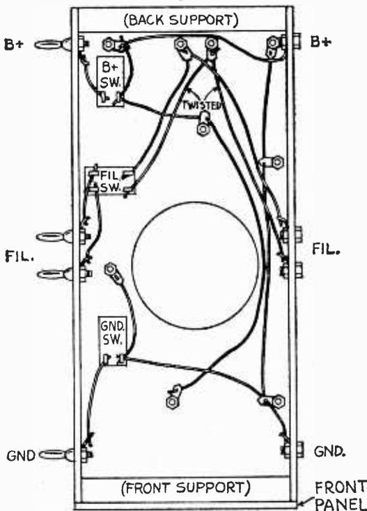
FIGURE 5: PICTORIAL WIRING
