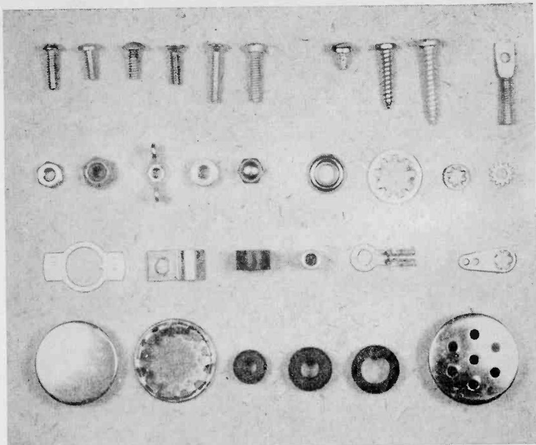
**MORE HARDWARE YOU'LL SEE** includes assorted machine screws (above left), self-tapping or sheet metal screws, spade bolts, various nuts, lockwashers, switch plates, cable clamps, solder lugs, grommets and snap-hole plugs.
