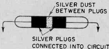
THE COHERER ; WIDELY USED FOR DETECTING WIRELESS SIGNALS AROUND 1900.
