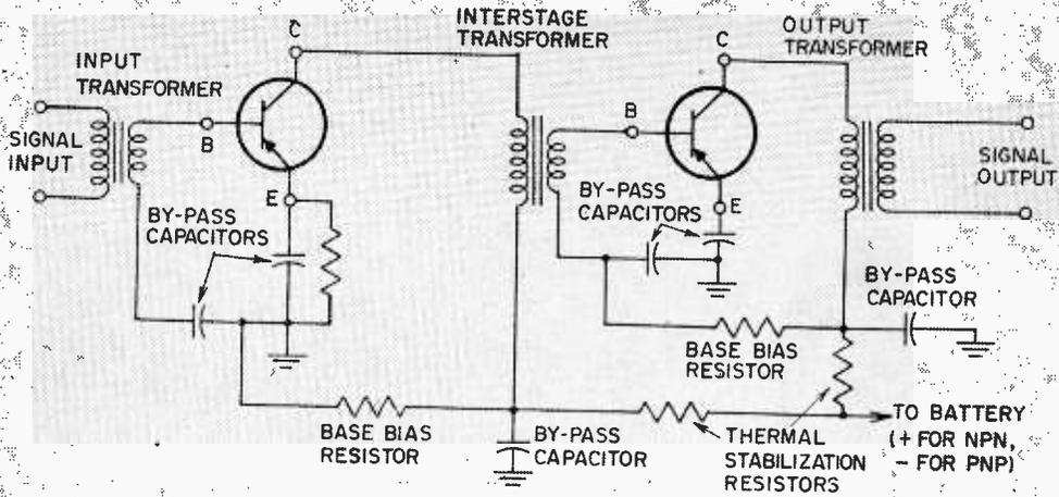
TRANSFORMER-COUPLED TWO STAGE TRANSISTOR AMPLIFIER,
