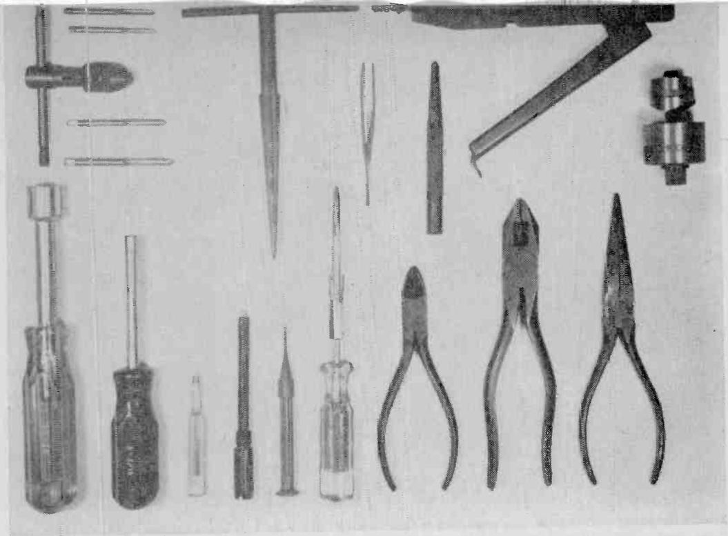
**METAL-WORKING TOOLS** for electronics include an assortment of taps and a tap-handle, a reamer, tweezers, center punch, hand nibbler, chassis punches, nut-drivers, screwdrivers, wire cutters and pliers. Have tools on hand.
