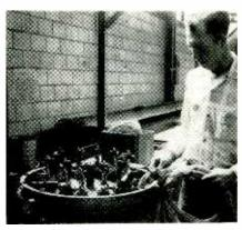
STEP 11-Pressurizing test barrel used for testing feed-through bushings at pressures up to 15 psi
