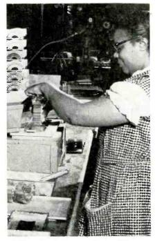
STEP 5—Tinning terminals in solder pot
