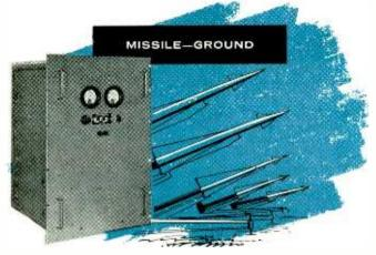
Perkin has developed Magnetic Amplifier Regulated DC Power Supplies for missile launching and check-out, with ratings of 30, 50, 100, 200, 300, 400, 500 amperes and above. The unit shown here is a 24-32V, DC @ 100 amp. unit, 19" rack panel mount, with a regulation of  $\pm \frac{1}{3}$ % over the range of 24-32 volts. There are provisions for remote operation and sensing. Perkin ground power supplies are now being used in the Thor, Atlas, Bomarc, Vanguard and other missile programs.
