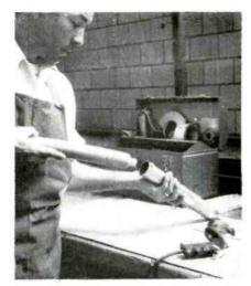
STEP 6—Loading filled plastic liner in potting gun
