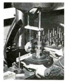
Pointer of indicator, at center line on scale, indicates that stack is at desired height. Pointer is actuated by downward projection bolted to ram of press. Fcr safety, operator must press down two valves as shown when operating press
