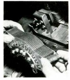
STEP 1—Loading position of slide, with operator preparing to insert assembled contact bank. Spacer comb is being placed between decks of switch with right hand
