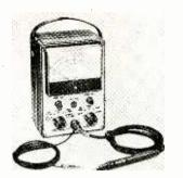
JUNIOR VoltOhmyst® WV-77C — Biggest value in vacuum-tube volt-ohmmeters! Factory tested and calibrated to lab standards. Measures dc from 100 millivolts to 1200 volts; ac from 100 millivolts to 1200 volts rms; resistance from 0.2 ohm to 1,000 mcgohms. User Price \$59.50\*
