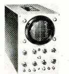
5" OSCILLOSCOPE WO-91A—Dual Band 4.5 Mc scope, for waveshape observation and measurement, signal tracing and alignment of chrominance circuits and wide-band amplifiers—voltage-calibrated input step-attenuators and calibrated graph screen make possible direct voltage readings as easily as with a VTVM. User Price \$239.50\* \*User Price (Optional)
