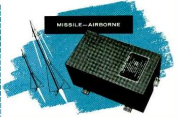
Perkin airborne power supplies more than meet both military specifica-tions MIL-E-5272A and MIL-C-7115. The use of silicon rectifiers pro-vide a much more compact package with higher efficiency ratings and longer life expectancy. The unit illustrated provides 27.5 volts DC (26 to 30 volt range), 20 amperes continuous duty. The input is 115/200V AC, 3 phase; frequency range 400 CPS  $\pm 6$  CPS. The regu-lation is less than  $\pm 0.5$  volts.
