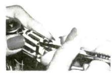
Packing second coil into stator slot
