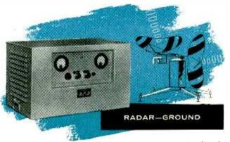
Hundreds of Perkin Ground Radar Systems are in operation through-out the country. Built to specifications MIL-E-4158, this unit was con-servatively designed and will operate at 150% load continuously without damage to the unit. Specifications are: AC Input-120/208V  $\pm 10\%$ , 3 phase, 60 cycle  $\pm 2$  CPS, 4 wire system; DC Output-24-32V @ 100 amps; Regulation  $-\pm \frac{1}{2}\%$  (for any combination of line and load changes); Ripple-1% RMS or less.
