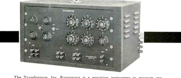
The Transformers, Inc. Ratiometer is a precision instrument to measure any voltage ratio from 0.000001 to 1.111111. Transformer ratios can be accurately measured at "no load" and under full load. Two models are available:
