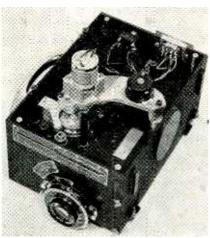
Gearcase for the recording camera
