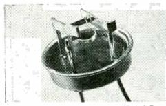
View of uncapped G-E silicon NPN diffusedmeltback transistor, showing mounted silicon bar with aluminum base lead connected. Bar ends attached using a gold-alloy mounting technique. No solders or fluxes are used.
