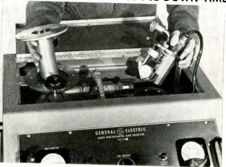
**DOWN-TIME IS REDUCED** through easy access and removal of the spectrometer tube (right) and by a simplified vacuum system design.
