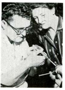
Lloyd Larsen demonstrates how automatic file is used for removing welding flash inside complicated waveguide section
