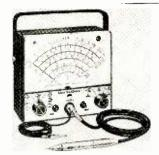
SENIOR VoltOhmyst<sup>®</sup> WV-98A — Improved circuit provides greater accuracy, 3% on BOTH ac and dc measurements. Measures directly the peak-to-peak values of complex wave forms and rms values of sine waves. *LARGE* full-vision meter, with less than 1% tracking error, provides one of the easiest reading VTVM scales. User Price **\$79.50**\*
