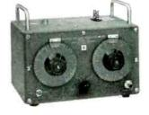
Impedance Meter, Line Fault Analyzer Sierra 166 Impedance Meter (at left) measures impedance on high noise circuits, 30 kc to 300 kc; measures on "hot" lines through coupling capacitor. Sierra 124 Line Fault Analyzer pinpoints shorts, opens or grounds on open wire lines. Direct reading, range  $\frac{1}{2}$  to 200 miles, accuracy  $\frac{1}{4}$  mile.
