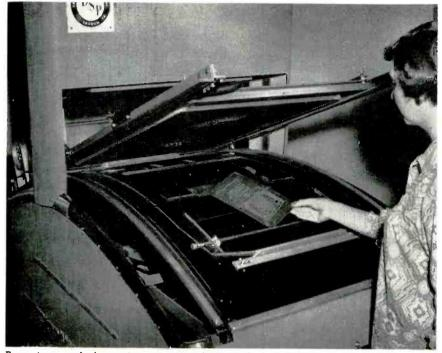
Removing panel after resist pattern has been applied, to complete printing cycle
