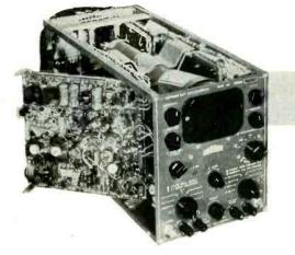
Bondwidth—0-4 Mc. Sensitivity (amp)—0.2 volts peak/major division Input Impedance—2 megohms, 30 uuf (max.)
