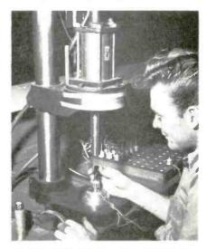
Placing guide thimble over stator in fixture on air-actuated arbor press
