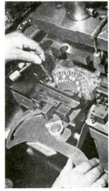
STEF 2—With bank assembly in position on slide, operator inserts positioning pin. Right hand is on lever which will later be pulled to move slide under press
