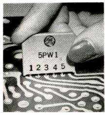
Manual placement in plated wiring board. Molded projections on phenolic housing keep unit above board so solder can form fillets around leads on top of board
