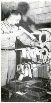
STEP 7—Filling cannector by using airoperated potting gan
