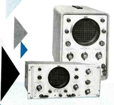
Low Frequency Cabinet Oscilloscope, Model 130A. Covers dc to 300 KC. Similar horizontal and vertical amplifiers. Input circuits balanced on 5 most sensitive ranges. Single ended input may be dc or ac coupled. Direct reading, linear sweep times. With most transducers, needs no preamplification to produce brilliant, high resolution trace. Universal automatic triggering; one preset condition provides optimum triggering for almost all inputs. \$650.00.
