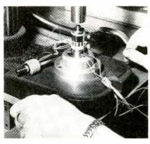
Operator has placed yoke rings in position on thimble and is preparing to operate press controls with both hands to push rings down against those already on stator. Complete stator with yoke rings can be seen on bed of press
