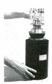
**TRIODE MODULATOR** for instrumentation radar
