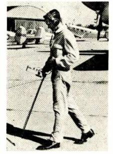
Operator traces underground cable at airport installation and pin-points cable fault. The detecting-element coil is mounted on the telescoping boom connected to the amplifier-indicator case. Signal strength is indicated on an output meter and headset monitors the output
