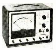
**MASTER VoltOhmyst**<sup>®</sup> **WV-87B**—Ideal for TV, radar and other types of pulse work. Has accuracy and stability necessary for laboratory applications. Features  $\pm 1\%$  multiplier and shunt resistors; a  $\pm 2\%$  meter movement; DC polarity reversing switch; zcro-center scale adjustment for discriminator alignment;  $\pm 3\%$  accuracy on AC and DC voltages, many other features. User Price **\$137.50**\*
