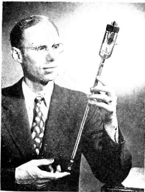
megacycles is typical of the device. The tube is a foot long and a few inches in diameter. Its amplifying property results from the transfer of energy from an electron stream to a wave moving on a helix surrounding the stream.
