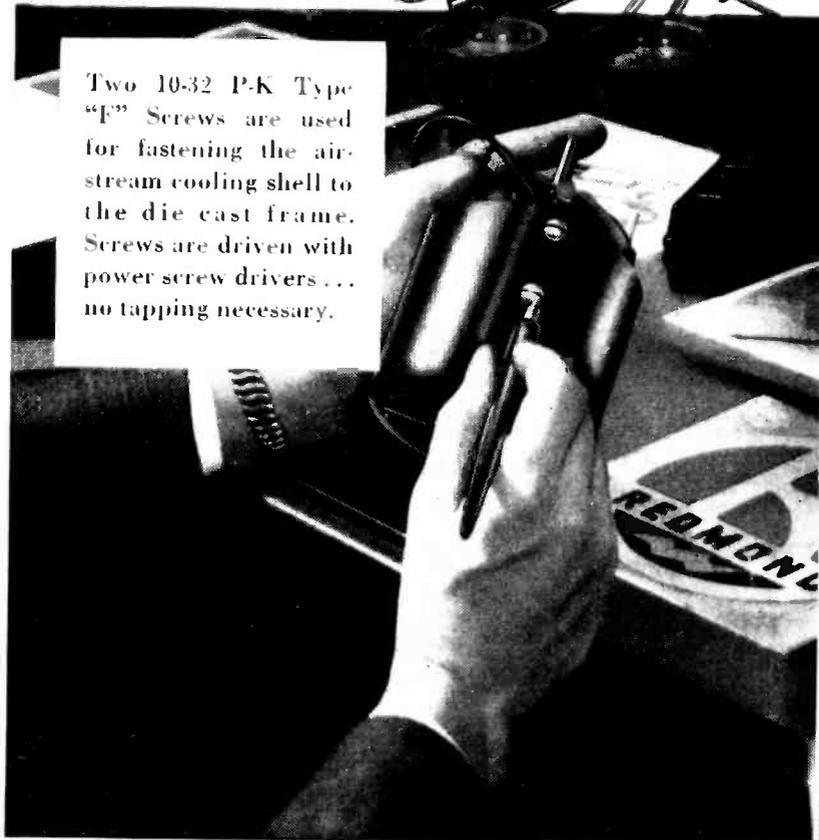
Two 10-32 P-K Type "F" Screws are used for fastening the air-stream cooling shell to the die cast frame. Screws are driven with power screw drivers ... no tapping necessary.
