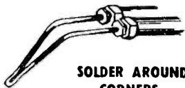
Service and maintenance men can save time by the fast heating of the Soldering Gun. By use of the new induction principle, 5 second soldering heat is supplied from a light weight built-in transformer.
