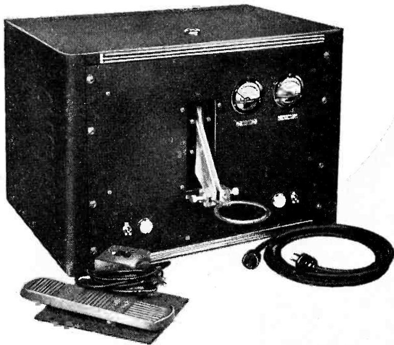
A low-cost, low-powered induction soldering unit, designed for use wherever production soldering of small metal parts and assemblies is part of the job. It increases the quality of soldering operations . . . minimizes time and expense involved . . . requires no experienced help . . . and can effect major production economies in such diverse fields as radio, electronics, jewelry, electrical fixtures, toys, kitchenware, motors, paint brush ferrules, can sealing, etc.
