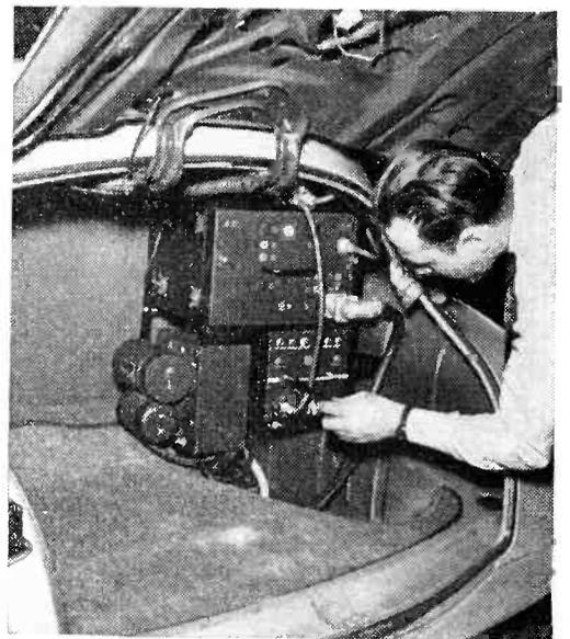
In the baggage trunk of the cab are mounted the 40-watt f-m transmitter at top, receiver at lower right, and dynamotors at lower left
