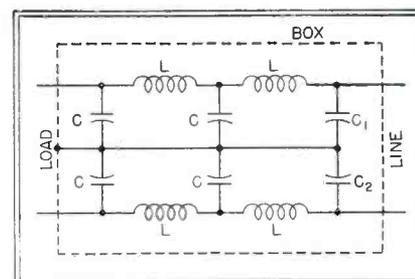
Capacitors  $C_1$  and  $C_2$  were not always necessary in the filter. All capacitor values were  $0.1 \mu\text{f}$  but lower values were sometimes satisfactory. The inductors marked  $L$  consisted of 20 turns wound on a one-inch diameter form
