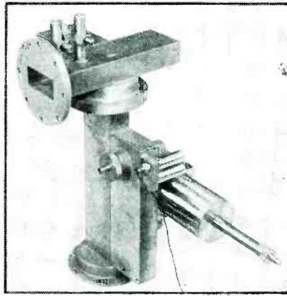
This wave-guide structure comprises a directional coupler, barretter mount, cavity wavemeter, magic tee, crystal mount, and tuning screws for impedance matching
