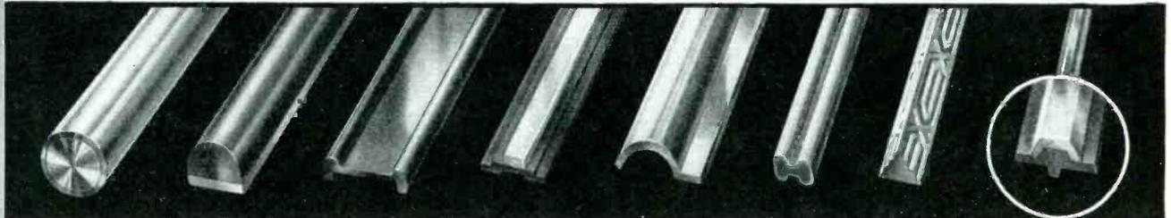
**WIRE:** We draw wire to diameters as fine as .005" to .006" depending on the material, and the precious metal thickness can be held to a tolerance of .0001". In spite of such small dimensions, such wires are often engraved for decorative purposes or shaped for industrial use. Laminated wires, available in every conceivable shape, are widely used
