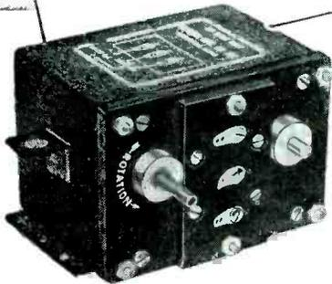
Remote control differential drive for airborne radar computer unit.
