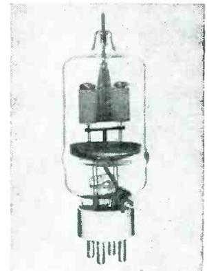
typical voltages include d-c plate voltage, 3,000; d-c plate current, 250 milliamperes; plate power output, 600 watts with an approximate driving power of 27 watts. The filament operates on 5 or 10 volts at currents of 12.5 or 6.25 amperes. Overall length of the tube is 7.625 in.; diameter, 2.563 in. Net weight 7 oz.
