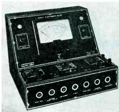
as voltmeter and ammeter. It has the following ranges: 6-30,000 a-c ma; 6-30,000 d-c ma; 3-6,000 v a-c; 6-6,000 v d-c; 0-1,000 megohms.
