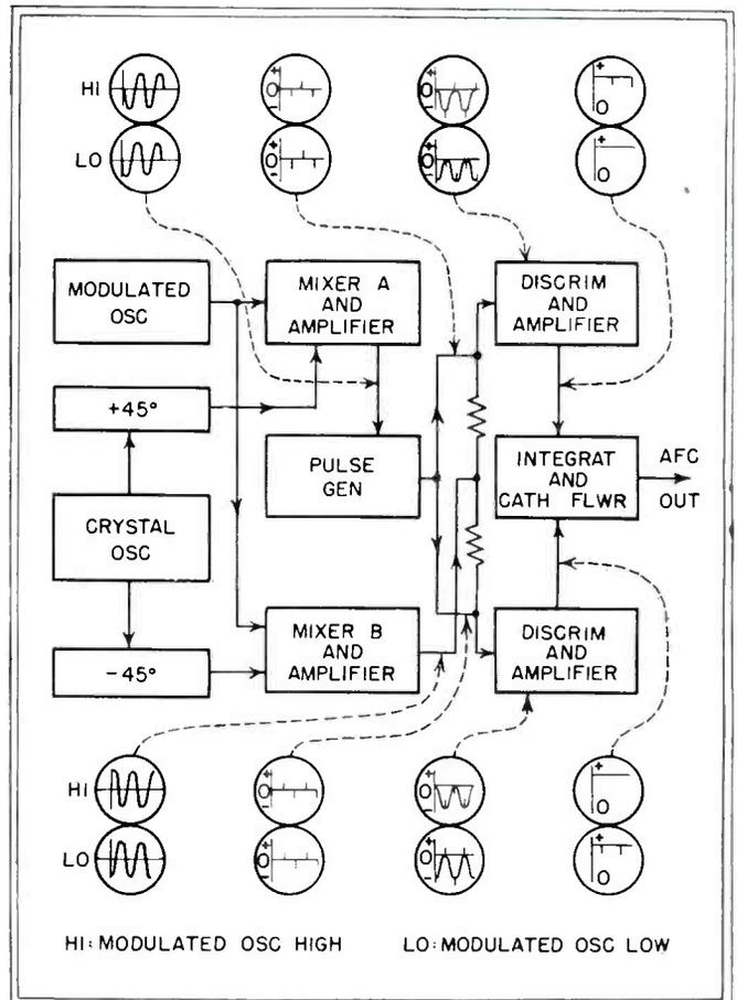
FIG. 2—Pulse counter stabilizes f.m. oscillator
