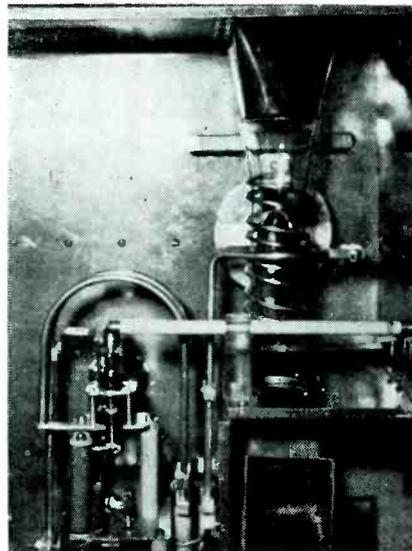
Tank circuit assembly of the Aircon r-f heating generator for a slot machine. A cellophane-wrapped frankfurter and roll slides down the chute to the coil where it is electrically heated in 20 seconds and then delivered to the customer for ten cents
