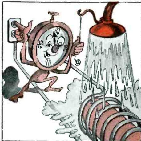
**3** **CONTROLLED QUENCHING** is secret of uniform hardening! With Allis-Chalmers Induction Heater, water quench can be *direct connected* to Timer. Quenching operation and heat sequence are *identical* each time. This feature, plus design of work coil, completely controls hardness and depth of penetration within very close limits.
