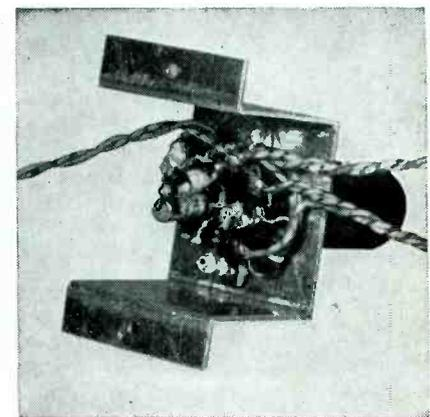
Laboratory model of the simple 100-mc converter made by Electronics Research, Inc. of Evansville, Indiana
