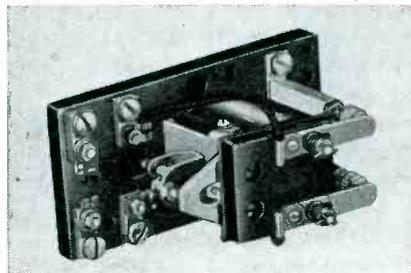
6 to 230 volts, and the a-c types, on 6 to 440 volts. Contacts will carry 25 amperes d-c up to 24 volts, or one ampere at 230 volts. In operation on 60 cycle a-c circuits, contacts will carry 25 amperes up to 250 volts or 50 amperes up to 440 volts. All relays employ silver-to-silver contacts.
