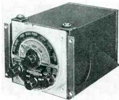
PAR-70A requires 2.5 amperes at 12 volts. The -70B type equipment requires 1.25 amperes at 24 volts. Overall size is  $4\frac{7}{8}$  x  $5\frac{7}{8}$  x 7 inches. The weight is 5 pounds, including a vibrator power supply. The loop antenna is 11 inches high, 9 inches in diameter and weighs 1.4 pounds including azimuth indicator and 6-foot transmission line.
