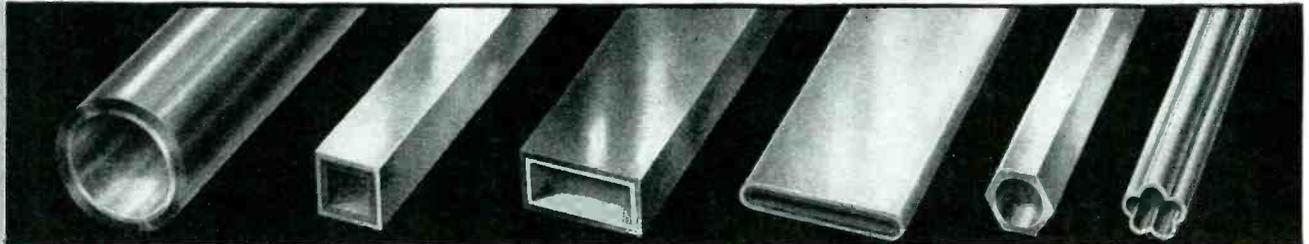
**TUBING:** Because our tubing is actually deep-drawn sheet, its quality is easily controlled. Dimensional limits lie between approximately .015" O.D. to 2" O.D. with wall thickness as small as .005". Very close tolerances can be maintained both on wall thickness and diameters. Laminated tubing is now used in the electrical industry, for electronic applications, high frequency radio parts, delicate instrument
