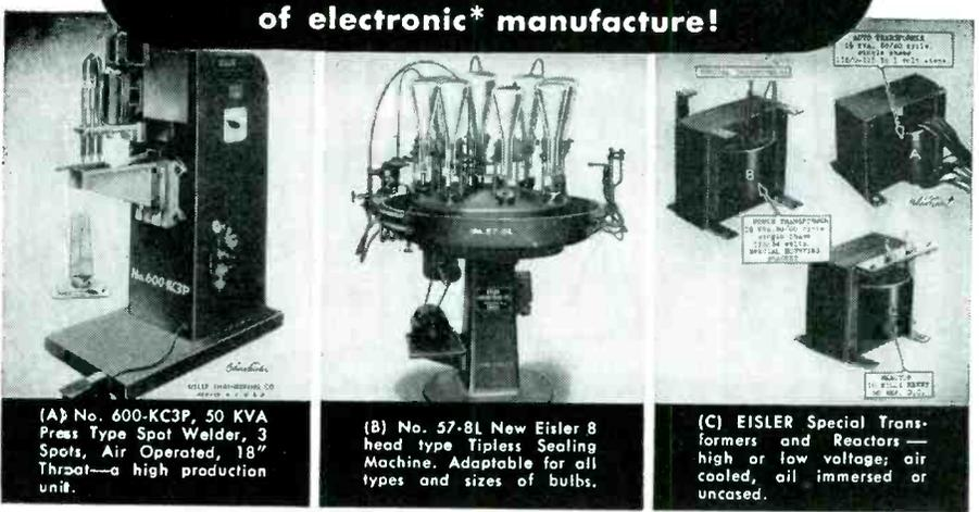
(A) No. 600-KC3P, 50 KVA Press Type Spot Welder, 3 Spots, Air Operated, 18" Throat—a high production unit.
