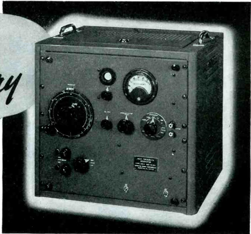
This instrument has found universal acceptance because of its wide frequency coverage from 20 cycles to 5 megacycles. A five step decade attenuator provides a means by which extremely small output voltages can be accurately set and a six position switch enables any one of a variety of output impedances to be quickly selected.
