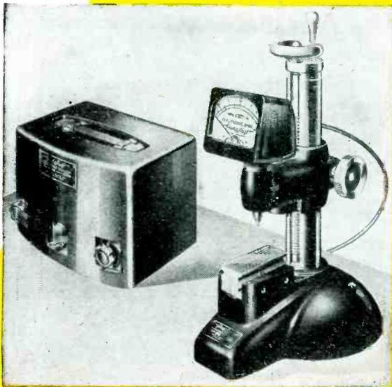
**J & H Electronic Gages.** Such as the widely used comparator that measures to millionths of an inch.
