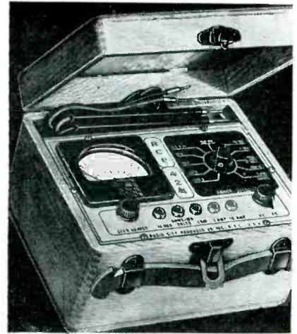
ohms. It can also be read directly as a decibel meter across a 500-ohm line. The instrument measures  $7\frac{1}{2} \times 5\frac{1}{4} \times 3\frac{1}{4}$  inches and weighs 2 pounds. A portable type, Model 424P, is somewhat larger and heavier. Both models have self-contained batteries.
