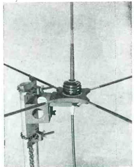
cut to a specified frequency in the range 28 to 152 megacycles. Complete with 50 feet of RG 8/U solid dielectric cable it sells for \$33.50, f.o.b. The Type 703 50-foot cable extension complete with connectors is priced at \$12.75.
