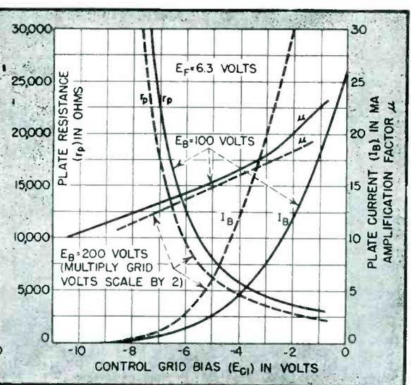
FIG. 3—Transfer characteristics
