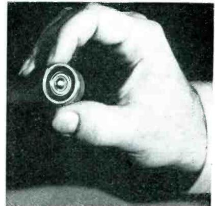
charge characteristic. No rest periods are required owing to a new method of minimizing polarization effects. Within rated limits each cell has an ampere-hour capacity independent of drain. Each cell measures 1 inch in diameter and is  $\frac{3}{8}$  inch high. The cell case does not corrode, being made of steel, nor does it take part in the electrolytic action of the
