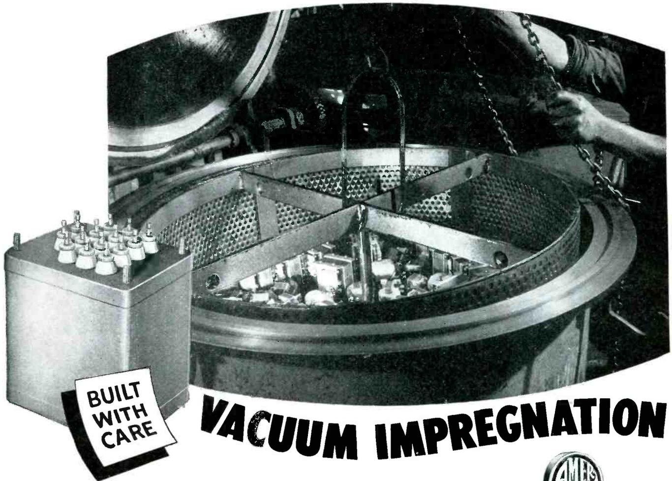
Vacuum impregnation helps to stabilize the performance characteristics of AmerTran-Transformers. Each unit is subjected to both heat and a vacuum process to withdraw all moisture. While still in the vacuum chamber, the compound is introduced and forced into every interstice and around all surfaces of the windings.
