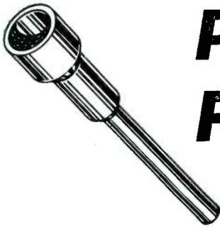
Counterbored head, drilled secondary hole to 1/3 of way down through shank.
