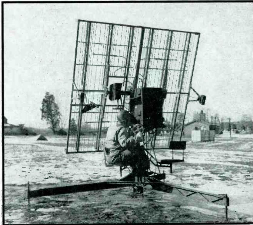
Radio set SCR-658, used for radiosonde tracking to determine wind speed and direction
