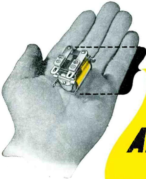
The "CR" relay illustrated is a single pole normally open double break arrangement. Standard insulation is molded bakelite. Contacts are silver, although alloy contacts can be supplied. Contact rating with  $\frac{1}{4}$ " silver is 15 amperes at 24 volts D. C. or 110 volts A. C. Non-inductive. The arrangement shown is  $1\frac{33}{64}$ " high;  $1\frac{3}{32}$ " wide and  $1\frac{25}{32}$ " long. Weight 3 ounces.
