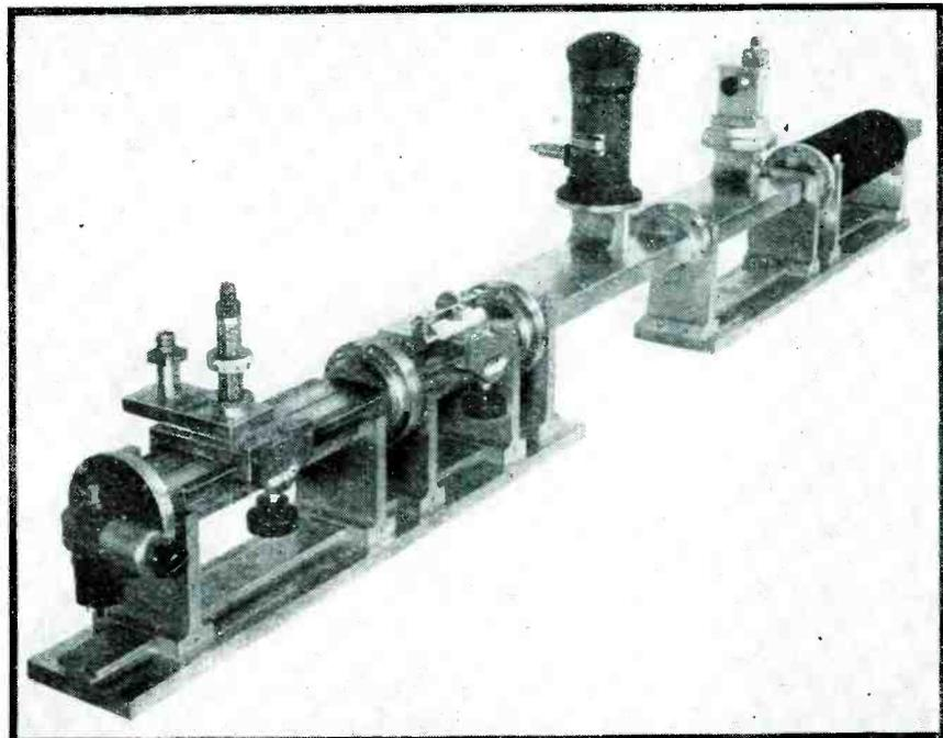
An assembly of wave-guide measuring instruments used to determine the effect of load impedance upon oscillator power and frequency. From left to right are: a reflex klystron, impedance meter, impedance transformer, directional coupler (with a cavity wavemeter this measures frequency) barretter mount for power measurement, and high-power matched load. All the rectangular guide shown is  $2 \times 1$  inch.
