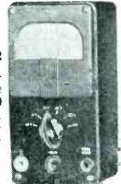
The output meter, 0-1.5-6-15-60-150 V. AC, all ranges have a constant impedance of 4000 ohms, therefore ranges can be switched without changing load on circuit. A built-in condenser is also provided to block D.C. when checking output right at the plate terminals. This instrument is very useful when using a signal generator to align a set.
