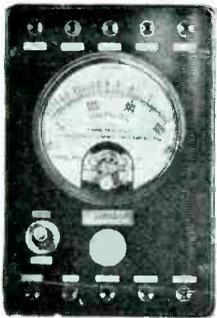
**685-2 Tube Checker**, check many tubes but not above a 25 volt filament comes complete with Loktal and Octal adapters. It can easily be converted by adding a new transformer for the higher filament voltages. Without conversion it will check over 250 standard radio tubes.
