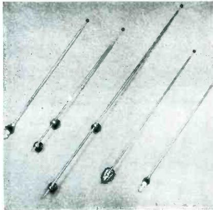
provided with silver contacts to a shielded transmission line which prevents electrical interference. Of the several types available, all telescope into a moderate length.
