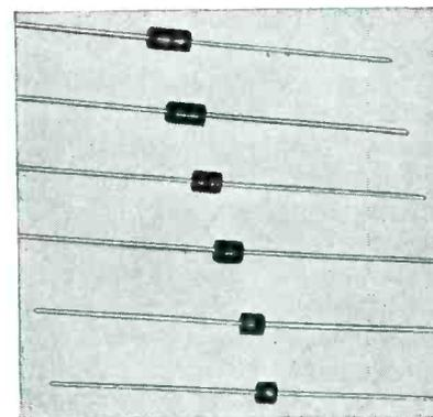
they eliminate the undesirable inductive characteristics common to twisted wires. Standard capacitance values include 0.68 to 4.7 micromicrofarads. The standard tolerance is plus or minus 20 percent.
