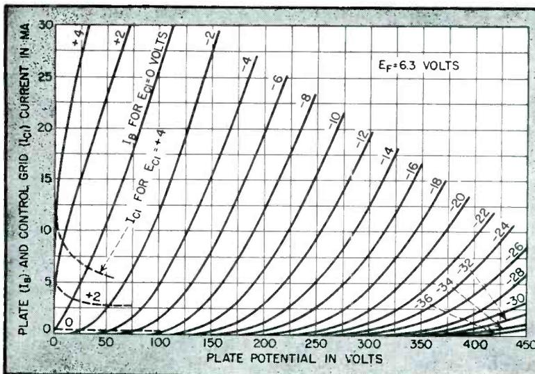
FIG. 2—Plate characteristics
