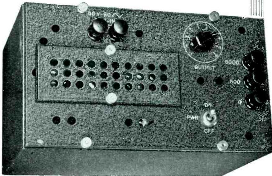
The Type MR-1000 is a compact source of audio frequency power producing up to 35 MW of signal energy at output impedances of 500 or 5000 ohms.
