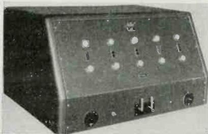
The unit has an electronic visual gauge which can be used as an inspection tool to safeguard against faulty components; or it may be used as an automatic filter to grade components for their individual tolerance. The unit checks a-c resistance and impedance, capacitance and inductance. Tests are made automatically. Instead of meter readings, rejects are indicated visually and audibly.
