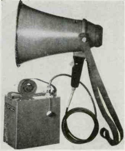
combination microphone and loud-speaker equipped with a pistol grip, squeeze-to-talk, switch and a strap permitting the unit to be suspended from the neck or shoulder of the user; and a battery-powered amplifier which is also equipped with a carrying strap. Both units are connected by a 6-ft. heavy-duty electric cord. The amplifier weighs 8 lb and 2 oz and measures 7½ x 7½ x 4½ in. The megaphone weighs 6 lb and 12 oz and measures 13½ x 10½ in. Units are splashproof and shockproof.
