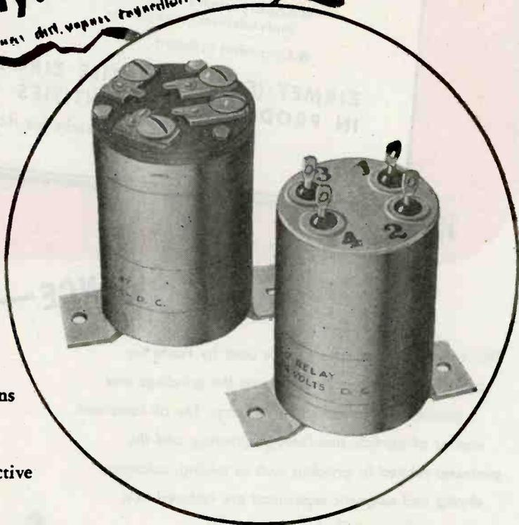
Unit has withstood Army test, including overload; vibration 55 cycles per second with .06' excursion; acceleration of 10 gravity units; salt spray tests of 240 hours duration.
