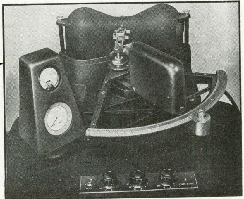
Focusing spectrometer engineered by North American Philips Co. The counting meter scale at the lower left indicates radiation intensities directly as the Geiger tube is rotated from one end to the other of the graduated quadrant that shows diffraction angles. The x-ray tube is in the dumbbell-shaped housing at the rear
