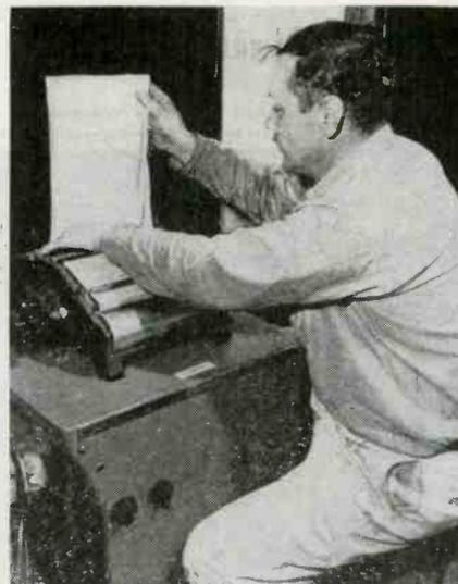
The conductor of a Rock Island freight train removes a facsimile message sent to him by radio from a wayside station. A complete message form is turned out in three minutes
