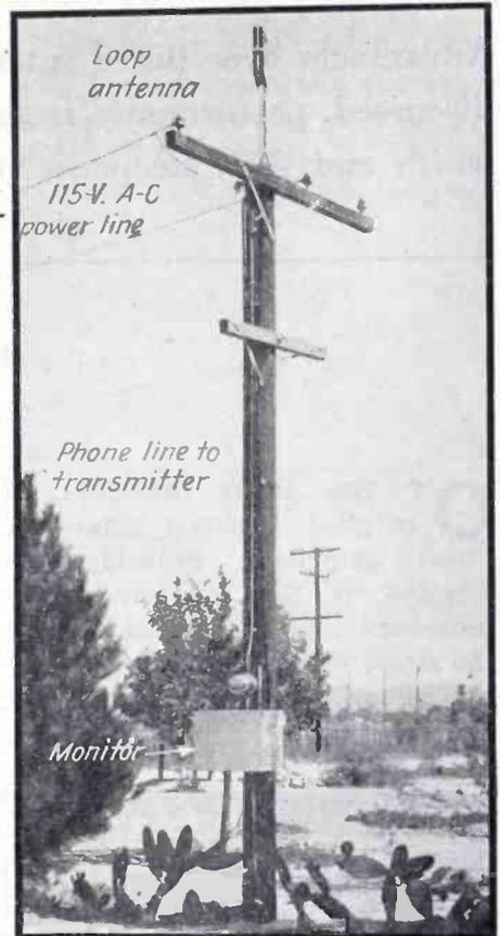
Mounted on a pole, the remote monitoring unit receives a signal from the antenna array to the right of the pole in the background and 1½ miles away. Receiver diode current goes back to the transmitter by phone line
