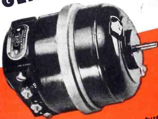
We were called upon to manufacture this small voltage generator in which concentricity between shaft and mounting ring had to be within .001" while diameter of large mounting ring was held to  $\pm .001$ ". Output voltage was linear with speed to 1% and voltages were equal within 1% for each direction of rotation. A careful analysis of tooling requirements, together with the use of precision equipment, did the job.
