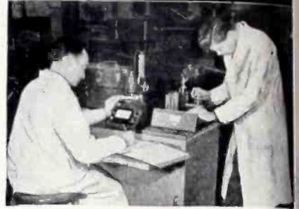
A complete inspection department on wheels, to check parts right at the machine or bench. Errors are caught where they start and hundreds of dollars in wasted materials and hours and material are saved.
