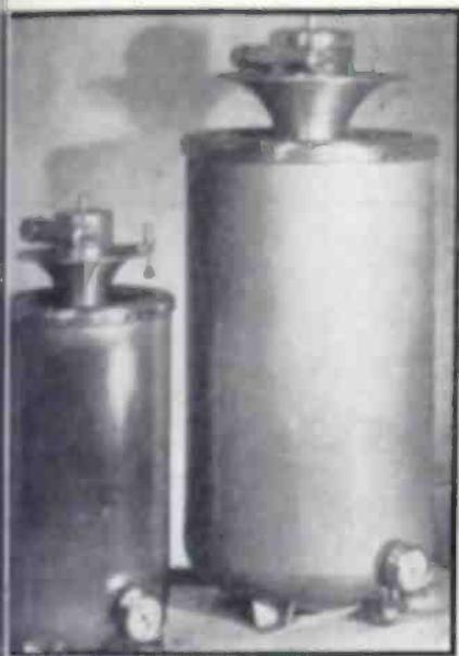
Two sizes of Lapp Insulator Co. pressurized capacitors show aluminum shells, gear head drives, and indicator pressure gauges. Also featured are adjustable provisions for external flash-over
