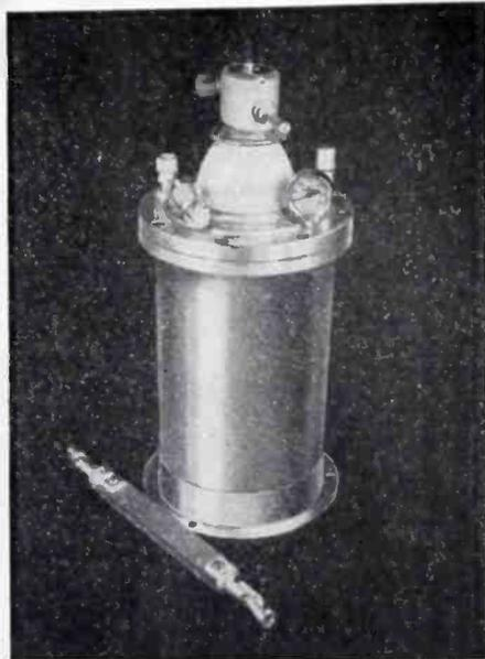
Pressurized, gas-filled capacitors made by E. F. Johnson Co. follow a basic design. Fixed and variable units both have copper-plated, drawn-steel shells in 6-in. diam. Miter-gear drive serves on variable version shown here
