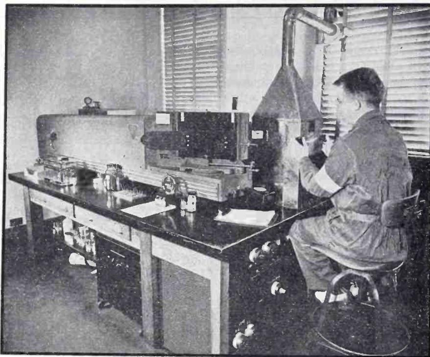
In this emission spectrograph, the samples to be analyzed are burned in an electric arc or spark in the hood at the right. The light emitted is broken into its spectrum by a quartz prism, and the spectrum is recorded on film
