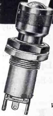
Designed especially for Aircraft, this Approved Pilot Light is compact, light, and mounts in  $\frac{5}{8}$ " panel hole. Finger pressure on head of unit closes bulb-testing circuit. Turning the knurled head regulates the intensity of light. Send for details.
