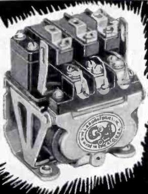
The exceptional efficiency of the G-M Type 27 relay is due in part to its two coil construction, with its great improvement in the relay's magnetic circuit. In ordinary relays the magnetic flux must be forced through the hinge air gap (Fig. A) with a consequent loss in efficiency. In G-M Type 27 relays this loss is avoided by providing a continuous path for the magnetic flux (Fig. B) through the iron structure of the relay and the working air gaps.
