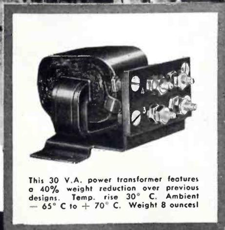
This 30 V.A. power transformer features a 40% weight reduction over previous designs. Temp. rise 30° C. Ambient — 65° C to + 70° C. Weight 8 ounces!
