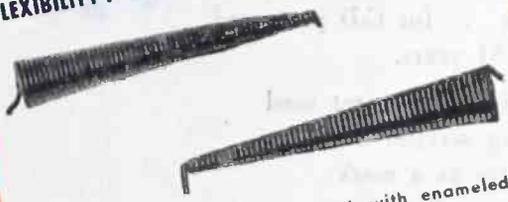
Formex wire (bottom) compared with enameled wire (top). The outer surfaces of the films have been elongated by stretching around a tapered mandrel and heating the samples to 150 C. Note the cracks on the enameled wire.
