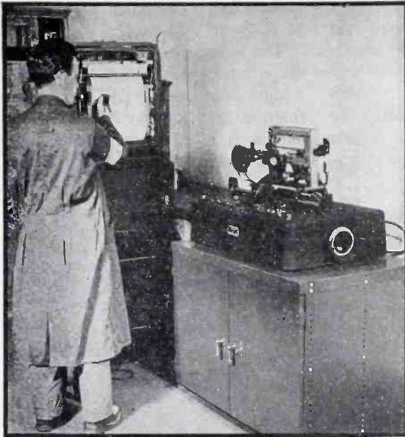
This Leeds and Northrup recording microphotometer can be used to measure the optical density of each spectral line on a photographic plate produced by an emission spectrograph
