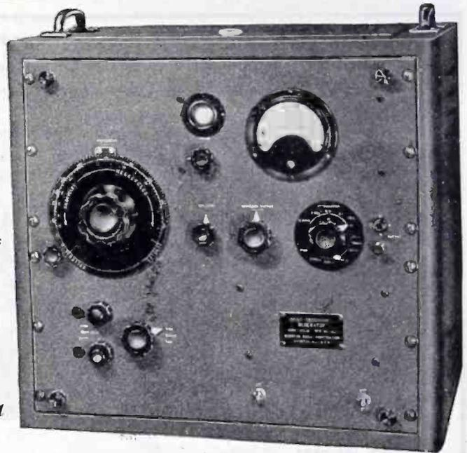
An accurate signal source capable of supplying a wide range of frequencies and voltages.
