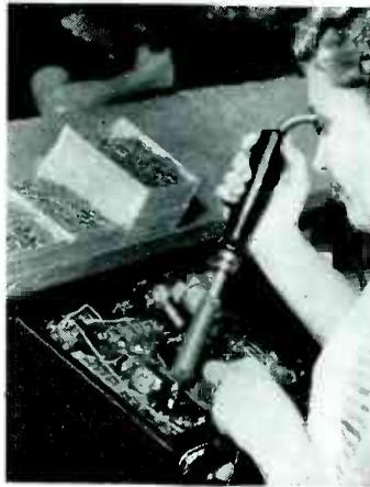
The patented, plastic rosin flux—self-contained in the core of the solder for fast, sure production—will not cause corrosion or injure insulating materials.
