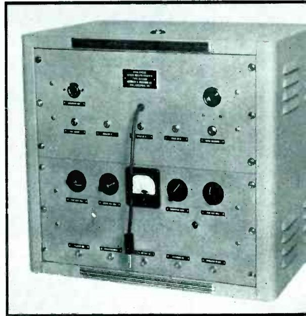
Fig. 6.—Complete vacuum tube scaling apparatus working on the trigger principle, containing pre-amplifier, recording end stage for the mechanical recorder, and a neon tube circuit for visual observation of the scaled pulses. It can be operated at scaling ratios of 2, 4, or 8 to 1, or without scaling, and with its regulated power supply and high-voltage source for the GM tube, represents a reliable apparatus for radiation measurements
