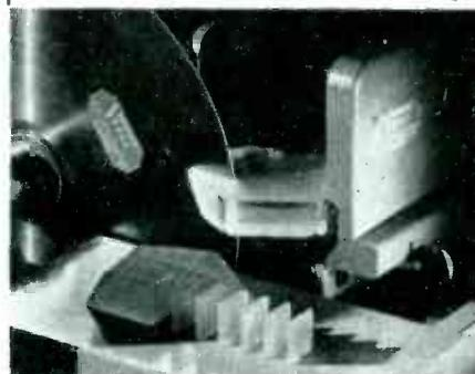
Quality Diamond Saws especially designed for the cutting of quartz frequency control crystals.
