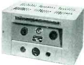
**RIDENOUR - LAMPSON IONIZATION GAUGE FOR MEASUREMENT OF PRESSURES IN REGION OF 10<sup>-4</sup> TO 10<sup>-7</sup> MM MERCURY**
