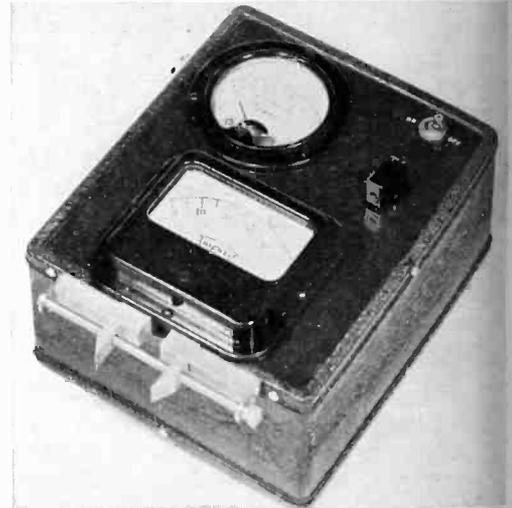
across the scale in accordance with the setting of the milliammeter, and indicates the comparative strength of the magnet. Variations of the rheostat-milliammeter control makes it possible to check magnets of different strengths. Source of current is self-contained No. 6 dry cell battery.
