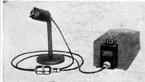
Converts Model 300 Voltmeter into direct-reading sound-pressure meter for sound and noise measurements, loudspeaker tests, etc. Comprises high-grade dynamic microphone accurately calibrated against Rayleigh disk, input transformer, attenuator and equalizer for compensating frequency curve of microphone. Range 30-10,000 cycles, reading down to 1 bar rms. Can be used with any Model 300 Voltmeter.
