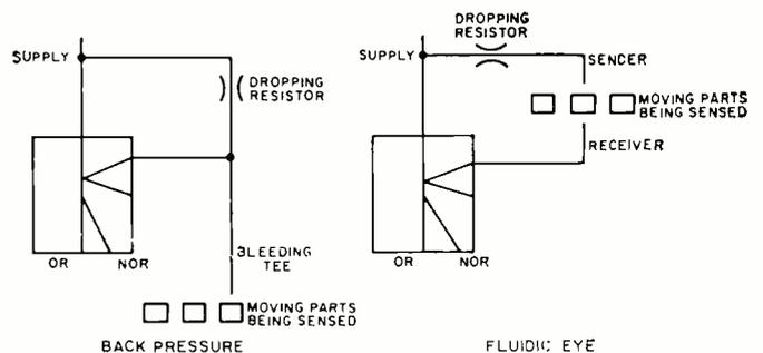
Fig. 8. Commonly used back-pressure and fluidic-eye type of sensors.
