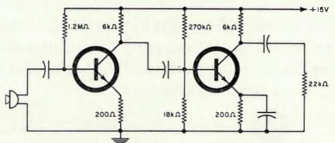
below a one-volt level. This represents a voltage ratio of 500; hence the pre-amplifier should have a voltage gain of 500 from input to output to drive a power amplifier with one volt r.m.s.
