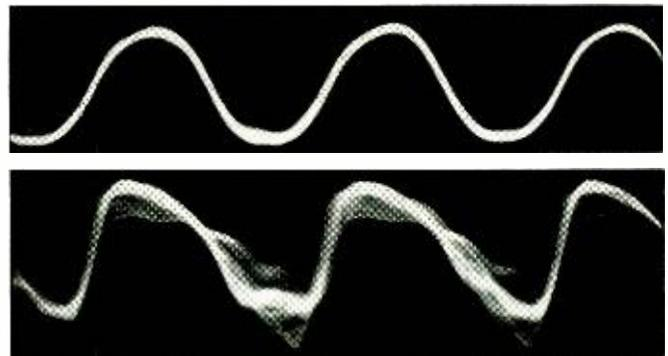
Fig. 2. Upper waveform is from a cartridge that is just barely tracking the sine-wave modulation. Lower waveform shows distortion produced when cartridge is not tracking.
