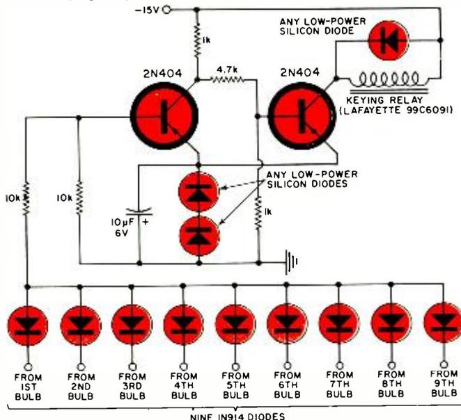
To monitor the nine left-most bulbs in the address register, we feed the signal from the nine indicator driver transistors to a circuit called an "and" gate. The word "and" implies that we get an output from the circuit only if the first signal is there, "and" the second signal is there, "and" the third signal is there, "and" so forth. The "and" circuit driving the relay is shown in Fig. 4.
