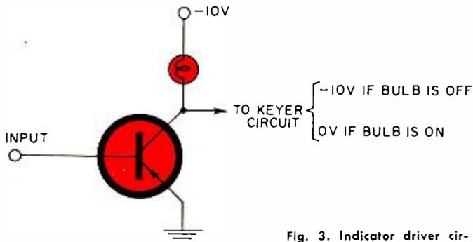
Fig. 3. Indicator driver circuit feeding indicator lamp.
