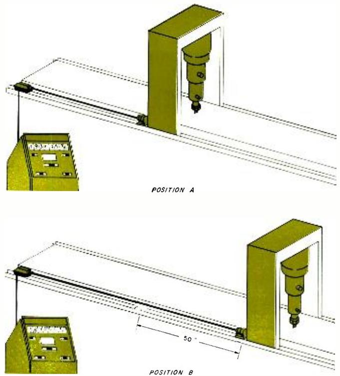
Fig. 3. An example of using a laser interferometer. Position A is the starting or zero point. At position B, the table has been moved 50 inches. Readout is by counter.
