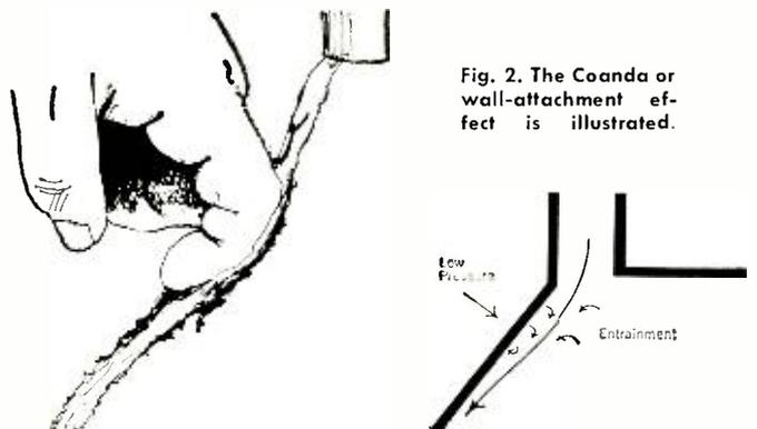
Fig. 2. The Coanda or wall-attachment effect is illustrated.
