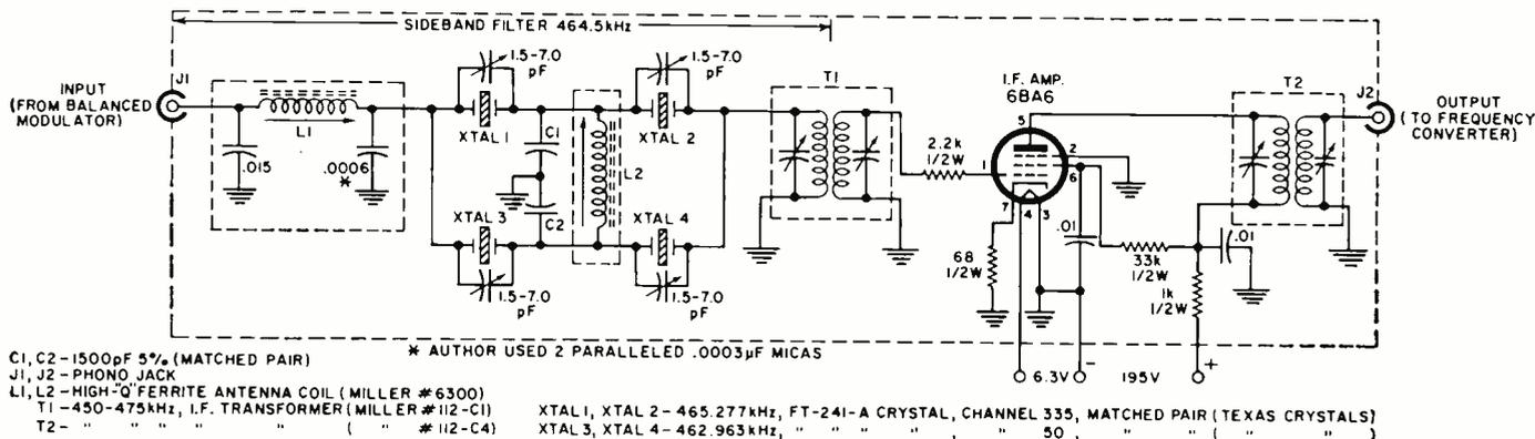
Fig. 1. Filter consists of two cascaded half-lattice crystal-filter sections with low-impedance input and high-impedance output.
