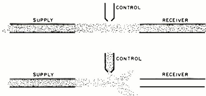
Fig. 7. Illustrating the principle of the turbulence amplifier.
