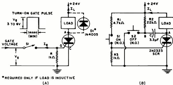
Fig. 2. (A) Basic SCR latching circuit. (B) An SCR latching circuit using a commutating capacitor to assist operation.
