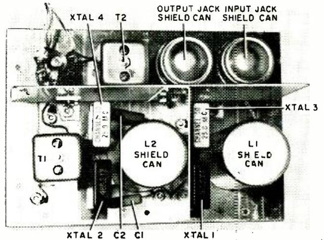
Fig. 3. Inside view showing parts placement and the internal shields. Coil and jack shield cans are in place in this view.
