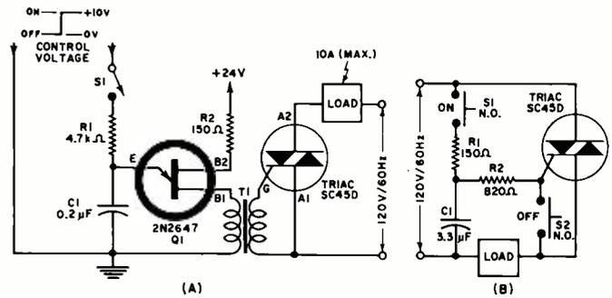
Fig. 5. (A) Low current isolated control of a large power load. (B) Triac connected in a typical latching circuit.
