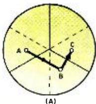
Fig. 2. (A) Top view of trihedral prism. Light striking point A is reflected to B, then to C. It then emanates and goes to detector. Distances AB and BC need not be equal. (B) A basic dual-beam interferometer using a trihedral prism.
