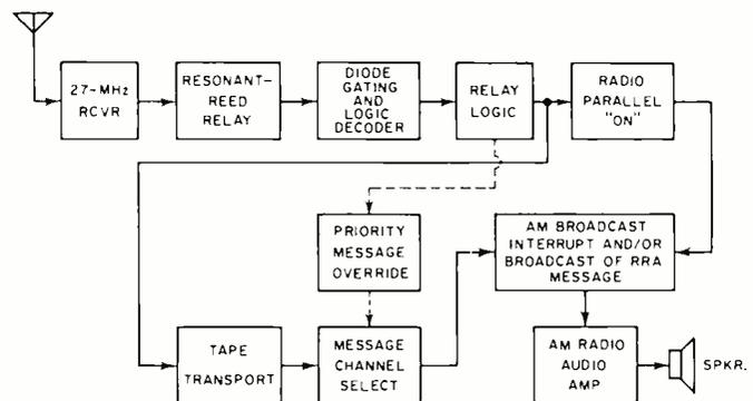
Fig. 1. When the RRA system picks up a tone-coded CB signal, a prerecorded tape takes over the car radio. Should a priority signal come in, it overrides other signals.
