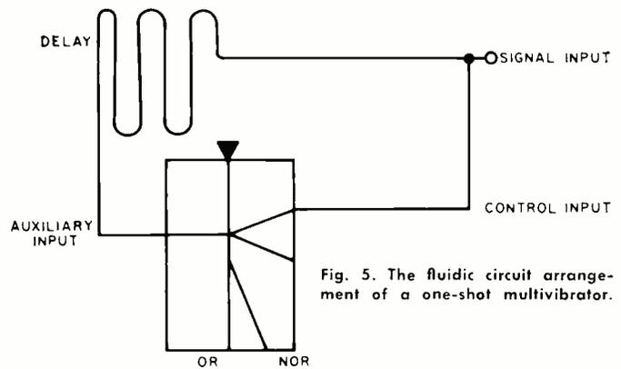
Fig. 5. The fluidic circuit arrangement of a one-shot multivibrator.
