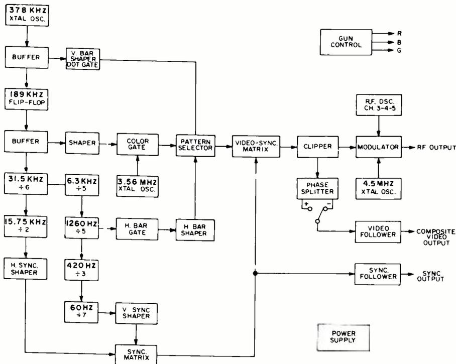
the receiver. The "Color Gun" control provides a means of making fast purity checks without disturbing the color screen controls of the receiver. Use of the gun control will also allow individual R-Y, B-Y, and G-Y displays to be viewed, thereby utilizing the picture tube to check color demodulation outputs and eliminating the need for an oscilloscope.
