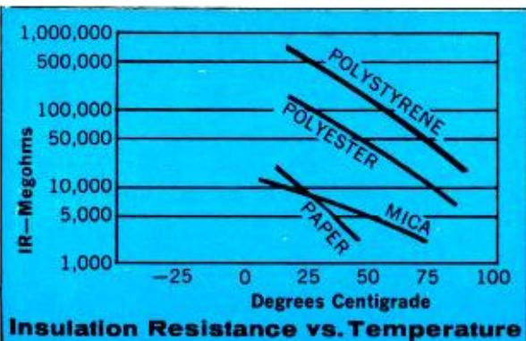
One more thing. Mallory Polystyrene Capacitors have the lowest dielectric loss in the business. Their dissipation factor (similar to power factor, a measure of efficiency as a capacitor) is extremely low . . . only 0.05%, which is a small fraction of that of other capacitors. And it stays at this low value over the whole temperature range. This means that they're high Q capacitors, ideal for tuned circuits. And their insulation resistance is way higher than polyester, mica or paper capacitors.
