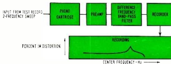
Fig. 6. Setup used for making the CCIF distortion measurement.
