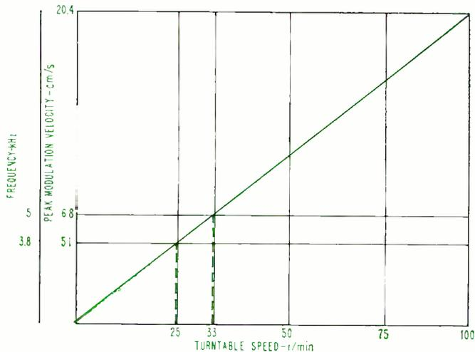
Fig. 3. Typical calibration chart for one band of special test record. Frequency and velocity vary as turntable speed.
