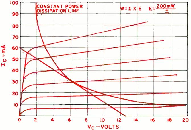
nal would be shown as a clipped, negative-going output voltage waveform, since the transistor would be saturated at this point. This would indicate that either the load resistor is too high (reducing collector voltage) or the bias resistor is too low (increasing base current).
