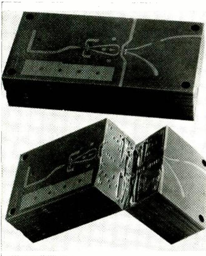
—some commercially available devices function at 700 to 1400 degrees C, well within most commercial and military requirements. Some fluidic devices are made from heat-fused ceramic material which is not affected by humidity or other adverse environments. And, since fluidic devices do not generate heat, system components are not damaged.
