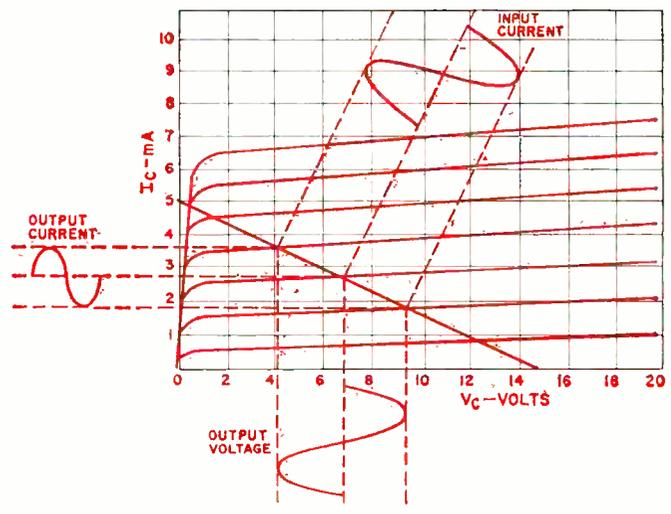
Fig. 3. Use of load line to show input and output currents, voltage.
