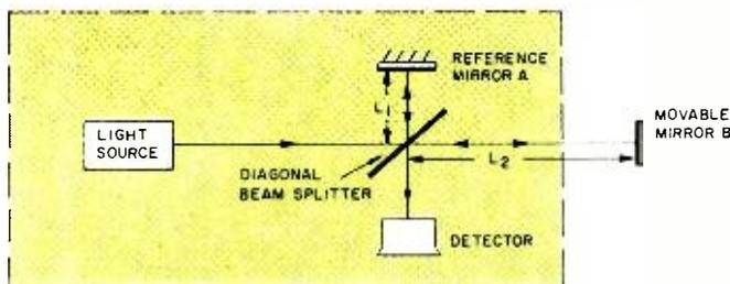
Fig. 1. Operation of the basic Michelson interferometer.
