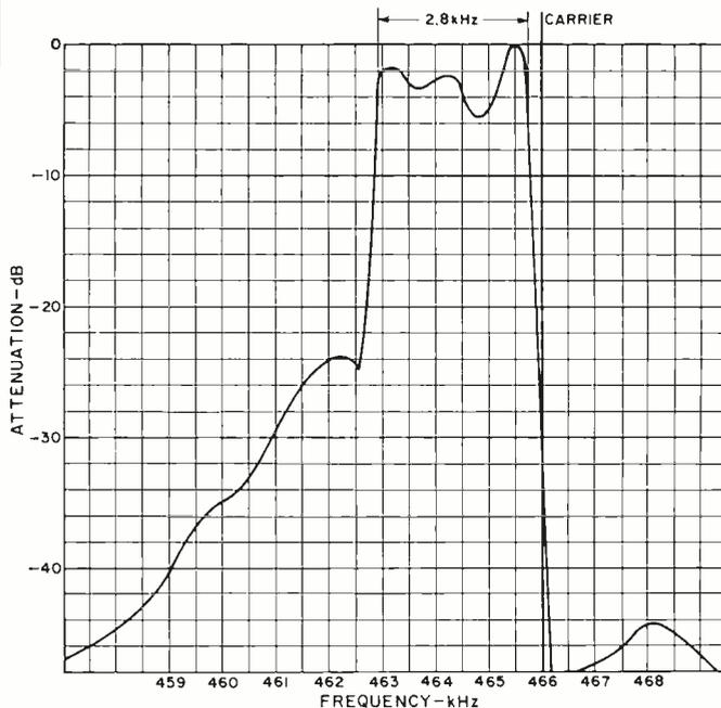
Fig. 6. The passband characteristics of the ferrite coil and crystal sideband filter are shown here after all the adjustments have been correctly made. Note the position of the carrier along the steep h.f. skirt.
