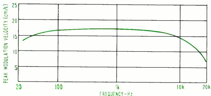
Fig. 4. Typical tracking-ability curve showing maximum modulation velocity the cartridge can track as function of frequency.
