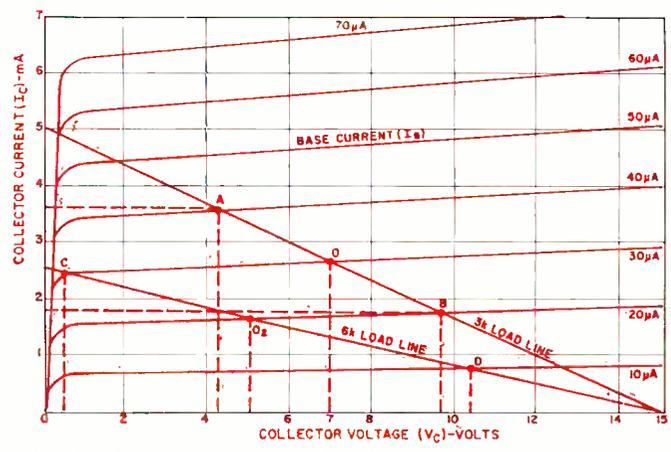
Fig. 1. Characteristic curves for the type 2N2712 transistor.
