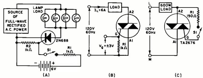
Fig. 4. (A) Basic application of SCR in a lamp-driver circuit. (B) Basic application of a gated bi-directional controlled rectifier. (C) The power line triggers the gated bi-directional controlled rectifier when switch S1 closes.
