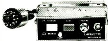
push button switches for standby, normal, call, and reset. There is a volume control and indicator light.
