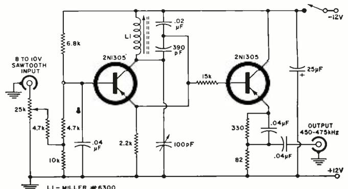
Fig. 7. Complete circuit diagram of the test sweep generator used by the author to develop the response curve of the filter.
