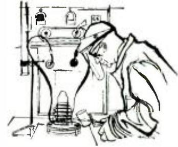
**T**HE cover photograph shows D. R. Ginter, a technician in the Semiconductor Laboratory of the Chemical and Metallurgical Division of Sylvania Electric Products Inc., at Towanda, Pennsylvania, operating equipment for the melting and casting of silicon. The silicon is being melted under a protective cover by power supplied from a radio-frequency oscillator through a fourteen-turn coil. The resultant eddy currents cause intense heat to be produced.
