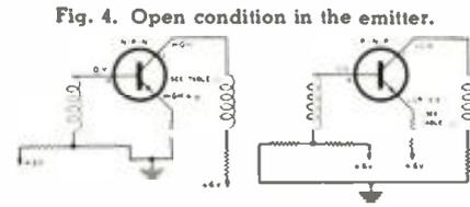
Fig. 4. Open condition in the emitter.
