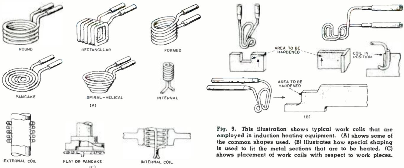
Fig. 9. This illustration shows typical work coils that are employed in induction heating equipment. (A) shows some of the common shapes used. (B) illustrates how special shaping is used to fit the metal sections that are to be heated. (C) shows placement of work coils with respect to work pieces.
