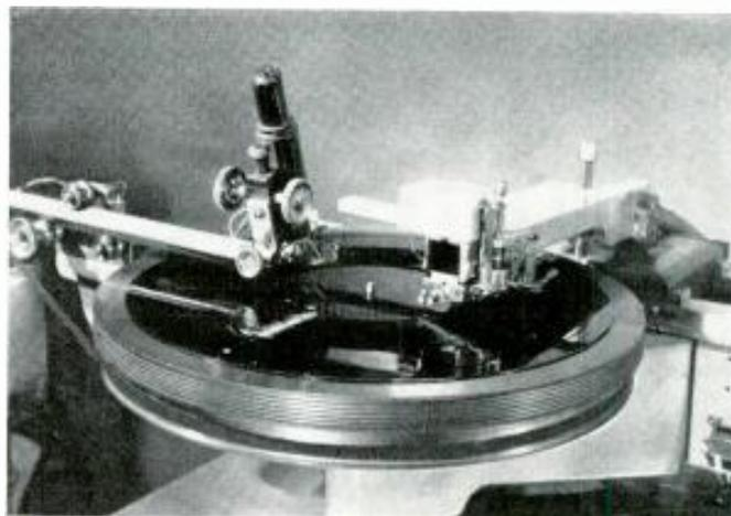
Close-up view of the master recording lathe that was used.
