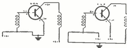
Fig. 7. Open lead in transistor base.
