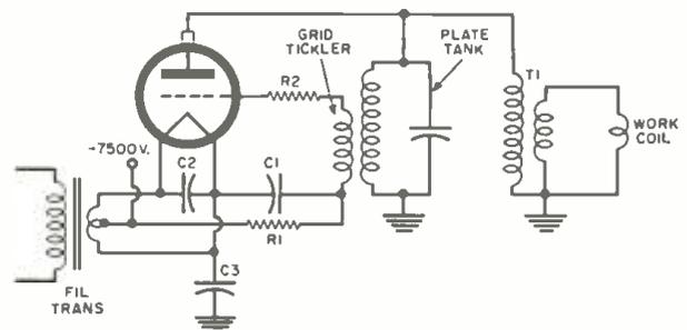
Fig. 12. Simplified diagram of a 20-kilowatt induction heating generator.
