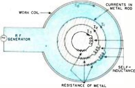
Fig. 6. Cross-section of currents in rod.
