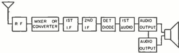
Fig. 5. Block diagram for deluxe transistor portables.
