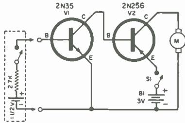
Fig. 2. Diagram of a less sensitive motor control circuit. An input control signal of  $\frac{1}{2}$  milliamperes will operate the motor. The several components within the dashed lines may be used for testing the circuit. These will provide an input control current of  $\frac{1}{2}$  ma. A penlite cell may be employed.
