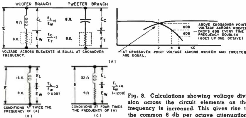
Fig. 8. Calculations showing voltage division across the circuit elements as the frequency is increased. This gives rise to the common 6 db per octave attenuation.
