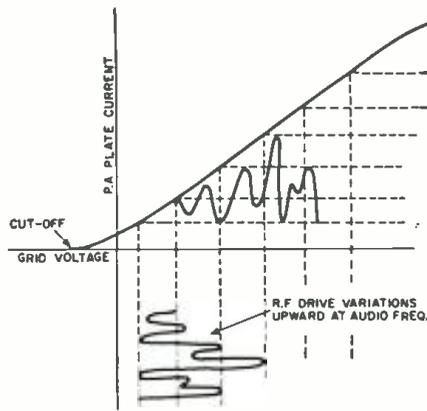
Fig. 4. How r.f. drive to power amplifier prevents p.a. cut-off, and constantly changes grid operating point at a.f. frequency.
