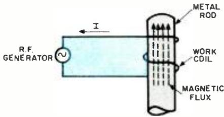
Fig. 5. Basic relation between r.f. generator, coil, and the rod to be heated.
