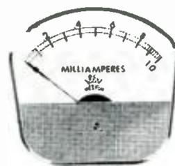
ments provide longer scale lengths, shadow-free scale illumination, interchangeable components, and accuracy ranging from ±5 per cent to ±2 per cent.
