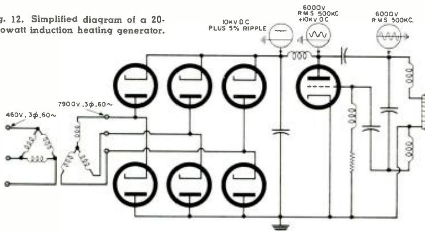
for maximum power output for each individual work piece. To minimize the external shielding required, the entire generator is housed in a grounded, electrically bonded cabinet.
