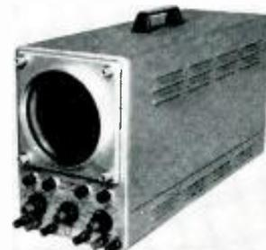
five-inch d.c. oscilloscope to its line of assemble-it-yourself test instruments. The circuit features identical d.c.-coupled vertical and horizontal ampli-
