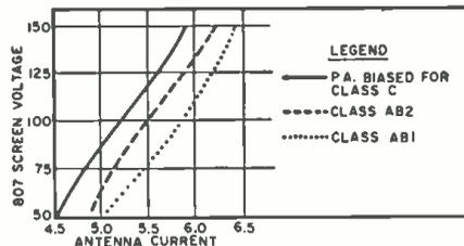
Fig. 5. Actual antenna current values for several values of buffer screen voltage.
