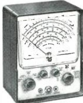
Exclusive larger 6-INCH 400 uA meter movement, edge-lighted, within 2% accuracy • 1% precision multiplier resistors • 7 AC (RMS) and DC ranges • 7 AC (peak-to-peak) ranges • resistance, dB, and other essential ranges • 12AU7 for DC ranges, 6A15 for AC • transformer operated selenium rectifier • durable plastic case.
