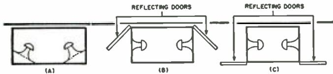
Fig. 6. Three basic constructions used for unitized cabinets.
