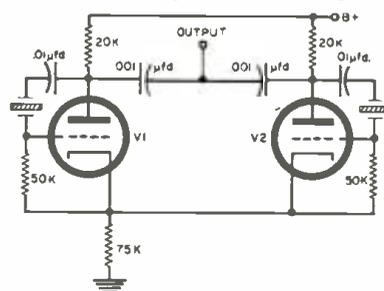
Fig. 3. Using the circuit to determine frequency of an unmarked crystal.
