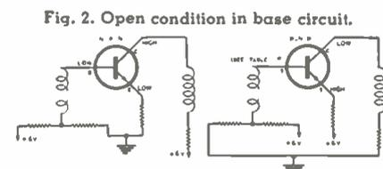
Fig. 2. Open condition in base circuit.
