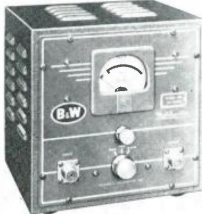
direct-reading r.f. wattmeter and standing-wave-ratio bridge. It is suitable for applications where adjustment of radio transmitter power output must be checked before going on the air as well as other uses.
