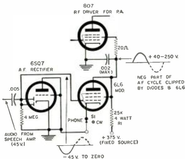
Fig. 2. Triode-connected 6L6 modulator is clamped to r.f. driver screen. Modulator draws current of only 13 ma. on zero audio.
