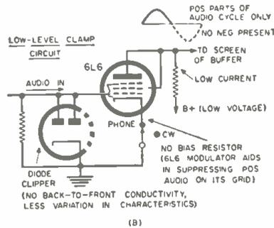
Fig. 1. Changes made in early clamp-tube circuit to allow low-level modulation, less power consumption, and lower voltages.
