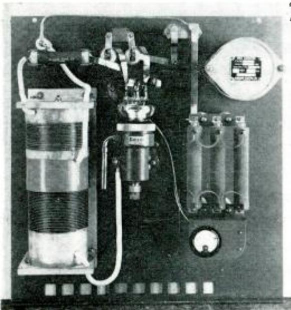
Fig. 10. Interior view of generator of Fig. 8, showing the r.f. oscillator.
