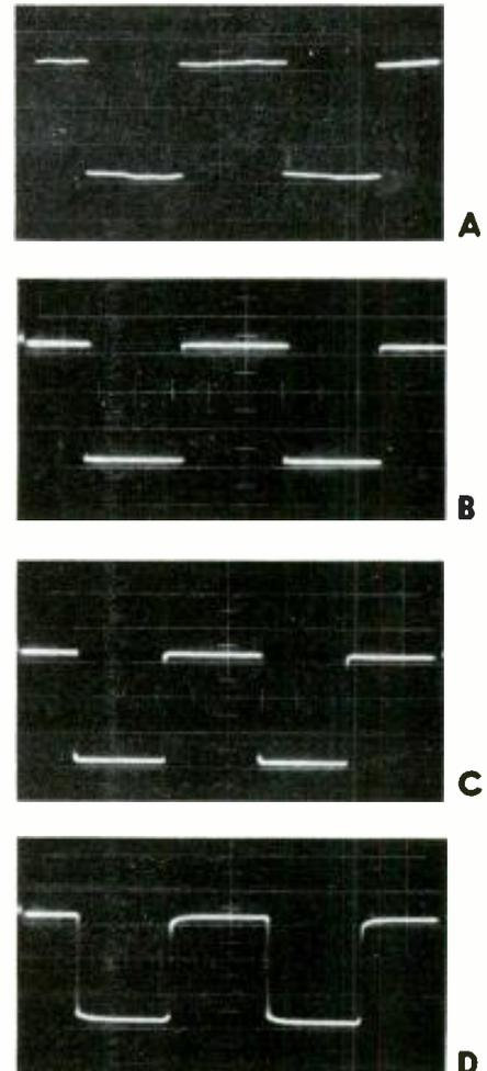
Fig. 6. Intermodulation distortion measurements with clipping point shown (16-ohm load).
