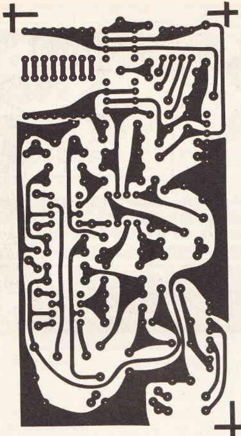
The modular pre-amp input stage solderside foil
