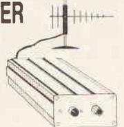
Based on the OM335 hybrid amplifier, the booster has specifications to rival the best, widest-band operation from 10MHz to 1.4 GHz, mid-band gain of up to 26dB and a wide supply range of 6V to 26V (it will run from car batteries for caravaners, dry batteries for campers, or a mains 'battery eliminator' in the home). No special UHF construction skills are needed - the project could be made by a careful beginner.
