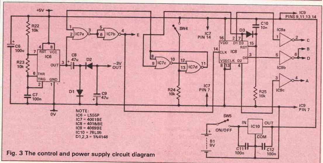
Fig. 3 The control and power supply circuit diagram
