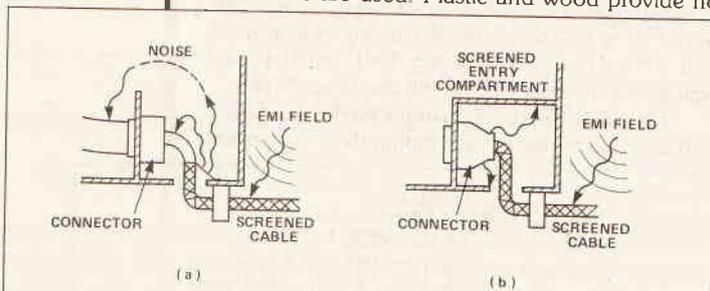
**Fig. 3 (a) Radiated EMI can enter a screened enclosure via a screened lead but (b) can be prevented with good practice**
