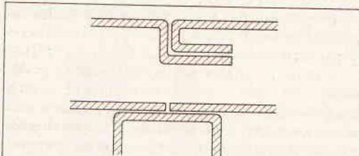
**Fig. 2 Seaming techniques for metal enclosures and internal shields**
