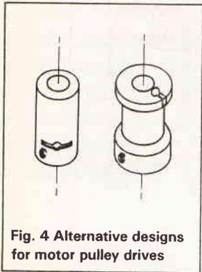
Fig. 4 Alternative designs for motor pulley drives
