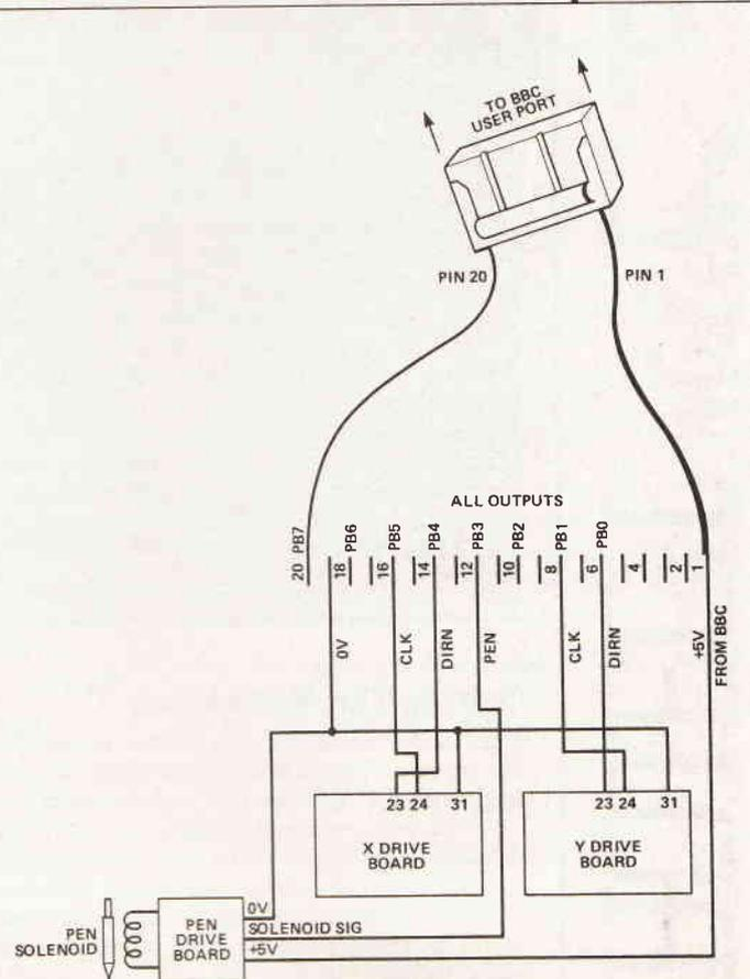
Fig. 7 Connections to a BBC computer
