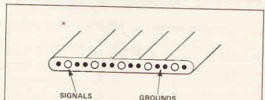
**Fig. 4 Signal wires in ribbon cable should be separated by earthed wires, effectively screening signals**
