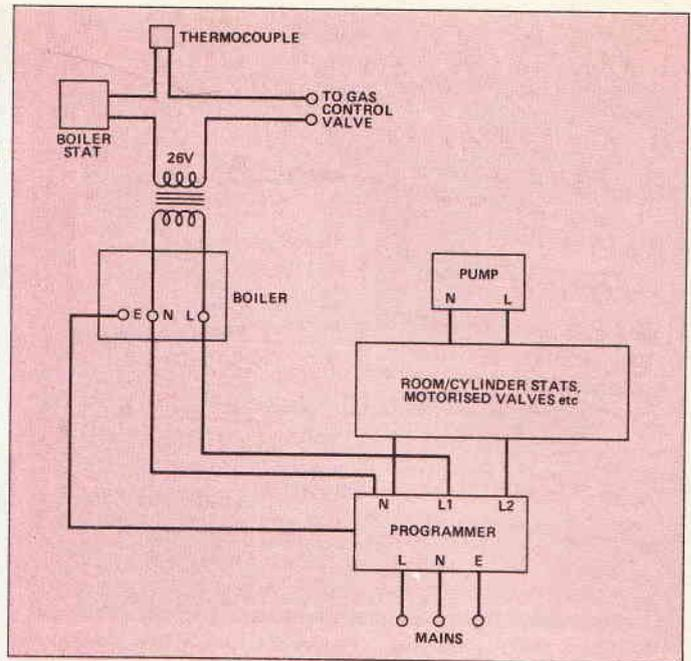
24V on the external circuits for safety reasons. It would certainly seem risky to use mains on a room thermostat unless its cover were made stronger than most I have seen in use.
