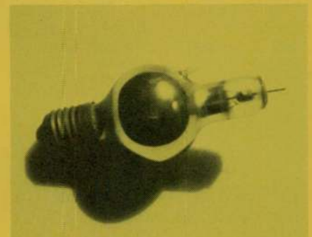
Fig. 8 Hot-cathode construction for mercury-vapor rectifier tubes.
