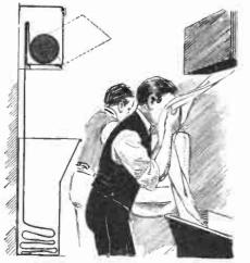
No. 1,514,400, issued to Frank M. Steiner, describes an improved type of towel holder for washrooms, wherein the same section of the toweling is used only once. A roll of absorbent cloth is kept in the hinged cabinet as illustrated above and when a clean section is desired, it is pulled down and the remainder allowed to collect as shown.
