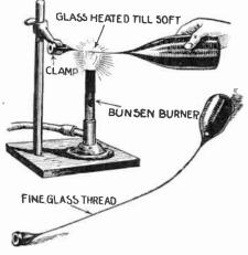
Fine glass threads are often required in various experiments. They may be quickly and easily made as illustrated above. Clamp the neck of a bottle in position and then heat the point shown. When the glass is softened, throw the bottle as far away as possible. A long fine glass thread will result glass thread will result.
