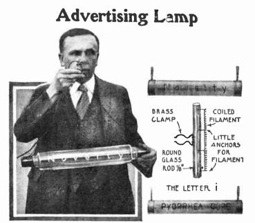
The novelty lamp illustrated above is the invention of Mr. H. Hartman. Upon a glass rod running from one end of the lamp to the other, a number of letters are clamped. These letters are of glass and contain little anchors which hold the filament. Three or four letters are connected in series and the groups then connected in parallel to the line wires. These are placed in the glass tube, which is then evacuated. —Holmes Feature Service. Science and Invention for May, 1925
