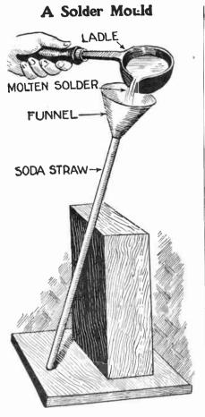
Usually after wiring up a set there is a con-siderable amount of solder left over. Melt the solder in a ladle and pour the molten solder into a soda fountain straw. By re-moving the straw after the solder has solid-fied or "set" a handy length will result. --C. F. Felstead.
