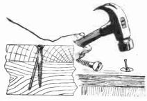
No. 1,518,119, issued to Warren C. Rees, covers the design of wood screw which is to be locked in position by means of a nail as illustrated above. It is impossible for a screw of this nature to loosen.
