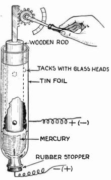
Take the bottom off a long, narrow bottle. Cork the bottle up tightly and force a stout copper wire through the cork. Coat the out-side of the bottle with tin-foil. Pour mercury almost up to the height of the tin-foil. The device is operated by a handle which presses the plunger down and thereby raises the mercury in the bottle. -V. Wardinhausen.
