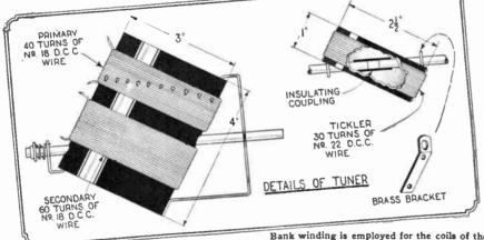
Bank winding is employed for the coils of the tuner, although any standard three-circuit coupler can be used.
