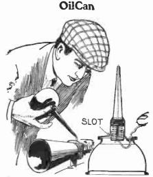
No. 1,520,829, issued to Gustave Lidseen, covers a type of oil can which cannot spill even though upset. Furthermore, a measuring device is incorporated which, if desired, allows only a certain amount of liquid to escape. Both the measuring and the sealing devices are actuated by a finger lever as indicated above.
