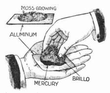
A pretty experiment involving the preparation of aluminum oxide may be performed as above. Place a few drops of mercury on a strip of aluminum and rub briskly with steel wool for a few seconds. A moss-like substance, alumi-num oxide will "grow" on the aluminum. -Arthur A. Blumenfeld.
