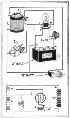
Herewith is shown a fundamental oscillatory circuit.
