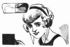
No. 1.514,152, issued to Hugo Gernsback, protects a soft pliable cushion of a highly resilient material designed to be placed over the cap of a radio or telephone receiver, making the same more comfortable in use.
