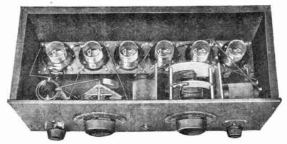
Note the interior of this well designed set. All parts are separated so as to eliminate to a greater extent the feed-back which would otherwise occur. The denser to the right is a special type, and as can be seen, is well shielded. The con-The audio frequency transformers are also shielded and placed under the tube rack toward the back of the cabinet. By the use of the best type of transformer, dia-tortion in the audio circuit is eliminated.
