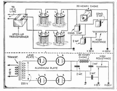
No modern set is complete unless a good "B" battery eliminator is used to supply the "B" voltage to the plates of the tubes. By the use of large condensers and correct size choke coils the AC ripple can be eliminated.
