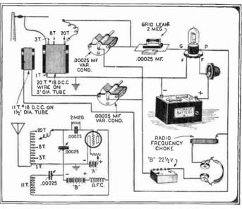
Short waves are rapidly coming into use for broadcasting purposes on account of the greater carrying powers and less fading experi-enced on these waves. The circuit shown is the latest Reinartz type.
