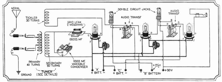
Five jacks, one each for the aerial and ground, detector and first and second atages of amplification afford very handy connection terminals. The antenna is a coil of bell wire 125 feet long which, when not in use, is placed in the
