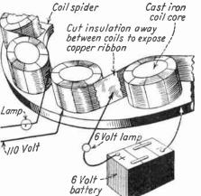
When testing magneto coils as above, if lamp lights, the coil is grounded. Replace with an-other one. Such trouble is indicated by consistent missing of the engine, not traceable to other causes.
