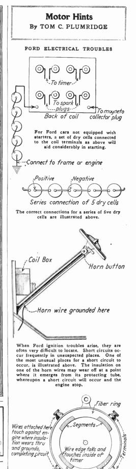
Other ignition troubles often occur at the commutator illustrated above. The wires connected to the terminal may become frayed and so short circuit to the commutator housing or the engine frame. Also the segment may become badly worn, whereupon a new timer should be installed.
