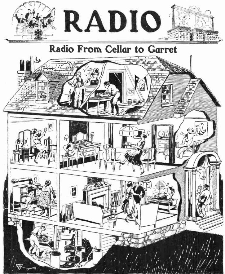
The loud speaker system installed in this house is quite easy to duplicate. A pair of wires run through all rooms where a loud speaker is wanted. The loud speaker is then plugged in at will by the use of a jack and plug system.
