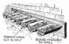
A rack for holding various small parts around the shop may be made from several tomato cans cut in half and mounted as shown above. -F. J. Wilhelm.
