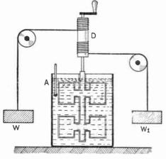
The simplest method for the determination of mechanical equivalent of heat is shown above.
