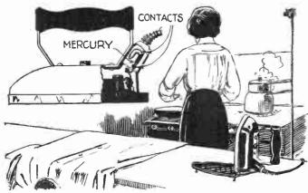
No. 1,511.382, issued to Dayton Ulrey and Daniel I. Mayne, covers several designs of fluid circuit breakers, the most basic of which is illustrated above. A conducting fluid, preferably mercury, completes the circuit when the electric iron is horizontal. The circuit is broken when the iron is tilted and so prevents overheating and waste of power.
