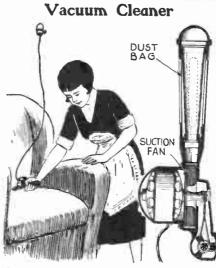
No. 1,596.231, issued to Frank W. Finkhousen, describes a novel type of portable vacuum cleaner which is entirely self-contained. Above at the right is shown a cross sectional view of this device. A small dust bag is incorporated in the handle. An electric motor operating from the house current turns a fan which in turn is belted to a small brush as shown.
