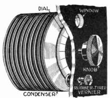
A novel effect is obtained when a dial is mounted in back of a panel. The dial num-bers are viewed through a "window" drilled through the panel. -J. Liebowitz, Reporter No. 2939.
