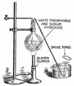
By setting up the apparatus as shown above and boiling the solution, phosphine will be evolved and when the bubbles reach the surface of the water in the beaker, they will spontaneously catch fire and form smoke rings. Before starting experiment, it is advisable to pass illuminating gas through the flask to remove all the oxygen that may be contained therein. The second tube shown is for this purpose.
