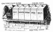
Another rack for various parts may be made of large cocoa cans placed on a shelf which does not extend quite to the edge of the can. A rod passed through them serves as a pivot. -F. J. W.
