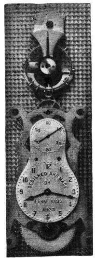
The clock here illustrated measures 8½ inches high, and except for the main spring and hold jewels, was designed and constructed entirely by hand by the author. The hair spring is made of piano wire and the metals of the balance are fused together instead of being soft soldered. It loses less than 30 seconds during a week. ---W. L. Bass.
