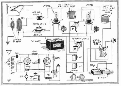
The low power broadcasting set shown above can be used to communicate with stations about 10 to 15 miles apart. The modulation system is of the best and latest design.
