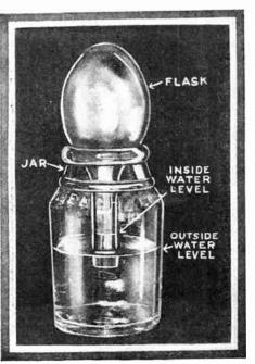
One of the simplest weather forecasters is the water barometer. A simple one may be made as shown above. A flask of any available size is inverted in a jar which is half full of water. It will be found that the water will rise or fall in the neck of the flask in accordance with atmospheric pressure. A rise indicates fair weather, while a fall means a change. —S. Leonard Bastin.
