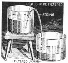
By wetting an ordinary cotton string, it may be used as a filter as shown above. The end from which the filtered liquid drips must be lower than the surface of the liquid to be fil-tered. —Arthur A. Blumenfeld. tered.
