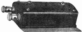
A miniature phone block which will accommodate 11 pair of phones, seven in series and four in parallel, is a very handy device which can easily be constructed upon the dimensions given in the diagram. A small block of wood is drilled and fitted with short lengths of thin copper strip. A piece of rubber tubing acts as a spring, effecting good contact. A fibre cover is screwed to the top, giving a pleasing appear-
