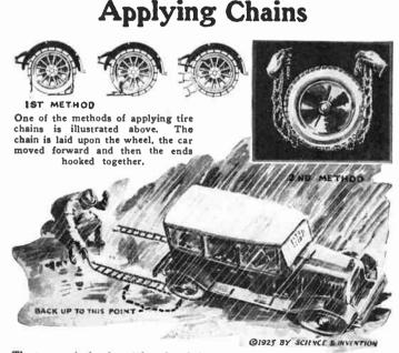
The two methods of applying tire chains to automobiles indicated above are found to be the most practical under all weather conditions. In the first, the chain is placed over the wheel, the car moved forward for a distance about a foot, and then the ends of the chain are hooked together. In a second the chain is laid upon the ground, the car backed upon the chain, and then the ends lifted and hooked together as shown.
