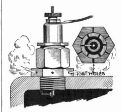
If holes are drilled in the shell of a spark plug as well as in a nut which fits the shank of the plug, carbon may be quickly removed from the porcelain by turning the nut so that the holes line up and running the engine for a few min-utes. When in ordinary use the holes must be turned out of line. —M. Mather.
