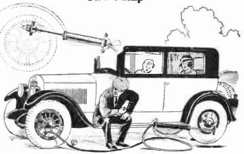
No. 1,520,249, issued to Elmer Kaufmann, provides protection for the type of tire pump clamps illustrated above. One end of the pump is secured on a swivel to the running board of the car, whereupon the handle is fastened by another swivel clamp to one of the rear wheels which is jacked up and turned by means of the motor.
