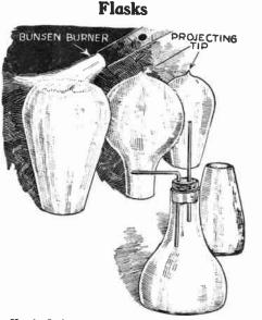
Handy flasks may be made from various types of electric light bulbs. The brass base is cut off and the edges of the glass rounded. If flame is then applied to the opposite end, the glass will be depressed so as to form a base. -G. M. Blackford.
