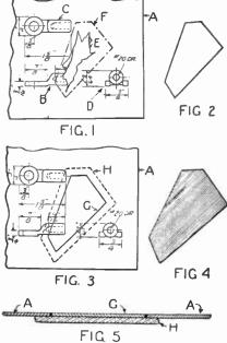
When a tracing is mutilated as shown in Fig. 1, it may be restored. The tear is at E. A second sheet of tracing paper is placed beneath the drawing and a section, F, is cut from both cloths, obtaining a strip from the new sheet which will fit into the removed portion of A. The new piece is placed and fastened with an overlapping strip and collodion. In Fig. 5, A is the original sheet, G the replacement, and H the binding strip. The removed portion is redrawn on the new piece. —Gustavo Gallopin.
