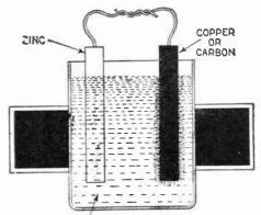
DILUTE SULPHURIC ACID The simplest form of galvanic battery con-sists of a carbon or copper rod and a zinc plate immersed in dilute sulphuric acid.
