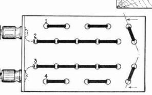
Between numbers two and three, five pair of phones can be conin parallel. nected If desired, these phones can be connected in series, by simply plugging in the proper places. A 3/16ths inch drill is used to make all the necessary holes. The device will find a large use where man phones are used. many
