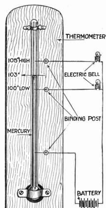
Heating alarms of the type illustrated above are by no means new and furthermore are not as efficient or as cheap to manufacture as thermostats. It is therefore not advisable to patent a device of this nature.
