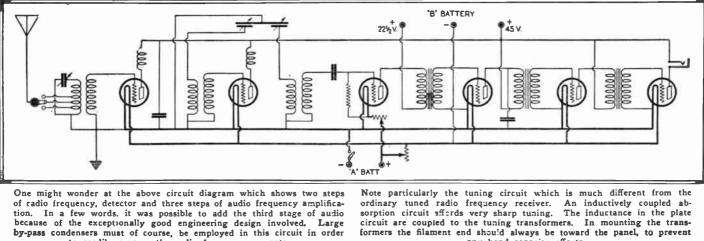
One might wonder at the above circuit diagram which shows two steps of radio frequency, detector and three steps of audio frequency amplifica-tion. In a few words, it was possible to add the third stage of audio because of the exceptionally good engineering design involved. Large by-pass condensers must of course, be employed in this circuit in order to readily by pass the radio frequency currents.
