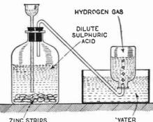
This shows a laboratory set up for the preparation of hydrogen gas.
