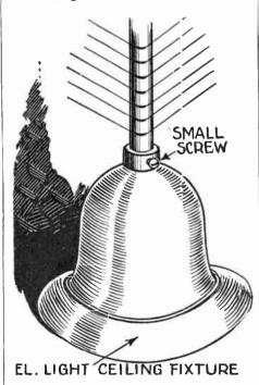
An electric light ceiling fixture makes an ex-ceilent mounting for a loop aeria. The base of the loop is inserted into the fixture as shown, and is held in place by the screw. —C. G. Switzer.
