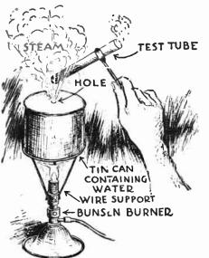
When materials in a test tube have to be carefully heated, the device illustrated above comes in very handy. A small tun can is fitted with a wire support and held above a Bunsen burner. Water is poured into the tin can and the cover, with a hole punched therein, placed in position. Heating the water soon evolves steam which in turn may be used to hea. the test tube. —Robert Rogers, Reporter No. 11,229.
