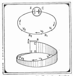
The above is a graphic illustration showing the fall of potential in a dry cell.
