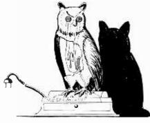
No. 1,727,002, issued to William B. Weaver. This lighter is a novelty using the form of an owl to contain coils which are heated to incandescence. The eyes of the owl contain the coils which are heated to incandescence; the base of the figure is equipped with an off-and-on switch. When the eyes light up they give the impression of an oxel blinking.
