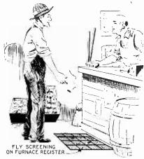
IN many cases trouble is experienced when customers knock small bits of paper, peanut shells and even coins down the furnace register. To alleviate the difficulty, remove the grill, cover the underside with fly screening and wire it to the grill.—A. C. Wilson.
