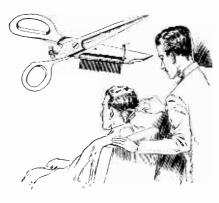
No. 1.726,390, issued to John W. Erhard and Antoinette Erhard. This patent relates to a device for combing and cutting the hair and also a means of gauging the length of the hair cut off. It consists of a pair of scissors, two shear members pivotally connected, a rod with a comb on it and a rack and pinion for rotating the comb upon opening and closing the scissors.
