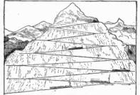
Diagram shows the switchbacking arrangement to obtain altitude of 17,000 fi. above sea level. American tocomotives are the standard equipment used for hauling the loads up the steep inclines.
