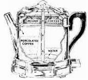
Here are the details of the new coffee pot. As the water on the right side is heated, the steam generated drives it up through the tube and over the ground coffee. The coffee dripping through, settles in the left compartment.
