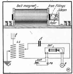
Electro-magnetic Control for Detector.
