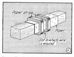
Fig. 3. How Form Is Constructed for Winding Galvanometer Coll.
