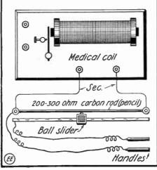
Potentiometer Method of Regulating Shock Coll Secondary Current.
