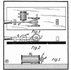
Release Magnet Coll Fitted to Lightning Switch.
