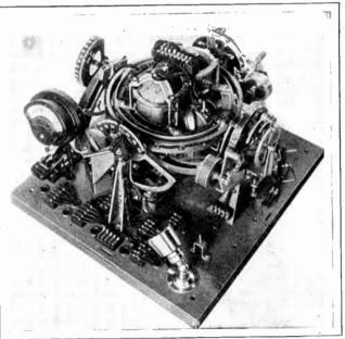
Fig. 6. Automatic Gyroscopic Stabilizing Set for Aeroplanes.
