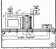
Scheme for Hooking up Telegraph Sounder to Act as Buzzer.
