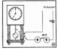
Clock Pendulum Makes and Breaks Test Buzzer Circuit.
