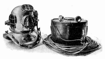
Fig. I, Telephone Set as Adapted to Divers' Helmets.
