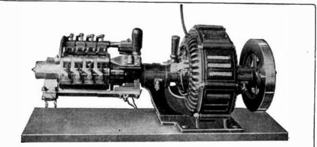
Motor Driven Rectifier for Heavy Loads and Capable of Converting Alternating Current Into Direct Current.
