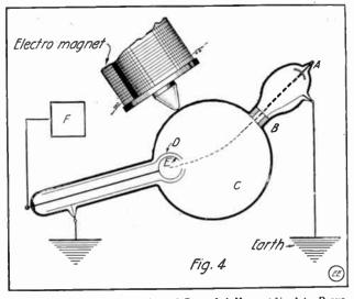
Fig. 4.—Evacuated Glass Bulb and Powerful Magnet Used to Prove Cathode Rays Are Negatively Charged Particles.
