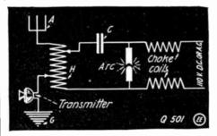
Wireless Telephone Hook-up for Arc Generator A. 2. The diagram given in the article which you mention can be used for wireless telephony.
