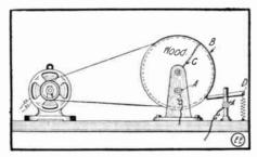
Easily Made Rotary Flasher for Battery Lamps.
