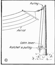
Scheme for Raising Aerial by Means of Ratchet Wheel and Crank.
