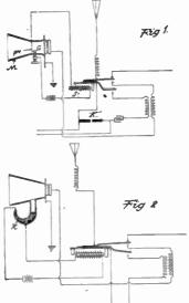
is connected to the antenna and ground. A second scheme for ac-complishing identically the same re-sults is shown in Fig. 2 and in-volves the capillary action of a small quantity of mercury placed in the tube R of the shape indicated, which connects and disconnects the relay circuit as aforedescribed and for similar purposes.
