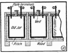
Scheme for Repairing Cracked Storage Battery Jars.
