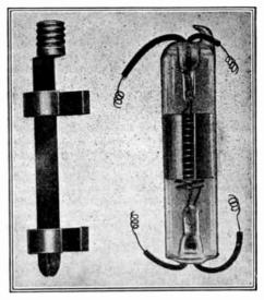
Latest Audion Detector and Holder Adapted to Screw Into Any Standard Socket.
