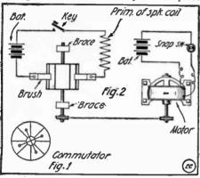
Utilizing Regular Commutator as Spark Coil Interrupter
