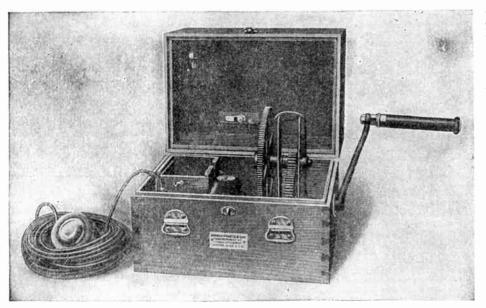
Fig. 2. Turning the Crank Whirls a Small Dynamo, Which Furnishes Current for the Divers' Hand Lamp.
