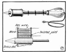
A Useful Electrically Heated Soldering Iron. up well by filing to a good point, then tin it thoroughly. Procure several sheets of thin mica (about .002 inch in thickness) and wrap it around the iron until you have five or six layers on. Obtain 20 feet of No. 26 nichrome resistance wire and two No. 16 asbestos-insulated copper feet of wire.
