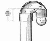
indicated and adapted to fit a pen-cil and also to contain an electric lamp receptacle. Two wires from the receptacle lead out to an exter-nal battery. This device would seem adaptable to use with a foun-tain light battery, which is already on the market.
