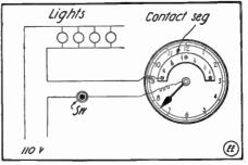
Time Switch Constructed from Any Clock. switch with relay attachment is best employed in such circuits. Contributed by LOUIS GOODMAN.
