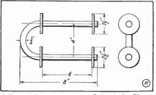
Powerful Electro-magnet Suitable for Use on Batteries.
