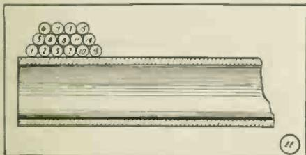
How "Staggered" Windings Are Built for Radio Purposes So As to Reduce Distributed Capacity.
