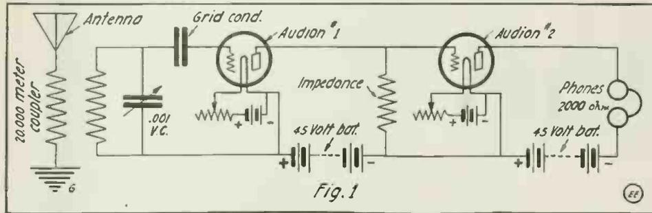
Diagram of Circuits for 20,000 Meter Undamped Wave Audion Receiving Set Which Has Given Highly Satisfactory Results.
