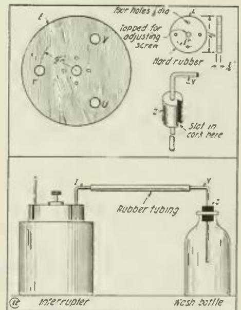
Details of Low Voltage Electrolytic Interrupter and Arrangement of Wash Bottle for Neutralizing the Gas Fumes Produced.
