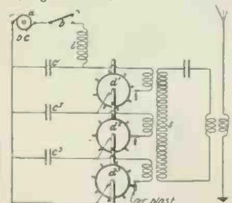
continuous oscillations intended for use in wireless telegraphy and telephony. Several series of insulated rotary spark gaps with compressed air
