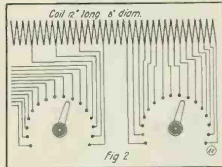
Connection Scheme for Primary of 20,000 Meter Loose Coupler.
