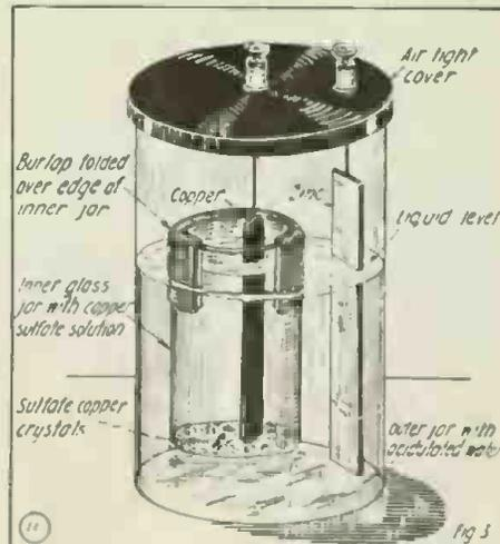
Finally the Gravity Cell Research Work Bolved Down to the Type Shown. The Copper Sulfate Oozed Out By Capillarity Thru Several Layers of Burlap Dipping in Both Solutions.
