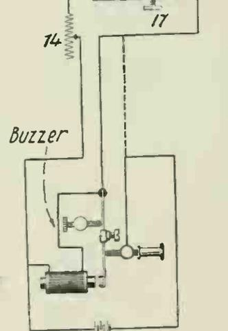
The apparatus in question consists of a telephone receiver connected with a circuit comprising a battery and a rapidly interrupted switch or contact, such as a buzzer.
