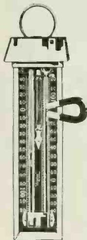
As the temperature fluctuates the mercury will rise in one side or the other, leaving the index in either case to show when the next reading is taken what has been the highest degree of heat or cold since the thermometer was last set.
