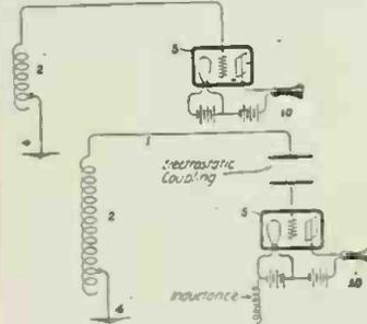
represents the aerial circuit, containing a tuning inductance 2, which is connected to the earth or a suitable capacity at 4. The aerial 1, preferably consists of a long horizontal conductor connected to the earth. The free end of the aerial being a point of maximum potential, is connected to a vacuum detector 5. The patent mentions the use of an inductance connected to the filament circuit as shown; this inductance being adjustable.
