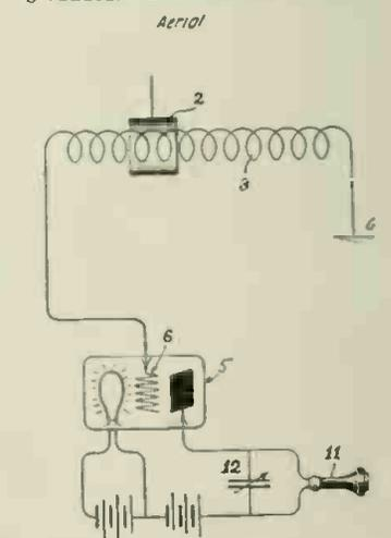
ductance coil is connected to the grid of vacuum bulb detector used in the manner shown, or a crystal detector may be used instead. It is seen that electrostatic coupling is thus employed and in tuning such a receiving set metal ring 2, is moved along coil 3, and also the degree of coupling may be varied by contracting or expanding ring 2.
