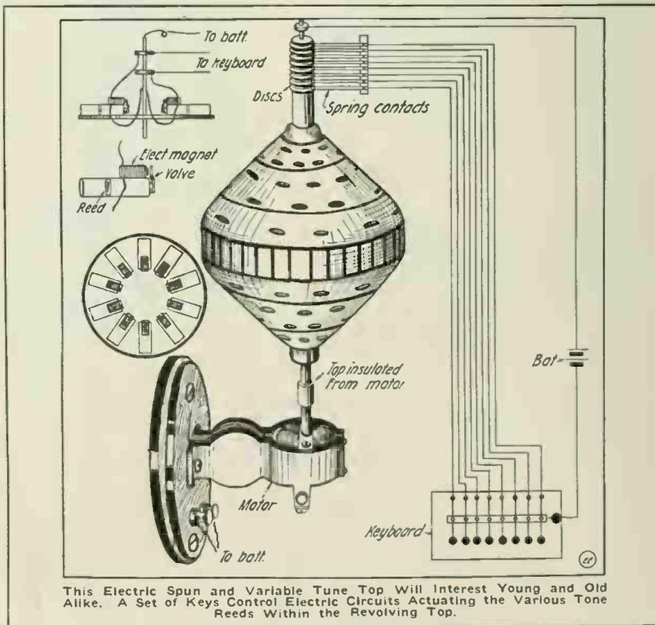
This Electric Spun and Variable Tune Top Will Interest Young and Old Alike. A Set of Keys Control Electric Circuits Actuating the Various Tone Reeds Within the Revolving Top.
