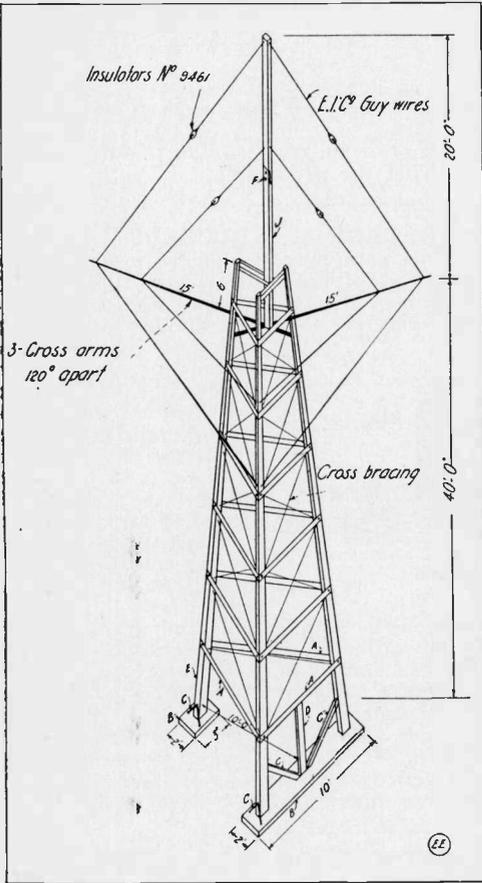
together till tight. This is much cheaper and offers less wind resistance than boards. The boards A. A. Fig. 1, are 1/2 inch thick and 3 inches wide and are secured by means of screws of suitable size. All the main joints such as at F. are secured by three iron bolts and nuts.
