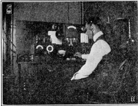
in back of the motor is used as a loading coil for long waves. The motor speed is 3600 R. P. M. and the 18 point disc gives a note similar to that of "N.A.R." A hot-wire ammeter shows in the middle of the picture with a S. P. T. T. switch which connects the aerial either to the ammeter,
