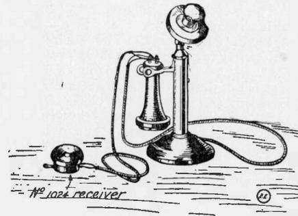
at hand, in the "Electro" No. 1024, 40 cent telephone watch-case receiver, which may be readily connected on multiple to any standard telephone receiver; on any line, as shown in the sketch. A 3-foot double conductor cord, No. 4003 is worth but 15 cents. Many thousands of these auxiliary telephone receivers are
