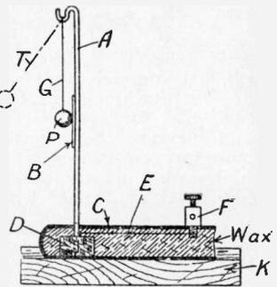
It is does not work properly try standing it on a piece of glass to insulate it from the ground.
