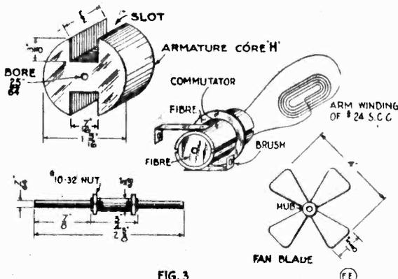
winding terminals are soldered to the segments. The shaft of steel, iron or brass is detailed at Fig. 3, and needs no special description. The armature laminations, forming the core "H," are locked between two No. 10-32 nuts threaded on the shaft. The commutator core is drilled out to make a driving fit on the shaft.
