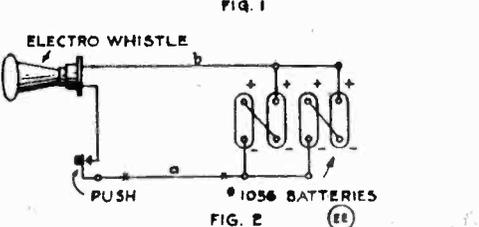
longest life. These individual batteries consist of 3 cells each, and therefore give  $4\frac{1}{2}$  volts a piece or 9 volts for the two in series. The lamp cord may be secured to the bicycle frame and handle bar, with ordinary friction tape or string, and a very neat job can be arranged by passing the wire thru the tubular construction of the bicycle frame itself.
