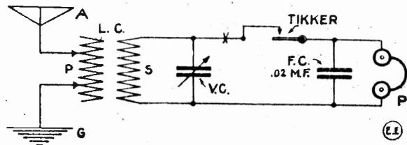
receiving sets, utilizes two crossed gold wires of about No. 28 B. & S. gauge, which make and break the signals at the point shown on the diagram here given. This wire is used, owing to the peculiar arcing characteristics of gold. With this hook-up or receiving arrangement, the tones of the received signals are thus controlled by the number of breaks per second made by the Interrupter or Tikker.
