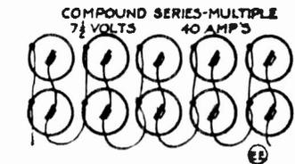
By connecting two such series files of cells on parallel or in multiple series, as indicated in the sketch; the voltage remains as previously, but the ampere or current capacity is of course doubled. As seen the carbon terminals of each series file are connected together; likewise the zinc terminals. The compound series-multiple hook-up shown, is sometimes utilized. As will be evident there may be any number of series files connected on multiple-series or parallel, and
