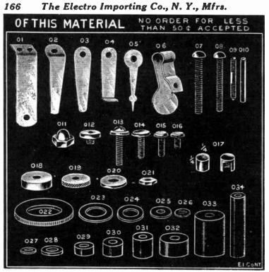
No. 01 Brass Leaf Detector Spring. No. 01 Brass Leat Detector Spring. 278 in. long, ½ in. wide, 1/64 in. thick. Three holes pass 8-32 screw. Price each, \$0.10. No. 02. Stiff Brass Spring. 2% in. long. 2%
