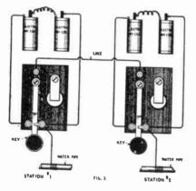
Diagram Shewing Connections for Intercommunication.
