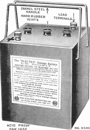
The 40 A.H. size has 3 plates in each cell; the 60 A.H. size has 5 plates in each cell; the 80 A.H. size has 7 plates in each cell; the 100 A.H. size has 9 plates in each cell. The cells are of hard rubber, NOT glass.
