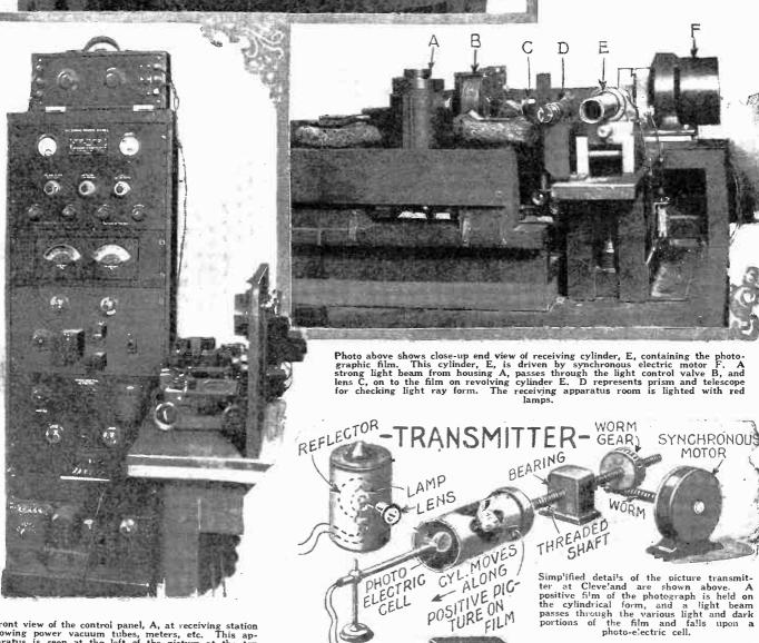
Front view of the control panel, A, at receiving station showing power vacuum tubes, meters, etc. This apparatus is seen at the left of the picture at the top of page, the operator behind the center panel board giving the signal to Cleveland when the apparatus has had a new film placed on it, and everything is ready for reception of the picture.
