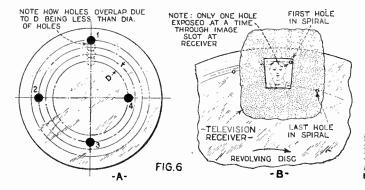
The proper neon tube to use behind the perforated receiving disc in the television apparatus, is one large enough to cover the size of the image. As shown at the right several small tubes may be utilized in an experimental apparatus, placing the tubes close together.
