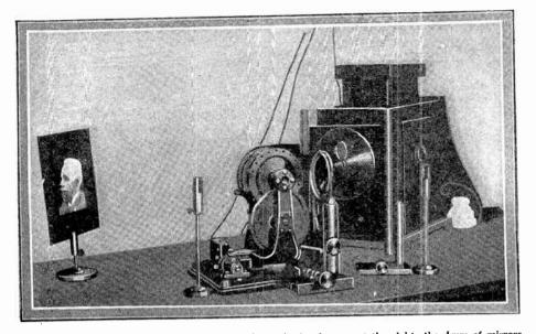
Fig. 61. This apparatus is diagrammed below; the projecting lantern at the right; the drum of mirrors, center; and the adjusting stands for diaphragm and fixed mirrors in front. At the left a continuous image appears on the screen, although only 1/25,000 of it is actually projected at any instant.
