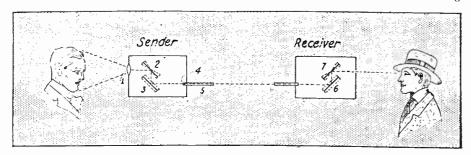
Fig. 27.—Depicts the Sinding-Larsen Telephot. Two mirrors vibrating at different frequencies cut up the light rays. These light rays are past through a metallic tube having strong reflecting inner surfaces. At the receiver, the light rays are past through a similar system as the sender and the picture is thus reconstructed.
