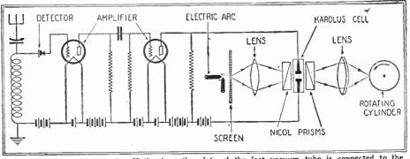
e receiver circuit. Notice how the plate of the last vacuum tube is connected to the the Karolus-cell. The variations in the plate current cause a corresponding change in the transparency of the cell, by the phenomenon of polarization. Fig. 99. The condenser of
