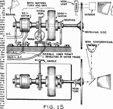
allows the operator who starts the machine up to look in the mirror and view the disk image created by the whirling holes and neon tubes. He watches this image and neon tubes. He watches this image and turns the synchronizing worm gear handle slowly, until the image is framed
