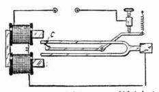
Fig. 39. The tuning fork interrupter which is kept vibrating with an electro magnet.
