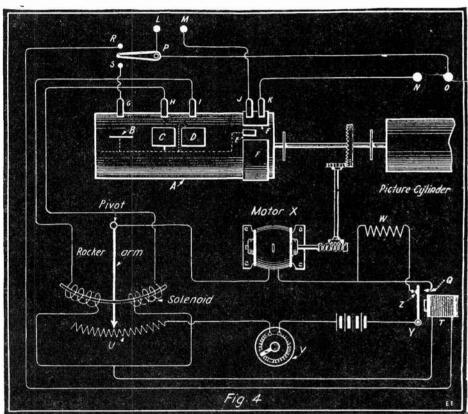
Layout for improved electrical synchronizer to be used for operating telephotographic transmitting and receiving apparatus here described.
