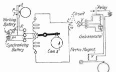
Fig. 26. Diagram of the transmitting end of the Belin apparatus for transmitting pictures by telegraph or telephone line.
