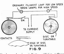
Simple synchronism indicator utilizing ordinary filament lamps for low speeds, and neon lamps for higher speeds. Whenever the transmitting and receiving discs are rotating in step or in synchronism, both lamps will light.
