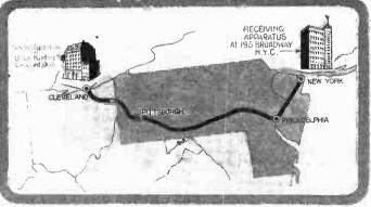
The circuit over which the picture currents traveled between Cleveland and New York City is shown in the official map above. Vacuum tube amplifiers as shown in the diagram below, were used at certain points along the line to boost the picture currents and the vacuum tube found another role in supplying the necessary control currents for the synchronous motors.
