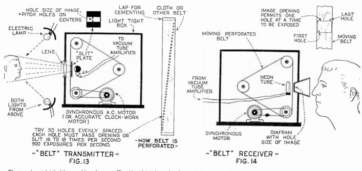
The experimental television machine shown at Fig. 13 and 14 above, has been tried out successfully by its inventor, Mr. L. J. Shramek. The perforated belt represents one way of causing the light ray to progressively traverse the image at the transmitter, and also to build up the image from the successive light pulses in the neon tube at the receiver.
