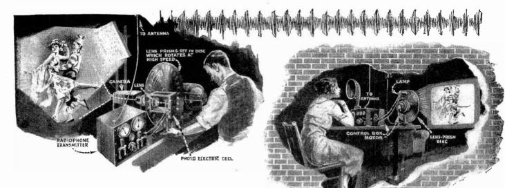
Fig. 34. This illustrates the Jenkins' method of sending moving pictures by radio. The main instrument in the machine is a disc revolving at high speed, upon which are mounted special lens prisms. A similar disc is used in the receiver which is comparatively simple and may be operated from an ordinary radio receiver and amplifier.
