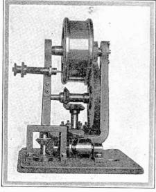
Fig. 66. This is a front view of the cylinder or drum of mirrors. It is turned by an electric motor, and at the same time swung from side to side by the gear at its base.
