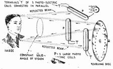
Fig. 95. How the extreme positions of the succeeding pencils of light exploring the object st the transmitter are enabled to pick up the whole intage. The solid angle of vision is made up of rapidly moving beams of light.
