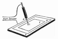
Fig. 39. This sketch illustrates how colored pictures may be sent by radio by means of special papers supporting some colors which are melted by the heat of a spark passing through
