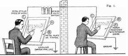
One of the first steps in electrical "picture transmission" is shown in the illustration here-with. The two operators move the metal pencils back and forth along the platens at approximately the same speed. Through electro-chemical action, the dots and dashes are reproduced on the paper at the receiver, whenever the transmitting operator's pencil touches the metal plate.
