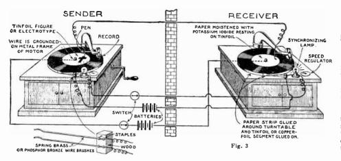
A pair of phonograph motors, or rather two complete machines, can usually be procured without much trouble nowadays since the advent of radio broadcasting. The diagram above shows how two disc phonographs can be utilized for transmitting and receiving a drawing or other image by electrochemical means.
