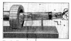
Fig. 83. Close-up view of the Dauvillier special vacuum tube used to reproduce image by virtue of cathode beam oscillated of controlled by the electro-static fields.
