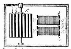
Fig. 40. The phonic drum used to synchronize the telehor.
