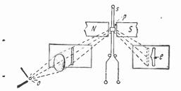
Fig. 38. The oscillograph arrangement which converts the variable current into picture elements at the receiving apparatus.
