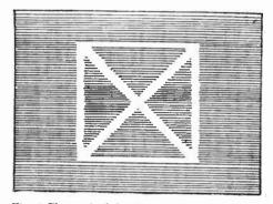
Fig. 4. The received drawing is a "negative" of the drawing on the transmitter drum, since the re-ceiver stylus is lifted off the drum when the trans-mitter reaches point after point on the drawing.
