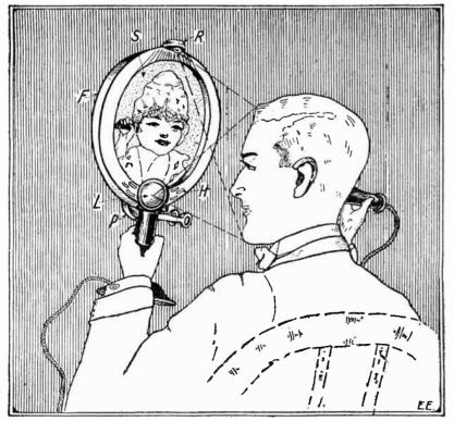
Fig. 21. What the future Telephot will look like in order to be practical. Light R throws light on speaker's face and is reflected into lens L. Instead of a mouthpiece, the holes H of the sensitive transmitter inside of frame F pick up the speech. The picture of the distant person appears on screen S.
