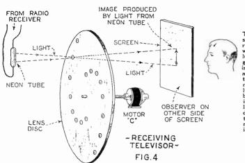
bright section of the subject's face which bright section of the subjects face which was analyzed by transmitter lens No. 15 at the particular instant and which caused the electrical impulse. If, for instance, the spot appears in the center of the field covered by the transmitter lenses, it will be indi-cated on the receiving screen by a spot of light placed in the center of the screen.
