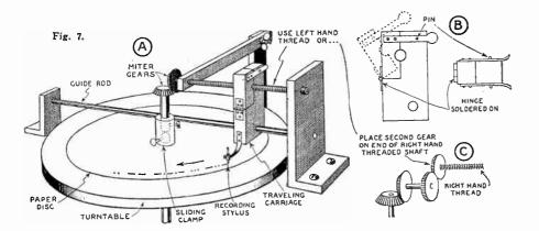
By means of the attachments shown above, and which can readily be fitted to any disc type phonograph, it is possible to transmit and reproduce a larger image than with the arrangement described and filus-trated previously, wherein the regular tone arm of the phonograph is used to traverse a recording pen across a small disc.
