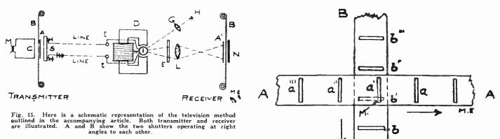
Fig. 16. Right. Here is a detailed view of the shutter arrangement. The arrows indicate the direction of movement and the small letters a, and b, represent the slots in the endless bands.
