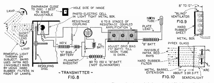
Here the subject is illuminated by powerful lights, the reflected light rays acting on a photo-electric cell. Figs. 9 and 10 show method of arranging invisible infra-ray illuminants for use at the television transmitter,
