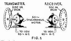
The simplest means of operating the transmitting and receiving disc of a television outfit is to drive each dlsc by sixty cycle synchronous motors, as shown above.
