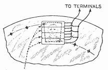
SUFFICIENT NEON TUBES TO COVER IMAGE OPENING: BEST TO USE ONE NEON TUBE LARGE ENOUGH. ----
