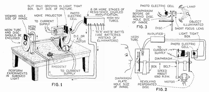
The simplest experimental television machine which will help to demonstrate the principles of transmitting the living image over a wire, is shown in the picture at Fig. 1 above.
