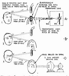
Fig. 90. Successive light beams issuing from the holes in the whirling disk at the transmitter sweep over the object; their movement is exaggerated here. A lens is also used in front of the disc.
