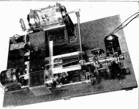
Photos in this article by courtesy of the Radio Corporation of America. Above is shown the transmitting apparatus for the hroadcasting of photographs, maps, etc., by means of radio
