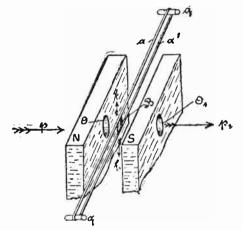
Fig. 5. The light relay described in this article.
