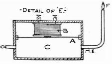
Fig. 13. Here is the light changing device indicated by a box in the previous figure. When diaphragm A moves, flame flickers.
