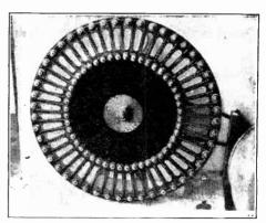
Fig. 37. Front view of the receiver disc showing how the lens prisms are mounted.
