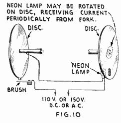
Simple synchronizing scheme which will cause the neon lamp to be lighted each time the brush and segment or tooth on the transmitting disc makes contact, the light pulsations being visible only when the slot in the receiving disc is opposite the neon lamp.
