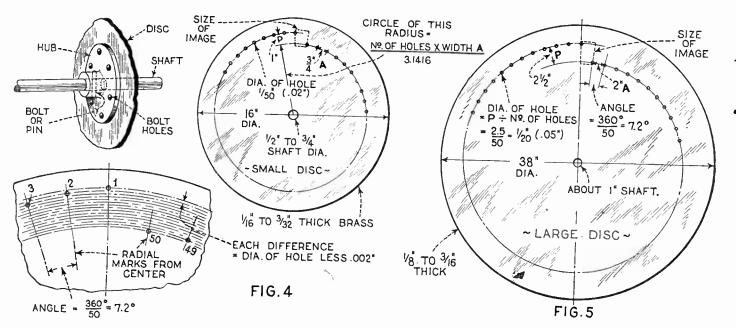
The method of laying out the holes in the disc used in the Bell television The holes in the disc used in the Bell television apparatus are laid out on a spiral in the manner illustrated.
