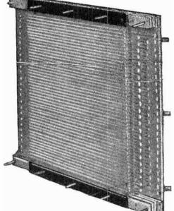
Fig. 92. The large 24 by 36-inch glass tube screen on which the television image was reproduced at the demonstration in the Bell Telephone Labora-tories in New York City.
