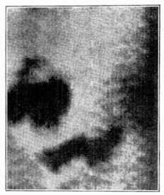
A high magnification of a small area on one of the received photographs show a smoothness of texture hitherto unattainable with commercial processes of photo-transmission. The high-lights and shadows are brought out in perfect detail, the artistic effect suffering not at all.
