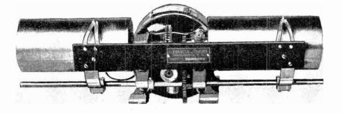
Another form of the device employs a small motor for turning over the cylinders which carry the "pens" and the chemically treated paper.
