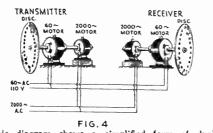
This diagram shows a simplified form motor drive for television disc. of dual
