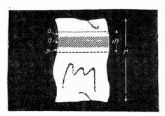
Fig. 38. A developed view of the cylinder showing the marks used for synchronizing the receiving apparatus
