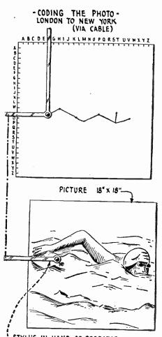
STYLUS IN HAND OF OPERATOR WHILE PICTURE IS IN PROCESS OF DECODING. Fig. 11. Showing the method in which the picture was coded. A pantograph arrangement with a hori-zontal and vertical scale together with a code representing the intensity of tint of the various areas form the basis of the Leishman telegraph picture process.
