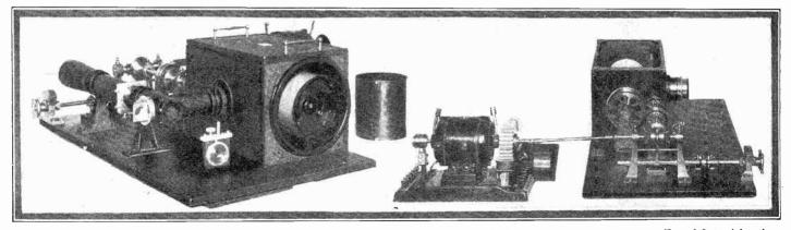
Fig. 102. The Telefunken-Karolus receiver system showing at the right a cylinder on which the unexposed negative film is mounted. One Karolus-cell may be seen in position in the center of the optical device and one standing in front of the receiving cylinder case.
