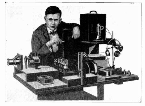
Fig. 44. Another view of the telebor machine with its inventor, Mr. Dionys Mihały. The numbers refer to I tuning fork interrupter, 2 selenium cell, 3 mirror of «scillograph, 4 lenses, 5 phonic drum, 6 armature, 7 electromagnet of phonic drum, 8 diaphragm, 9 oscillograph.
