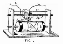
Fig. 7. This modified form of "te'ephotographic" transmitter operates with the drawing to be trans-mitter formed in relief on the paper. The trans-mitter circuit is closed when the stylus is lifted by the raised portions of the drawing
