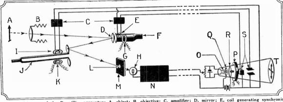
Fig. 84. Diagram of the Dauvillier apparatus: A, object; B, objective; C, amplifier; D, mirror; E, coil generating synchronous currents; G, 800 cycle tuning fork; G, exciting current; H, photo-electric cell; I, coil generating synchronous currents; J, 10 cycle tuning fork; K, exciting current; L, hole determining the point of the image; M, optical screen; N, amplifier; O, filament; P, concentrating coil; Q, grid; R, plate; S, condensers producing electrostatic fields; T, fluorescent screen.
