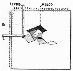
Fig. 12. At the receiving end the various letter combinations are potted by the operator and filled in by the artist.
