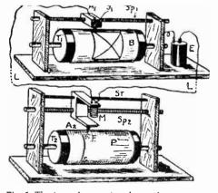
Fig. 5. The type of apparatus shown above operates by a positive action of the receiving stylus, the latter making a mark on the receiver drum when the transmitter current is interrupted by lines of the drawing.
