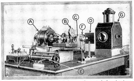
Fig. 70. The Belin transmitter: A is the 500-cycle alternator used as a motor for the moving mirrors; B, microphone of low-frequency mirror; C, "transparency" (photo film) support; D, diaphragm; E, alternator rheostat; F, objective lens; G, arc lamp.
