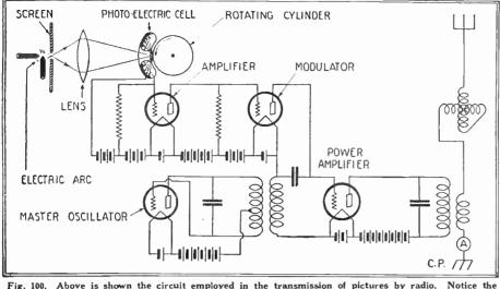
Fig. 100. Above is shown the circuit employed in the transmission of pictures by radio. peculiar construction of the photoelectric cell and its connections.
