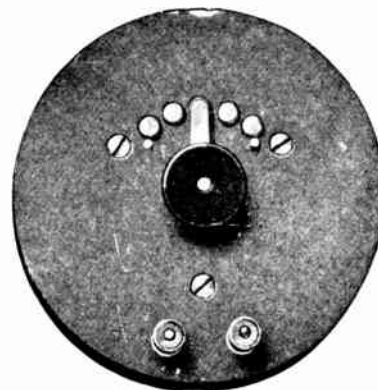
Signal Loading Coil R-26
