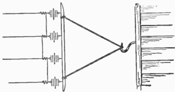
FIG. 22.—Ends of Antenna Wires Insulated and Bonded.
