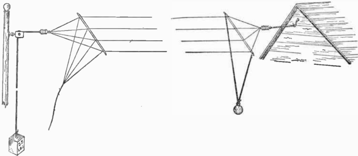
FIG. 19.—A Good Type of Aerial for Most Ordinary Conditions.
