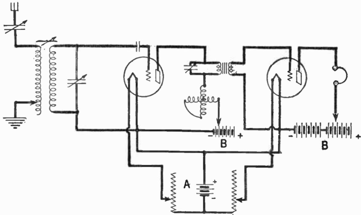
FIG. 15.—Diagram of Receiver Set, with One-Stage Amplifier Using Two Separate Blocks of B Battery.
