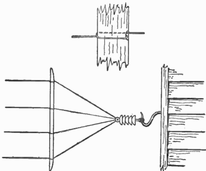
FIG. 21.—Ends of Antenna Wires Led Together.
