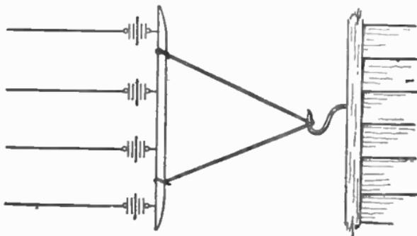
FIG. 23.—Ends of Antenna Wires Left Free.
