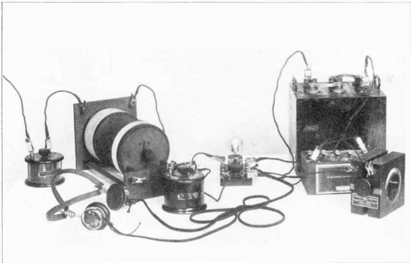
FIG. 13.—Receiver Set, Instruments Assembled by Amateur.
