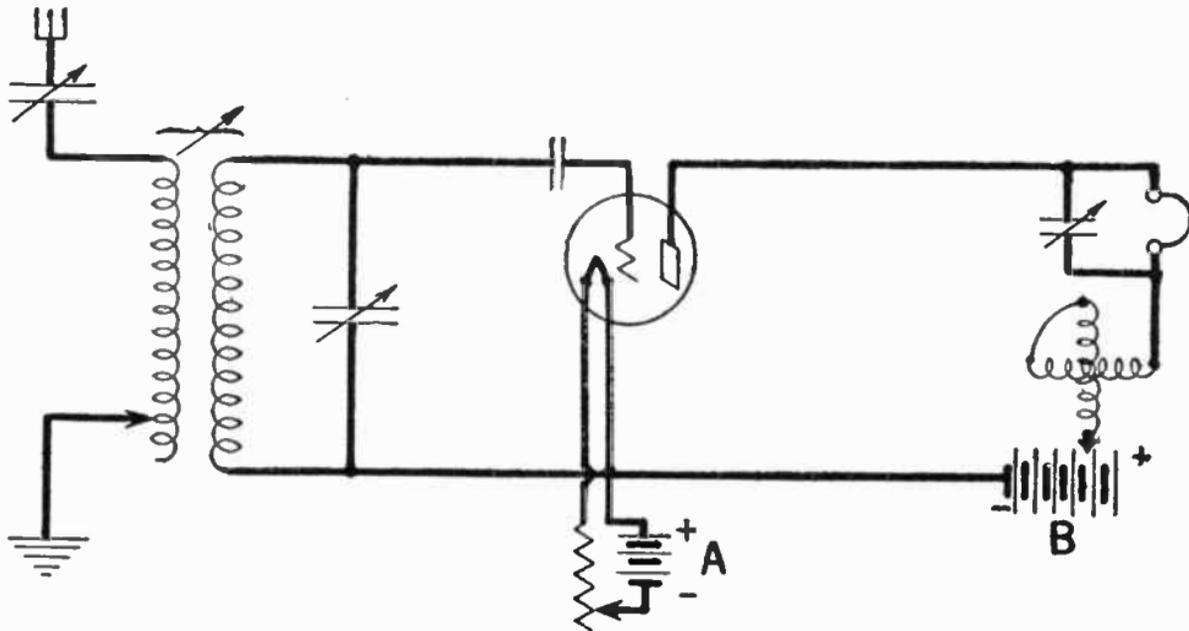
FIG. 11.—Diagram of Regenerative Receiver, with Variometer in Wing Circuit.
