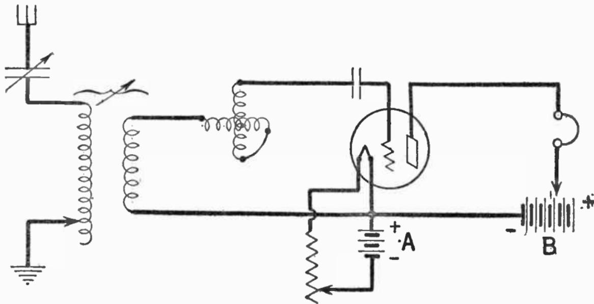
FIG. 8.—Diagram of Vacuum Tube Set with Series Condenser in Primary Circuit, and Variometer in Secondary Circuit.
