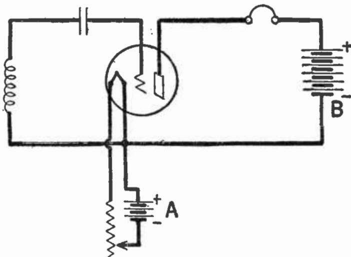
FIG. 35.—Diagram Showing Operation of Vacuum Tube.
