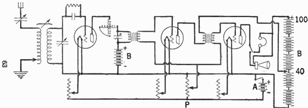
FIG. 18.—Diagram of Receiver with Two-Stage Amplifier, Potentiometer Wired So As to Effect a Negative Potential on the Grid, and Optional Phones or Loud Speaker.
