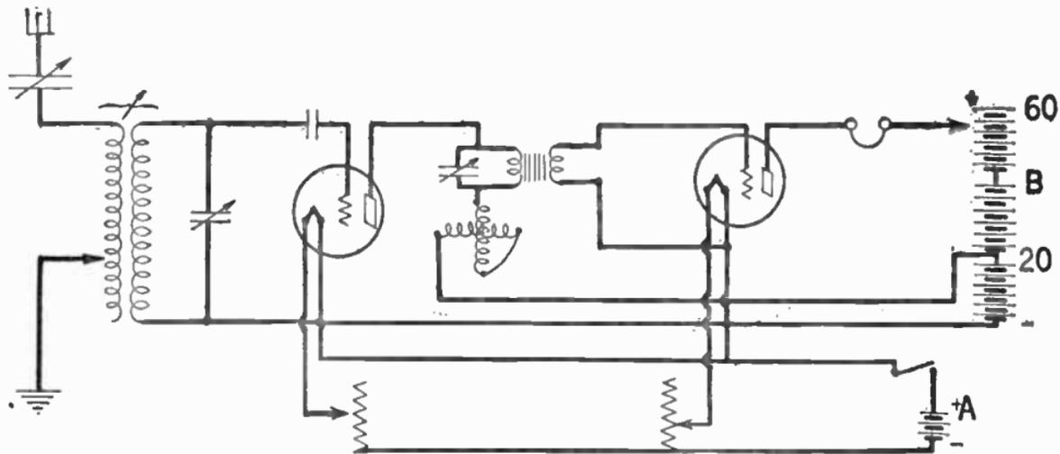
FIG. 16.—Diagram of Receiver Set, with One-Stage Amplifier Using Common B Battery on both Detector and Amplifier.
