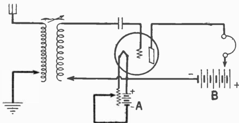
FIG. 7.—Diagram of Simple Vacuum Tube Receiver Set.
