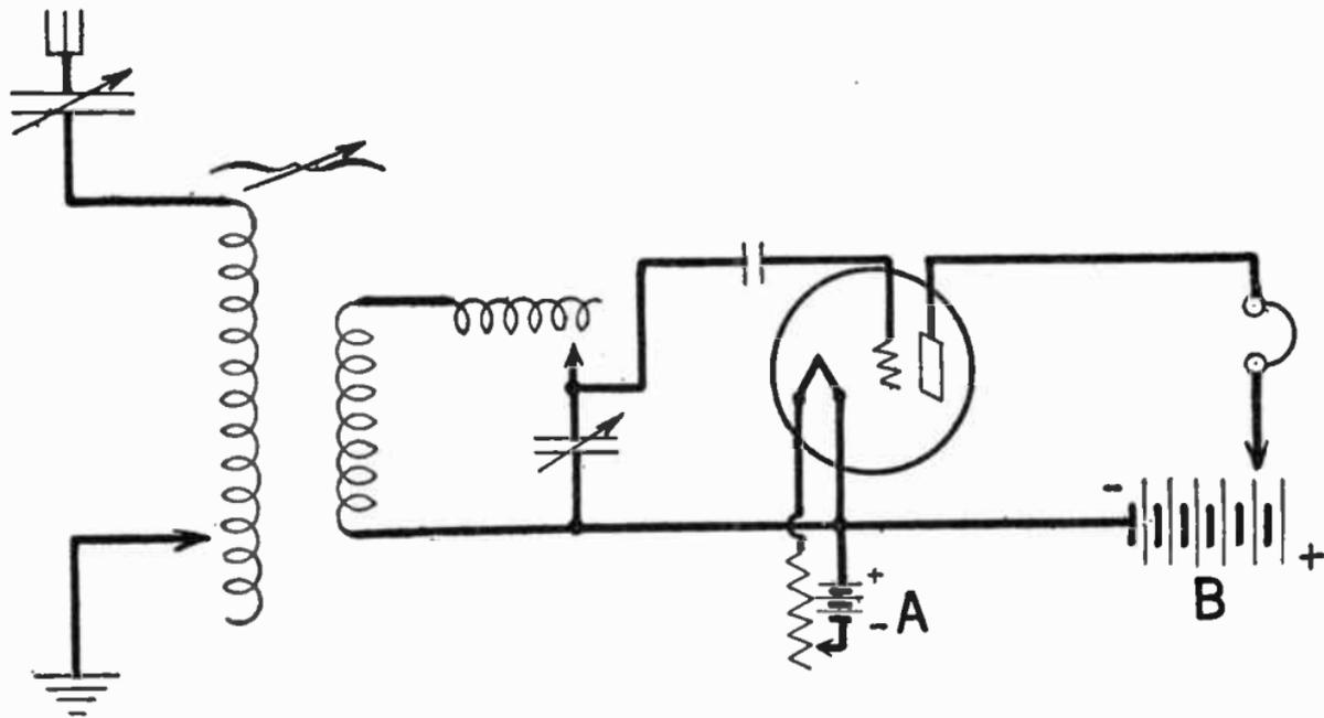
FIG. 9.—Diagram of Vacuum Tube Receiver Set, with Secondary Load, and Secondary Condenser in Shunt.
