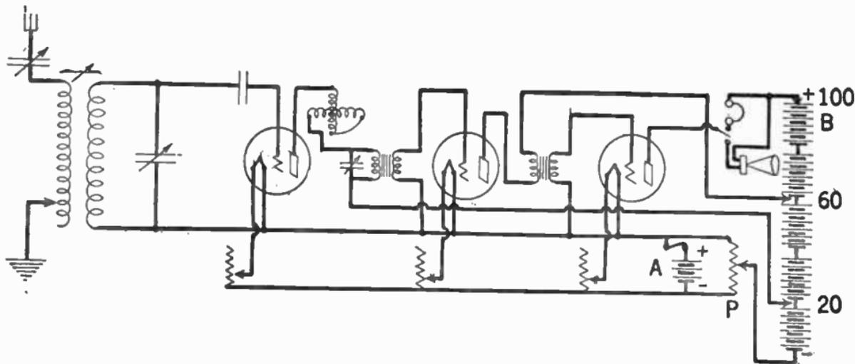
FIG. 17.—Diagram of Receiver with Two-Stage Amplifier, with Common B Battery, and Including Potentiometer and Optional Phones or Loud Speaker.
