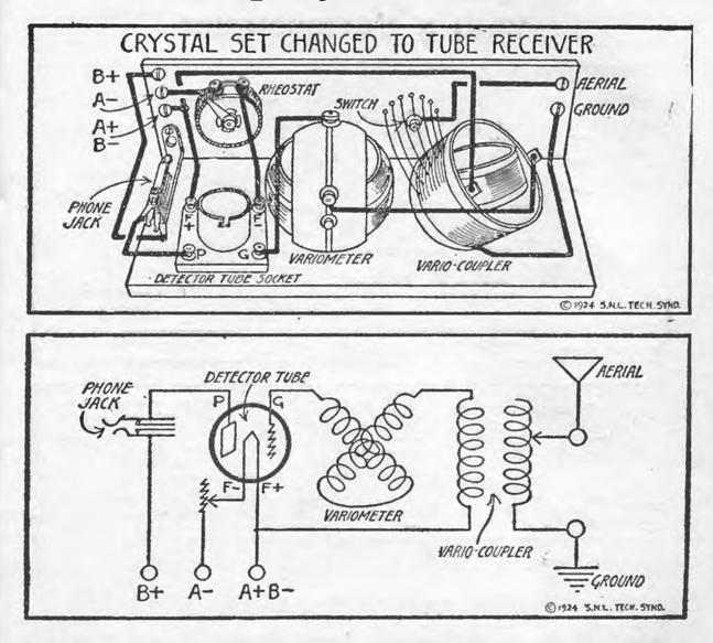
This is a circuit showing how the same apparatus can be used to change your crystal set into a vacuum tube receiver. This is possible without changing any of the apparatus on the front panel, or moving any of the instruments.
