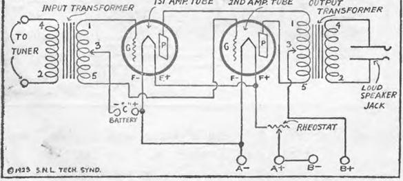
This is an amplifier for use in conjunction with any type of receiving set. It can be attached to a regular detector and two-stage receiver for the purpose of amplifying the signals for loud speaker reception without adding distortion to the output.
