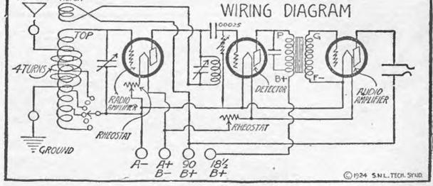
The Superdyne receiver shown above is an entirely new and efficient circuit using a stage of radio, detector, and a stage of audio frequency. It may be constructed with two stages of audio frequency if you desire.
