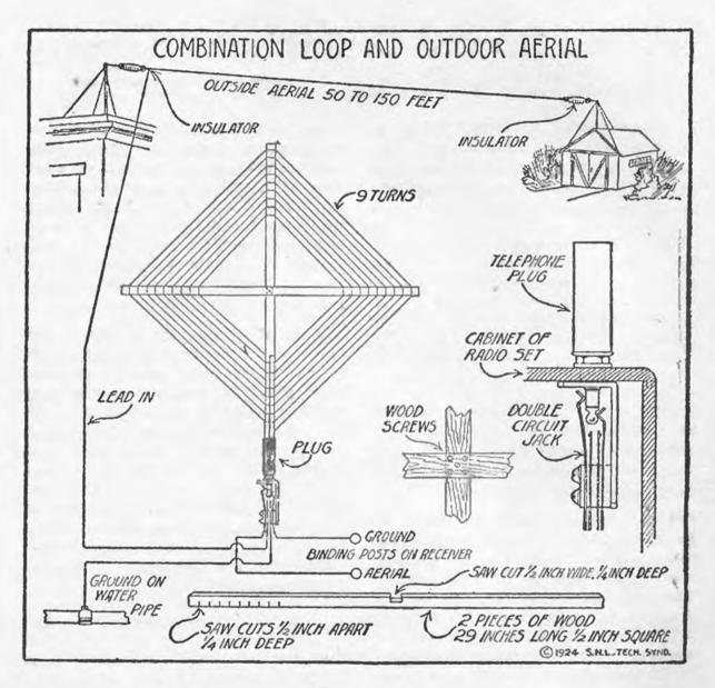
The loop is constructed on a wooden frame constructed of two cross pieces each one half inch square and twenty-nine inches long. Cut nine slots in each end of the cross pieces as shown in the illustration. Make these cuts with a hack saw approximately one quarter of an inch deep and one half inch apart.
