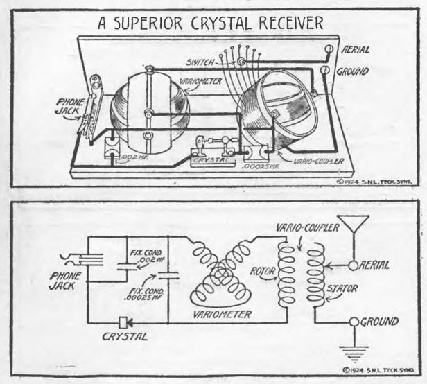
This is a crystal receiver constructed with a variometer and a variocoupler. This receiver is more selective than the crystal circuit shown on the preceding page, due to the fact that a two circuit method of tuning is used.
