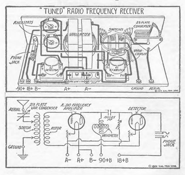
This is a circuit somewhat similar to the Tuned Impedance receiver shown on the opposite page. In place of the honeycomb coil and condenser a variometer is used to tune the circuit between the radio frequency tube and the detector.
