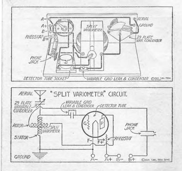
This is a very compact and easily constructed receiver made with a variometer. The circuit derives its name from the fact that the variometer is divided into two windings, similar to the winding of a variocoupler.
