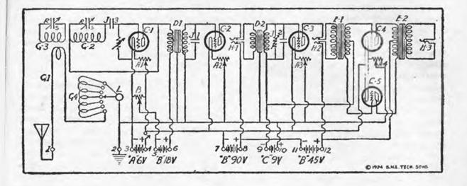
The single tube four circuit tuner can be converted into the five tube set shown on the opposite page by the addition of two stages of audio frequency and a push pull amplifier. The tuning unit remains the same.
