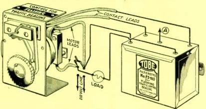
Fig. 2. Single Circuit Mechanical Contactor Used for Controlling Flashing Traffic Beacon.
