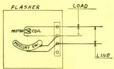
Fig. 4. Diagram of Mercury Switch Flasher in which the Switch Breaks both the Load and Motor Circuits.
