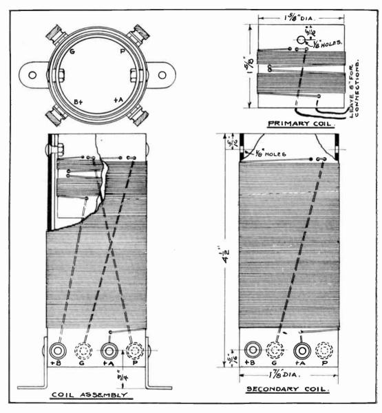
Fig. No. 27-Detailed Drawing Showing How to Construct Coil No. 2 for Duston Special
