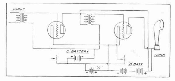
Fig. No. 12-Proper Way to Connect "C" Battery in Amplifier Circuit
