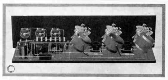
Plate No. 14-Rear View of Neutrodyne Type Receiver-Front View Is the Same as Shown in Plate No. 12
