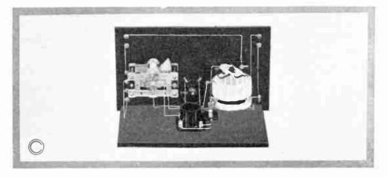
Plate No. 6-Rear View Low Loss One Bulb Set
