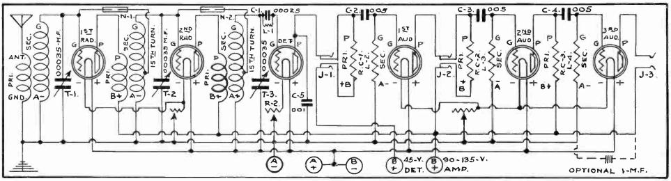
Fig. No. 25-Hook-up Showing Three Stages Resistance Coupled
