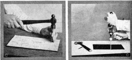
Plate No. 3-Marking panel from Template
