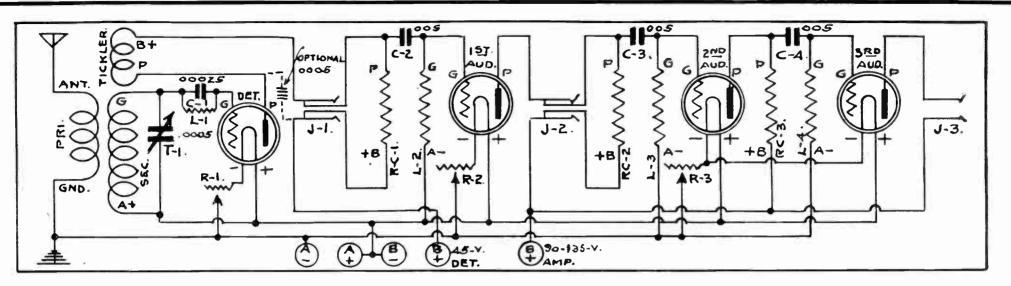
Fig. No. 19-Hook-up Three Circuit Set Using Three Stages Resistance Coupled Amplification
