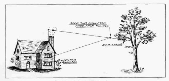
Fig. No. 4-Single Wire "V" Type Antenna
