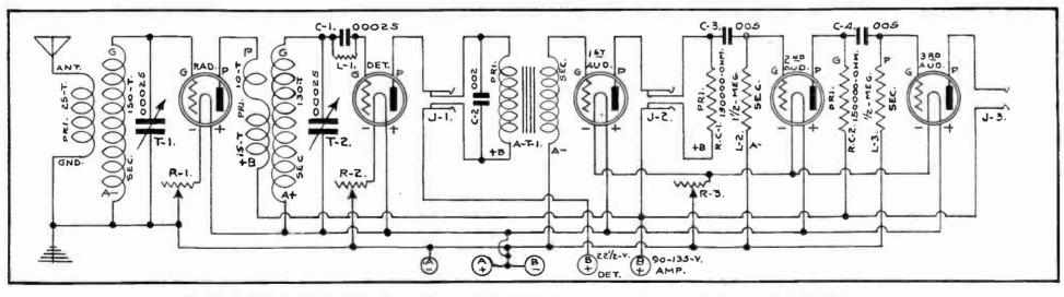
Fig. No. 29-Hook-up Showing Duston Special Using One Stage transformer Coupled and Two Stages Resistance Coupled Amplification
