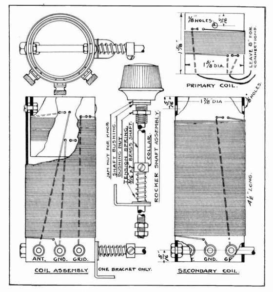
Fig. No. 28-Detailed Drawing of Coil No. 1 for Duston Special
