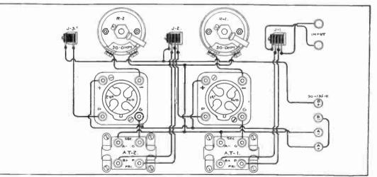
Fig. No. 16-Drawing of Two Stage Audio-Frequency Amplifying Unit
