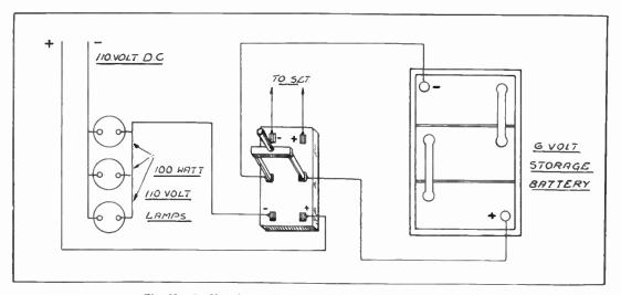
Fig. No. 7-Charging "A" Battery from Direct Current Line
