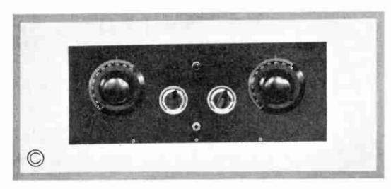
Plate No. 16-Front View of Two Bulb Reflex Set
