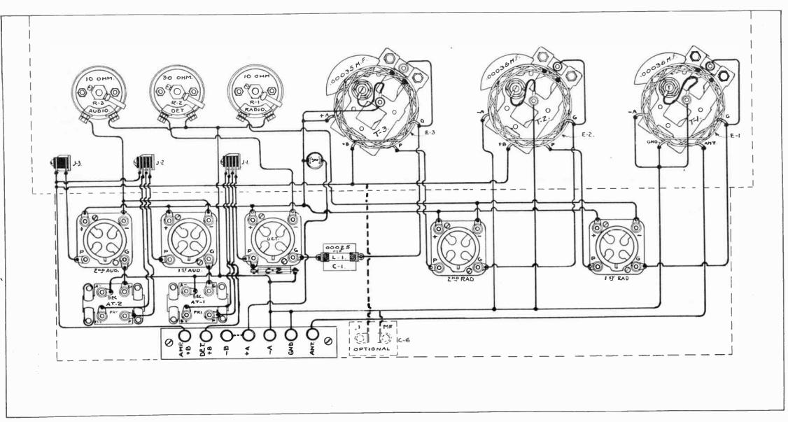
Fig. No. 20-Drawing of Low Loss Radio Frequency Set Using Transformer Coupled Amplification
