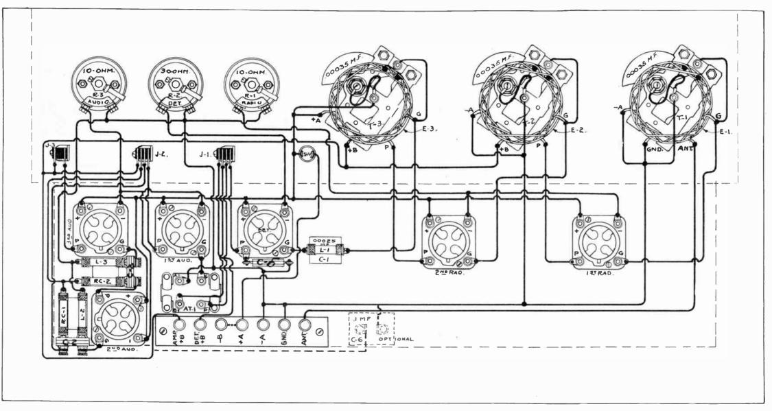
Fig. No. 21-Drawing of Low Loss Set Using One Stage Transformer Coupled and Two Stages of Resistance Coupled Amplification
