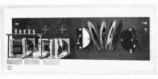
Plate No. 5-Set Assembled Ready to Wire
