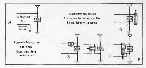
Fig. No. 5-Proper Ways to Install Lightning Arrestor
