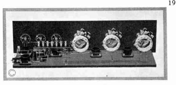
Plate No. 13-Rear View of Set Showing One Stage Transformer and Two Stages Resistance Coupled Amplification
