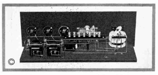
Plate No. 11-Rear View Transformer Coupled Low Loss Three Circuit Receiver
