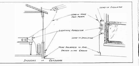
Fig. No. 1-Installation of Lightning Arrestor
