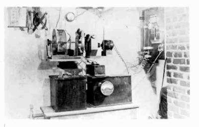
Typical amateur transmitter of the rotary synchronous spark gap era in 1919. The rig was built and operated by Lester Spangenberg in New Jersey.
