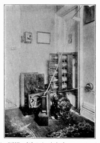
Transmitter, Station "2PM", which producted the first transcontinental signals in 1916. Note the synchronous rotary gap mounted between motor and generator, large plated Leyden jar condensers and 1 K.W. United Wireless coffin transformer. This was the very latest equipment at the time.
