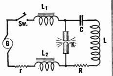
When the discharge is complete, the cycle of charge and discharge repeats itself with a frequency deter-mined by the constants of the inductance L and the capacity C. By carefully choosing these values, large amounts of high-frequency energy can be obtained. large am obtained.
