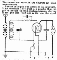
strength will be decreased. For the ordinary 201-A type tube, a gric leak of about four megohms resistance will give the best results. If a soft detector tube is used, a somewhat lower resistance leak is generally required; about one half to two megohms being about right.
