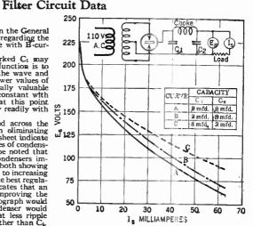
The curves shown are for a single section filter using the Raytheon tube as a rectifier. A multi-section filter would, bowever, give the same type of curves.
