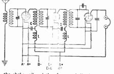
the choke coil and therefore good filtering action will be obtained. If the choke coil's impedance at 500 kilocycles is to be 1000 imes greater than the impedance of the condenset hen it must be 12,000 ohms. The inductance of a choke coil with an impedance of 12,000 ohms at 500 kilocycles is 38 millihenrys. Most raduo-frequency choke coils have an inductance of much more than this.
