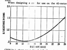
(7500-kc.) short-wave band (all these tests were made at this frequency), it is well to (1.) use about No. 12 to 14 wire; (2.) use a coil form if desired; (3.) use any good dope as a binder; (4.) use any reasonable amount of shielding where advanta-geous; (5.) keep the form factor (diameter divided by length) around 1 to 2.5. These data are taken from the February, 1927, These data are taken from the February, 1927, issue of the General Radio Experimenter.
