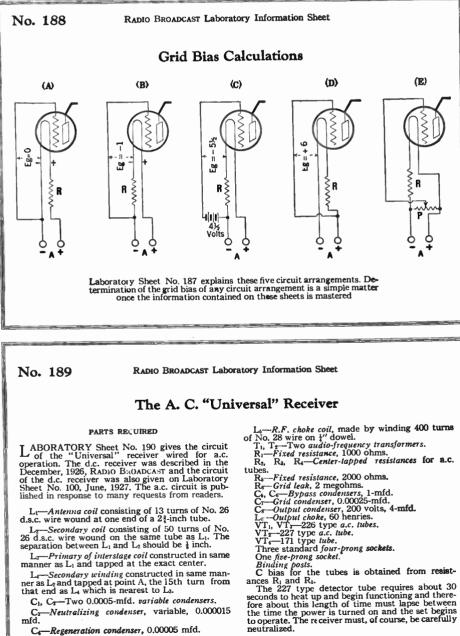
$L_2$ —Secondary coil consisting of 50 turns of No. 26 d.s.c. wire wound on the same tube as L<sub>1</sub>. The separation between L<sub>1</sub> and L<sub>2</sub> should be  $\frac{1}{2}$  inch.
