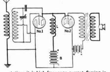
stations it is high frequency current flowing in the antenna that radiates energy in the form of electromagnetic waves (in this case, radio waves). Tube No. I is an oscillator in the waves). Tube diagram shown.
