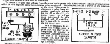
The tone quality of any set operating on a B-eliminator may generally be improved by adding capac-ity across the plus maximum and minus binding posts. Anywhere from 4 to 8 mfd. of additional capacity may be connected externally.
