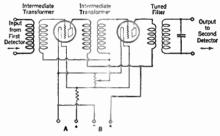
Regeneration in the intermediate-frequency ampli-fier will considerably improve the selectivity and sensitivity by sharpening the resonance curves of the transformers. The common method of connecting together in-termediate-frequency amplifiers is illustrated in the diagram, in which potentiometer control of regeneration is used.
