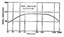
cation is increased. Large hypass condensers across the output of the power unit will frequently be necessary in order to prevent the occurrence of "motor-boating." The frequency characteristic of the complete amplifier is shown by the accompany-ing curve.
