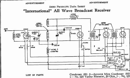
1—Aero Base Unit No. 8. 1—Aero Coil Kit LWT -10. 2—Aero C-60 R. F. Chokes. 1—Aero C-65 R. F. Choke. 2—Aero AE-770 Audio Frequency Transformers. 1—Aero Special Amsco Condenser. 00014. 1. -Amsco S. L. T. .00025 Condenser. 1— Aerovox Mica Condenser .00015. 1—Aerovox Mica
