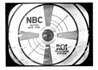
Figure 44—Excessive Auto Ignition Interference
