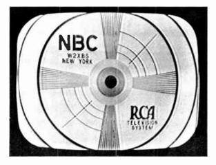
Figure 56—Transients in Test Pattern
