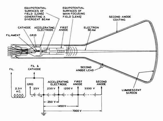
Figure 19—The Kinescope and Voltage Supply System
