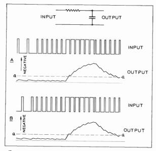
Figure 13—Vertical Pulse Selecting Circuit and Wave-forms
