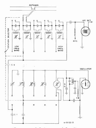
Figure 5—R.F. Input and Oscillator
