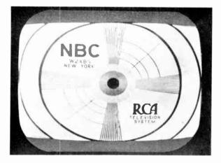
Figure 37—Vertical Height Control Incorrectly Set
