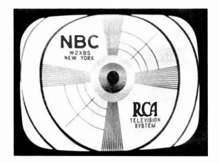
Figure 41—Vertical Linearity Control Incorrectly Set
