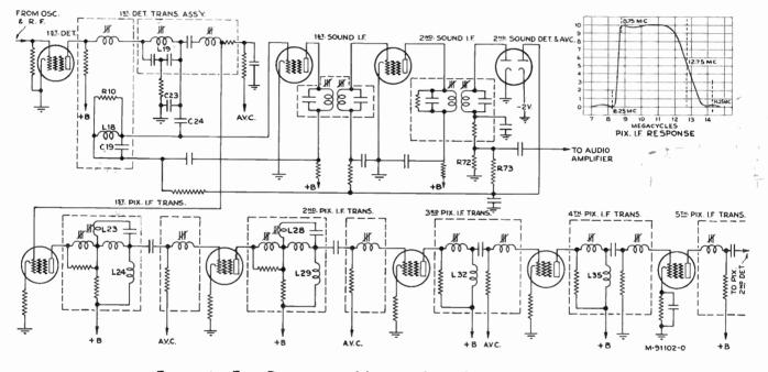
Figure 6—First Detector and Intermediate Frequency Amplifiers
