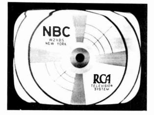
Figure 52—Unstable—"Tear-Out"— Horizontal Synchronization
