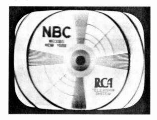
Figure 58—Loss of High Video Frequencies
