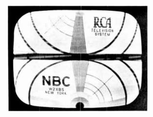
Figure 28—Vertical Hold Control Incorrectly Set
