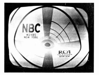
Figure 54—Excessive Ripple in Vertical Deflection
