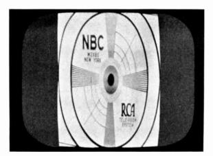
Figure 35—Horizontal Width Control Incorrectly Set
