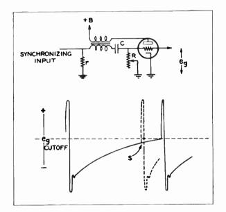
Figure 15—Blocking Oscillator and Wave-form
