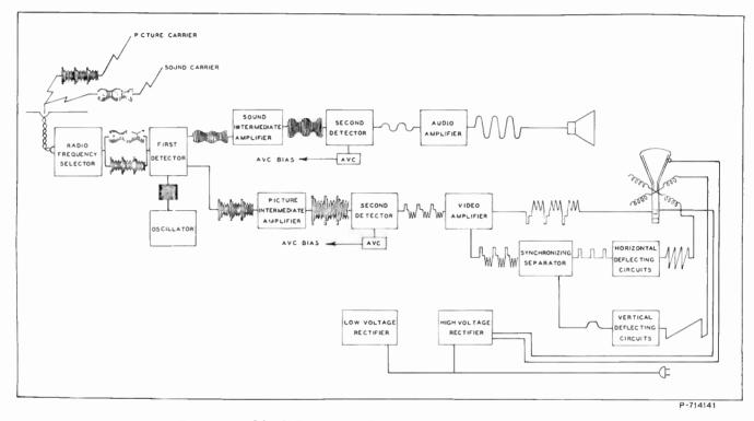
Figure 4—Block Diagram of a Typical Television Receiver
