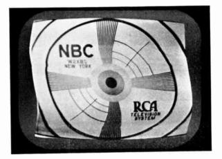
Figure 47—Excessive Ripple in Horizontal Deflection
