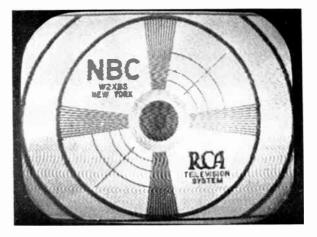
Figure 45—Excessive Diathermy Interference
