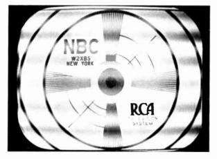
Figure 33—Sound Modulation in Picture
