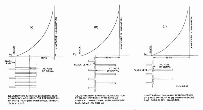
Figure 8—Operation of D.C. Restorer or Automatic Brightness Control
