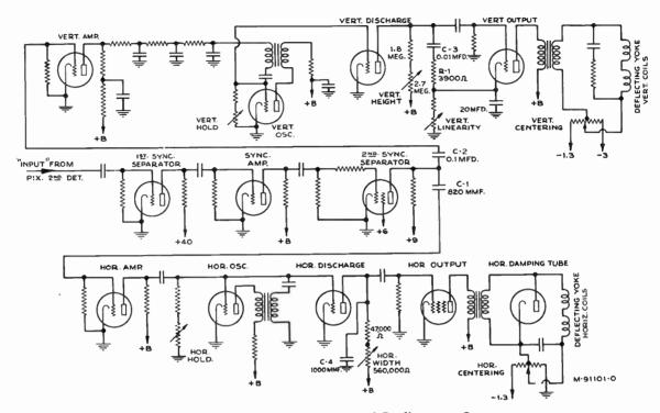
Figure 10—Synchronizing and Deflecting Circuits
