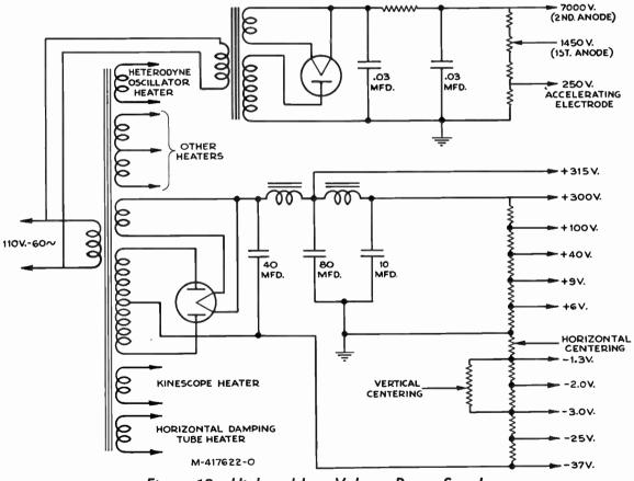
Figure 18—High and Low Voltage Power Supply
