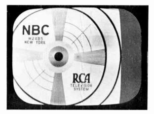
Figure 36—Horizontal Centering Control Incorrectly Set
