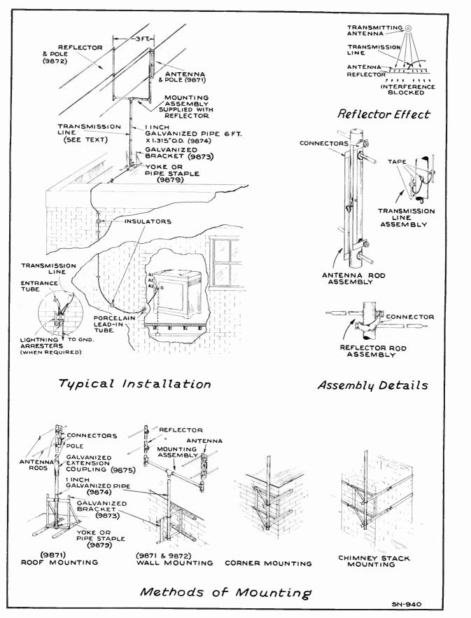
Figure 25—Typical Installation Details of RCA Double Dipole—Reflector Antennas
