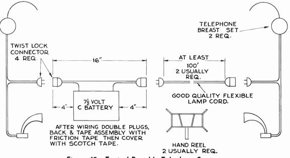
Figure 48—Typical Portable Telephone System
