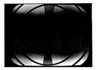
Figure 50—Excessive Ripple in Video Amplifier
