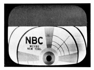
Figure 38—Vertical Centering Control Incorrectly Set
