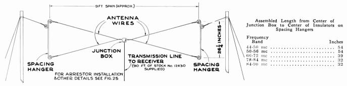
Figure 20—Typical Installation of RCA Double "V" Television Antenna
