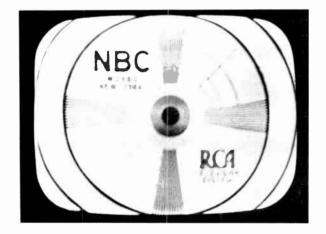
Figure 29—Focus Control Incorrectly Set
