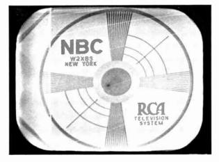
Figure 60—Effect of Damping Tube Failure
