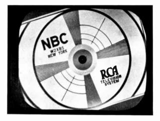
Figure 34—Picture Incorrectly Oriented
