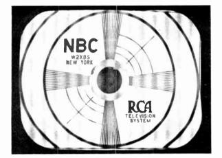
Figure 49—A 250 K.C. Sine Wave Signal with Test Pattern
