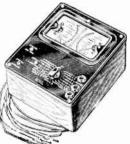
The Triplett Model 1200 is an extremely simple compact instrument, with both A.C. and D.C. movements. accurate within 2%. Ranges are: DC volts, 0-10, 0-100, 0-250, 0-500 and 0-1000; 0-1. 0-10 and 0-100 milliamperes; 0.1500, 0.1, 500.000 and 0-13 million ohms. AC scale is calibrated 0-10, 0-100, 0.250, 0.500 and 0-1000 volts. Voltage and resistance scales
