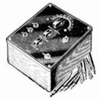
supply power for type 30 tubes. Coils, batteries, jacks, etc. in-dividually shielded. Used to determine frequency alignment, furnish the signal for aligning all types of broadcast receivers, and anywhere signal generator of constant amplitude is required. Complete with tubes and \$15.00 batteries. Net.....
