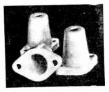
HIGH VOLTAGE SHAFT COUPLING. Isolantic insulated, rugged, and free from backlash, this coupling is made in three lengths, bored for 3/s''or 1/s'' shafts. Leakage path is 23/s'' less than over-all length. Type TX.3 (L=3/s'') Net 54.20
