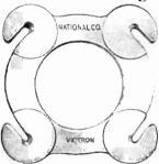
H. F. BUSHING. This small Steatite bushing has a variety of uses in transmitter construction, not only as a neat and efficient means of bringing H.F. leads through partitions, but as a support for coils, etc. Each pair of cones includes suitable metal fittings.
