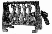
The REL Cat. No. 269 four-pole, double-throw rotary switch is suitable for a variety of purposes in radio and electrical installations. Its chief radio uses are: 1. Antenna change over switch where it is desired to disconnect filament and other auxiliary circuits. 2. Wave-length changing switch. 3. As a means of changing from CW to phone, or vice versa.
