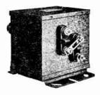
The same general construction has been employed in building the filament supply transformers. They are completely encased and sealed. The primary is arranged for 110 and 220 volts operation with the same method for changing as applied to the plate transformers. The secondary is adequately insulated for operation in connection with its associated apparatus even to the extent of using high voltage porcelain insulator at the terminals. No humid salt atmosphere will affect this transformer.
