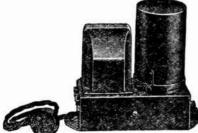
MIK 80 is designed for use solely with PAM 80. Taking advantage of the high amplification of PAM 80, it requires no tubes. It comes equipped with a cord and plug for attachment to PAM 80, through which it gets its power supply. It operates entirely from A.C., including button current supply. A 1,000-ohm variable volume control is provided, but not built into the unit for the sake of portability and convenience. Terminals for the microphone are tip jacks, color coded.
