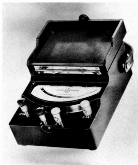
Fig. 28. Type AP-9 electrodynamic wattmeter
