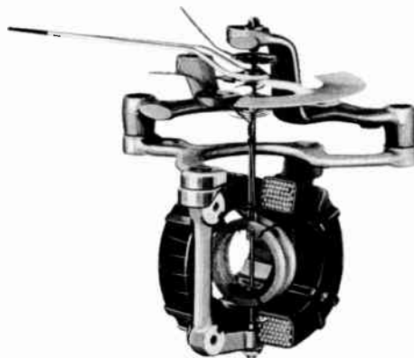
Fig. 9. Essential parts of a dynamometer instrument
