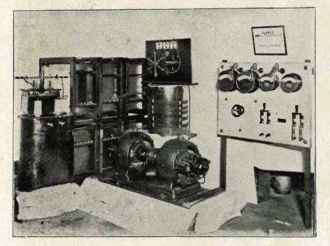
CLARK MOTOR GENERATOR SET WITH TRANSFORMERS, CONDENSERS AND OPERATING SWITCHBOARD
