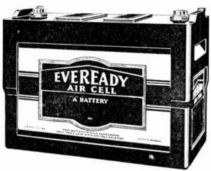
The Eveready Air Cell "A" Battery uses a liquid electrolyte, but is shipped div. In the dry state, it undergoes no depreciation. It can be activated for service at any time after manufacture and still deliver its full quota of ampere hours. It is activated for service by filling with water.
