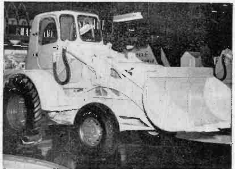
A hydraulically operated, diesel-driven scoop which can also work as a one-ton crane: it is especially suitable for loading and light excavation
