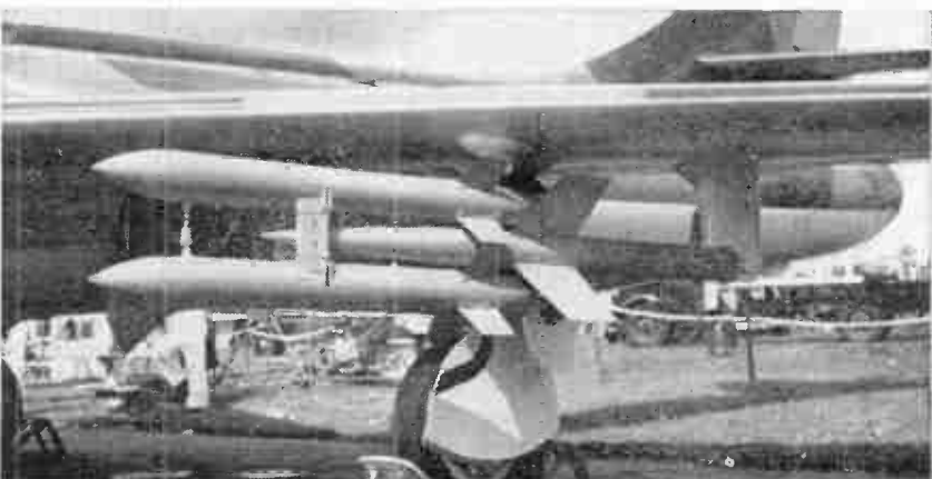
The Fairey Fireflash, an air-to-air guided missile, was put on show to the public for the first time when mounted under the wing of a Hawker Hunter F.4 fighter
