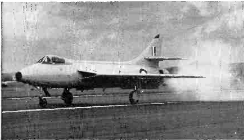
Rolls-Royce displayed a Hawker Hunter fighter fitted with a device that shortens its landing run by a third: the jets come out sideways and forwards instead of backwards
