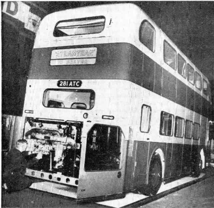
The Leyland Atlantean double-deck bus, seating seventy-eight passengers, is likely to go into service soon on the streets of Glasgow: its diesel-engine is at the rear
