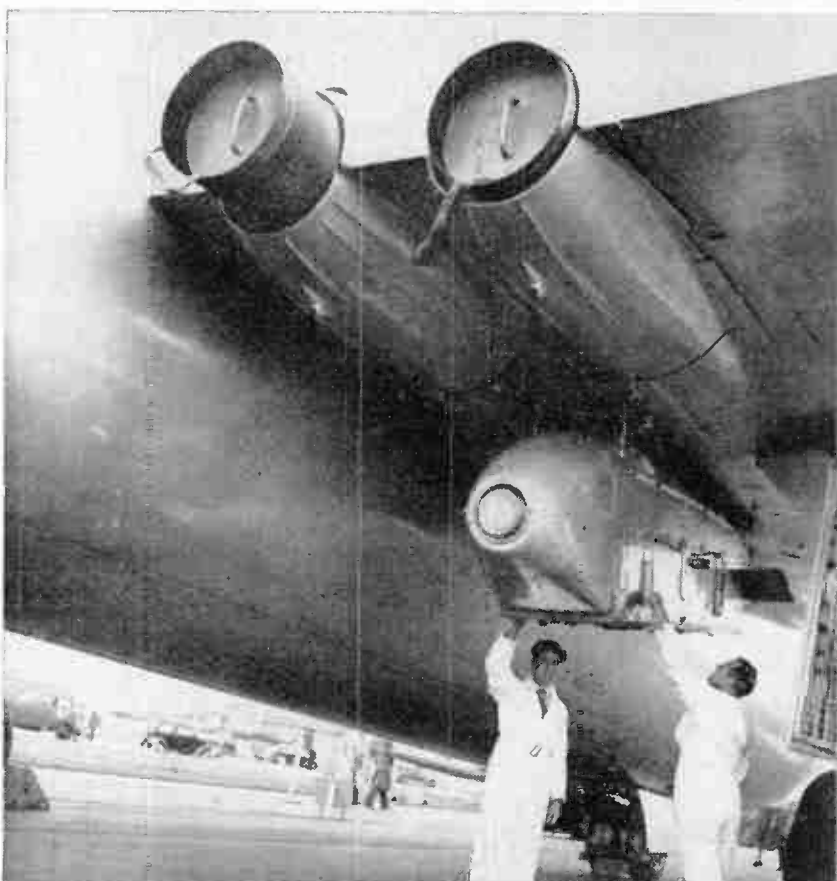
De Havilland Super-Sprite rockets fitted to a Vickers Valiant give the aircraft a shorter take-off, and can then be jettisoned; they are ready for squadron service
