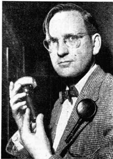
Pocket-size geiger counter for use in workshops where radio-activity is likely
