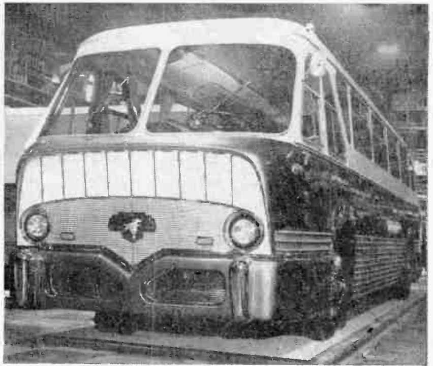
A 150-horse-power British chassis combines with an Italian body in the Worldmaster luxury coach, earlier models of which are already operating in twenty countries
