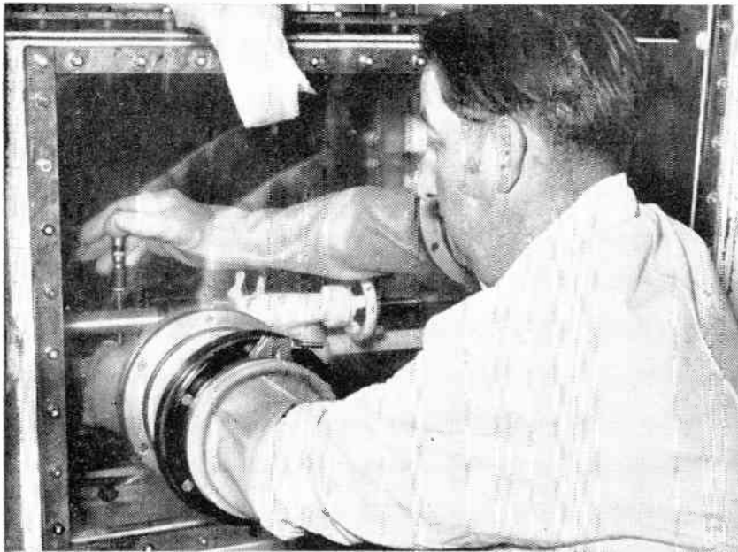
Not a man from Mars but a Harwell technician wearing a protective 'frog-suit' while he works in a highly radio-active area; the picture below shows how a glass-walled glove-box enables a lathe and a micrometer to be used on radio-active material
