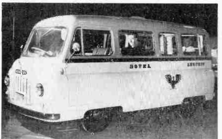
A British answer to the Continental type of small bus—the Morris Minibus, seating thirteen people, costs £625, and its 1½-litre engine develops forty-two horse-power
