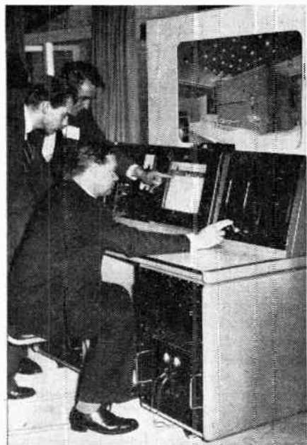
Students watching a lecturer demonstrating a reactor simulator, on which the future controllers of atomic reactors are trained
