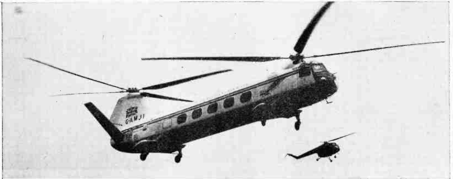
The Bristol 173, a twin-rotor helicopter designed to carry twelve to fourteen passengers. It is being used by British European Airways for development flying
