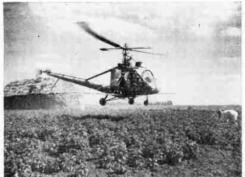
A helicopter in action spraying potatoes in Norfolk with an anti-blight fungicide: the machine operates only three to four feet from the ground
