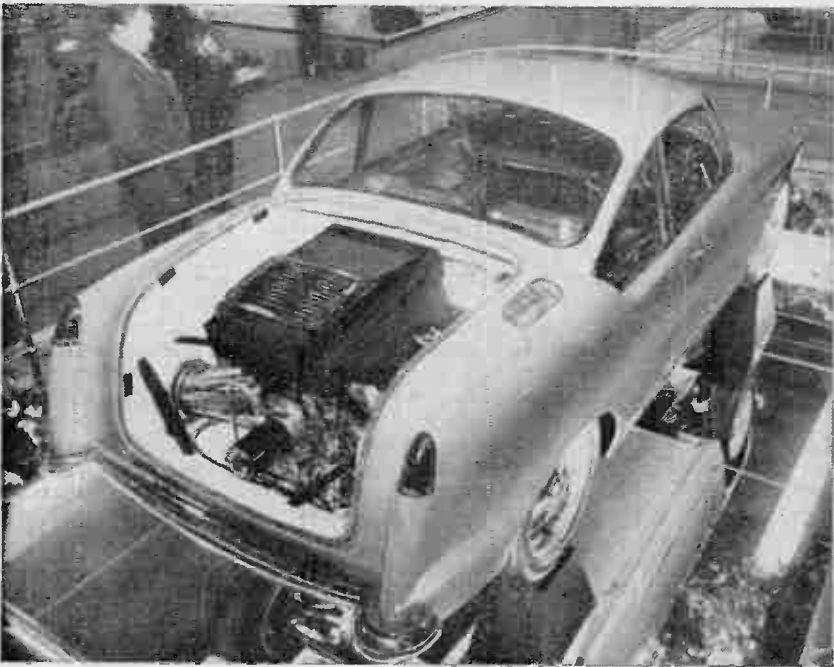
A glimpse of the future—a Rover prototype with its gas-turbine engine at the rear
