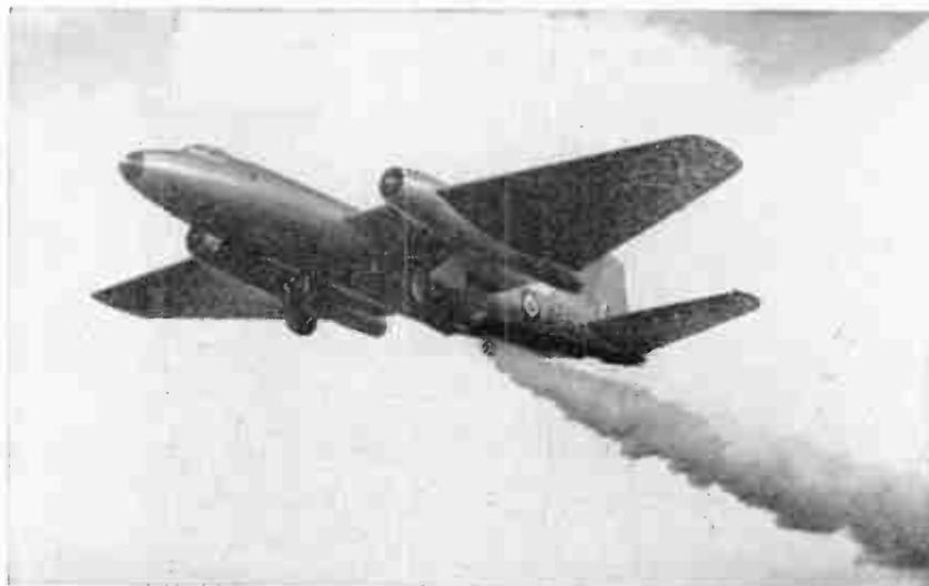
A Canberra bomber demonstrated a Napier Scorpion rocket-motor using liquid propellants, to be used to give fighters more speed and manoeuvrability at great heights
