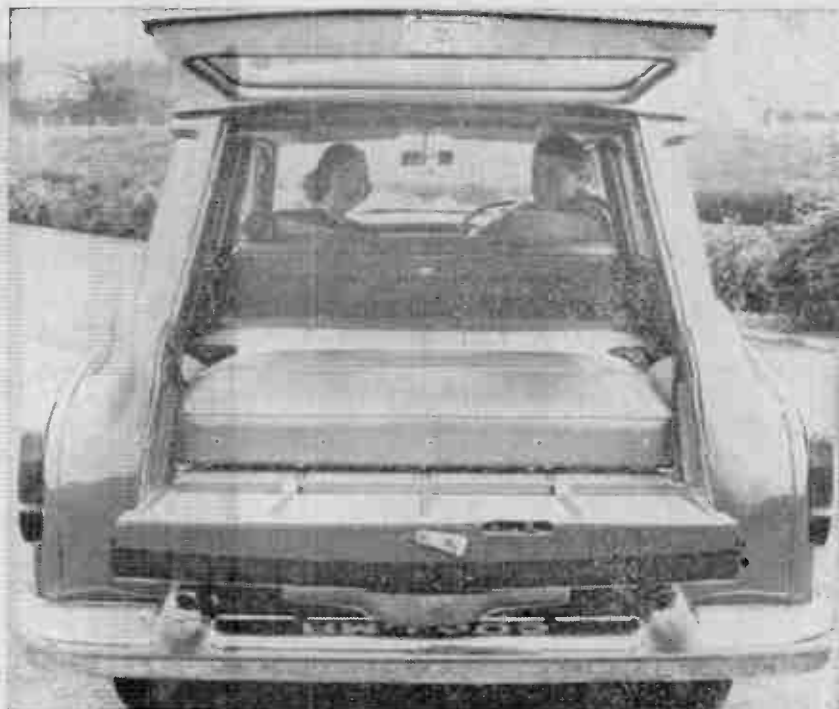
Vauxhall were showing several re-styled models: the estate-car version of the Velox can be fitted with a rear seat that converts into a bed 70 inches long and 42 wide
