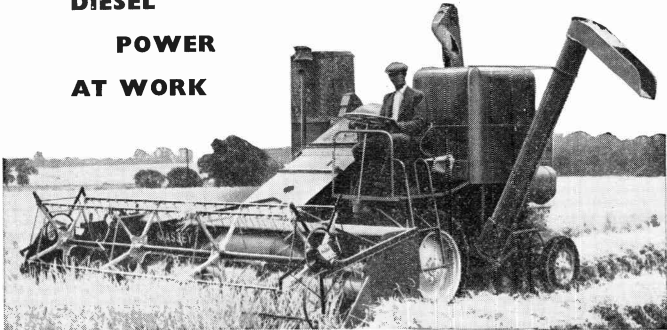
On the farm Perkins Diesel engines offer greater power, easier starting, greatly reduced fuel and maintenance cost. This is a Massey-Harris 780 Combine Harvester fitted with a Perkins L4 TA type diesel engine.
