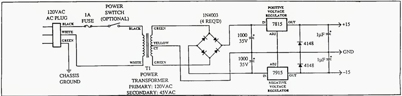
Figure 2. The power supply schematic
