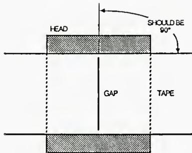
Figure 2. Azimuth alignment
