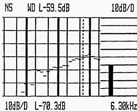
Figure 3B. S/n analysis at 15 in/sec A-weighted
