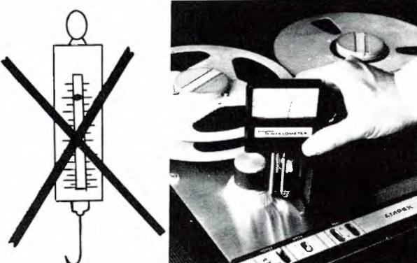
The Tentel tape tension gage is designed to diagnose problems in your magnetic tape equipment. Throw away your fish scales (or put them in your tackle box where they belong). The TENTELOMETER will measure tape tension while your transport is in operation, so you can "see" how your transport is handling your tape . . . smooth, proper tension for quality recording? or oscillating high or low tensions causing pitch problems, wow and flutter?
