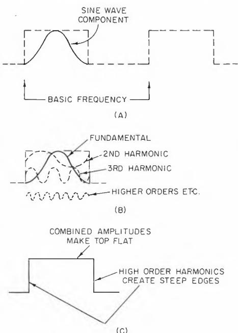
and trailing edges of the pulse. When phasing is correct, then so is the waveform of each of these harmonics. All of the amplitudes will combine with the fundamental sine wave to produce a perfectly flat top to the pulse. Since the pulse amplitude does not change during the time of the flat top passage, this flat top represents a d.c. component in the signal.
