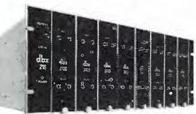
187 4-channel switchable record/playback noise reduction system
