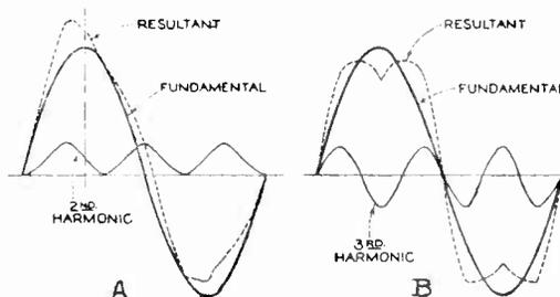
Figs. 7A and 7B - TWO TYPES OF WAVES CONTAINING ODD HARMONICS WHERE IN ONE CASE (7A) THE ODD HARMONIC LIES ENTIRELY ON ONE SIDE OF THE ZERO AXIS WHILE IN THE OTHER (7B) IT IS SYMMETRICALLY ABOUT THIS AXIS.
