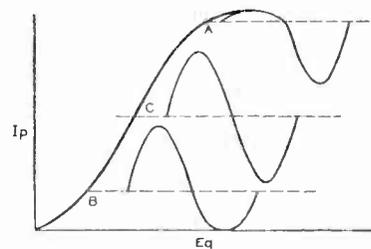
Fig. 10 - CURVES TO ILLUSTRATE PLATE CIRCUIT DISTORTION.
