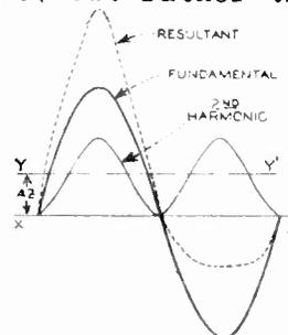
Fig. 5 - CURVES SHOWING THE PRESENCE OF A STRONG 2ND HARMONIC WITH THE FUNDAMENTAL.
