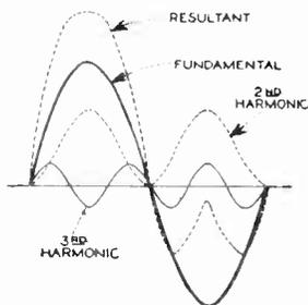
Fig. 8 - THE RESULTANT WAVE OBTAINED BY THE COMBINATION OF A FUNDAMENTAL, A THIRD AND SECOND HARMONIC
