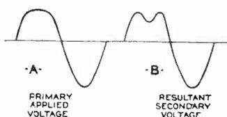
Fig. 12 - CURVE "B" IS THE RESULTANT DUE TO PRESENCE OF A DISTORTED WAVE
