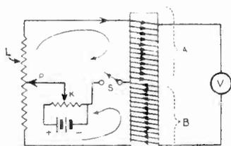
Fig. 14 - VOLTAGE IS APPLIED TO THE COIL BY MEANS OF POTENTIOMETERS.
