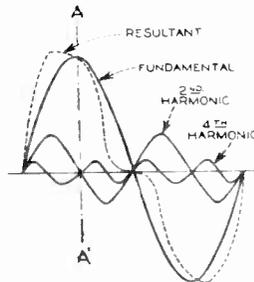
Fig. 4 - SHOWING A DISTORTED WAVE COMPOSED OF THE FUNDAMENTAL, 2ND AND 4TH HARMONIC FREQUENCIES.
