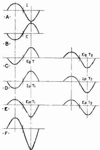
Fig. 23 - CURVES ILLUSTRATING VOLTAGES ACROSS VARIOUS TRANSFORMER WINDINGS.
