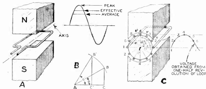
Fig. 2 - THESE FIGURES SHOW THE POSITION OF A WIRE LOOP IN A MAGNETIC FIELD, AND CURVES INDICATING THE VALUE OF VOLTAGE GENERATED AT THE VARIOUS POSITIONS OF THE LOOP.
