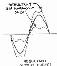
Fig. 22 - DEPICTING TOTAL VOLTAGE GENERATED ACROSS PRIMARY OF OUTPUT TRANSFORMER.
