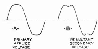
Fig. 13 - THIS TYPE OF WAVE CONTAINS ONLY ODD HARMONICS
