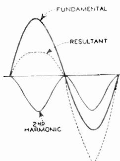
Fig. 6 - DEPICTING THE PRESENCE OF A STRONG 2ND HARMONIC, BUT  $180^\circ$  OUT OF PHASE IN COMPARISON TO FIG. 5.
