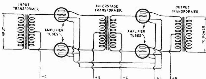
Fig. 24 - SCHEMATIC DIAGRAM SHOWING TWO STAGES OF PUSH-PULL AMPLIFICATION.
