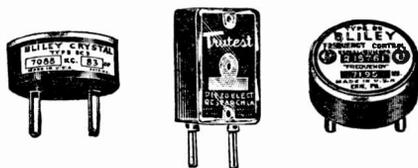
FIG. 14. Typical crystal holders. These are plugged into sockets in the same manner as radio tubes, and can be removed or interchanged in a few moments whenever it is necessary to change the carrier frequency of a transmitter.
