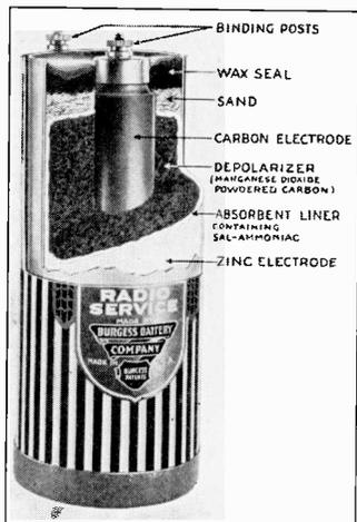
FIG. 9. Cut-away view showing construction of a dry cell.
