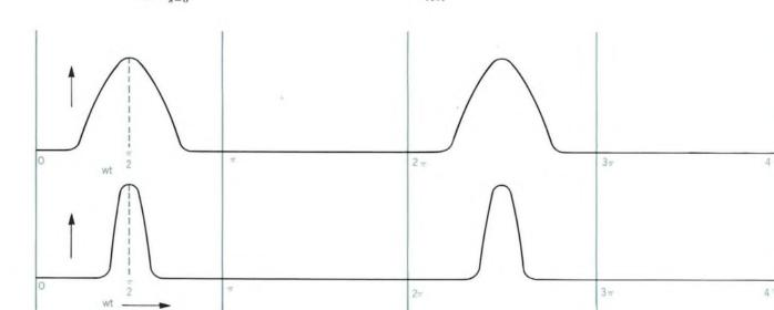
Figure 3 — Waveforms of Plate and Grid Current Drawn for Class C Operation Shown in Figure 2.
