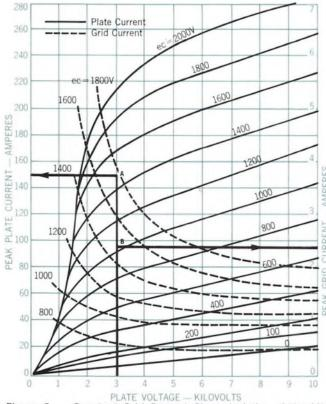
Figure 6 — Constant Grid Current Characteristics of the ML-8618.
