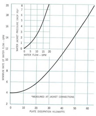
Figure 2 — Cooling Characteristics — ML-6696
