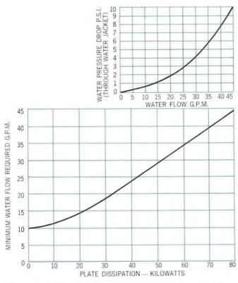
Figure 11 — ML-8618 Anode Water Cooling Characteristics.
