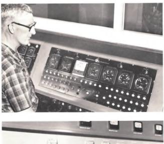
t the console of a 500 kW Continental transmitter, adjustment is made for the desired operating power in this case, as shown below: 15 kV, 52 amperes. Continental Electronics Doherty's similar to this are in service for the VOA both here and in Europe. At Munich, for example, a 1 megawatt (carrier power) transmitter using ML-5682's has been in service for nearly 15 years. (An extensive description of this transmitter may be found in CATHODE PRESS, Volume 10, Number 1, 1953.)
