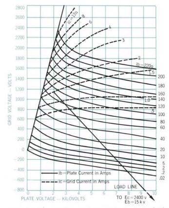
Figure 7 — Constant Current Characteristics for the ML-8618.
