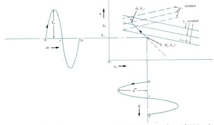
Figure 2 — Graph of Constant Current Characteristics Showing Operating Line and Sinusoidal Plate and Grid Voltages for Class C Operation.
