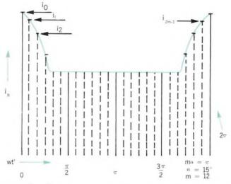
Figure 4 — Waveform of Plate Current Showing Shift in Time Axis to Make  $i_{\rm h}~(\omega t')$  an Even Function, and Division into 15 Intervals.
