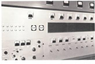
Control panel of the General Electric vapor-cooled 250 kW transmitter. Extremely compact for its power capability, this new transmitter employs five ML-7482 triodes; two as modulators, one in the second intermediate power amplifier position; and two as rf power amplifiers. (An extensive description of this transmitter may be found in CATHODE PRESS, Volume 19, Number 1, 1962.)
