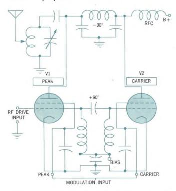
Figure 1 — Simplified Diagram of High Efficiency Screen Modulated Amplifier.
