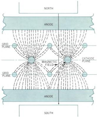
Figure 1 — Conventional Electrode Structure Showing Approximate Use of Cathode Emissive Area.
