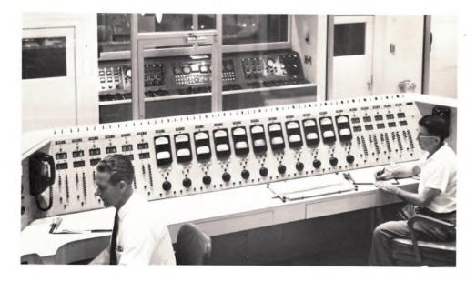
A ntenna selection controls (to indicate the combinations of antennas and transmitters in use; preset conditions for next change are also indicated) and indicators as well as individual transmitter control monitor are found in the transmitter control console. A typical panel has: % Modulation Meter, Audio Input VU Meter, Audio Gain Control with preset line key, Filament, Ready and Plate Indicator Lights, Modulation Peak Indicator Flasher, and an SWR Warning Light.
