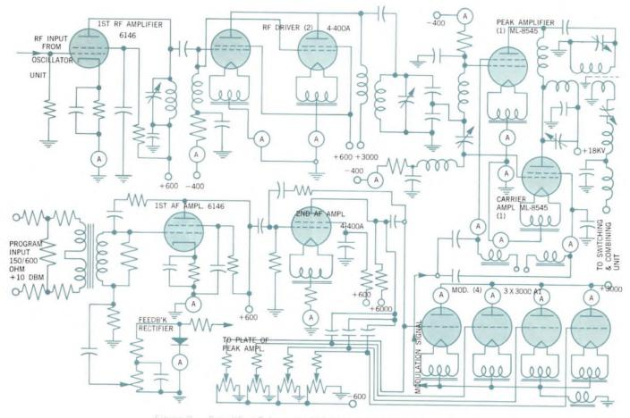
"gure 2 — Simplified Schematic 250 kW MF Broadcast Transmitter.
