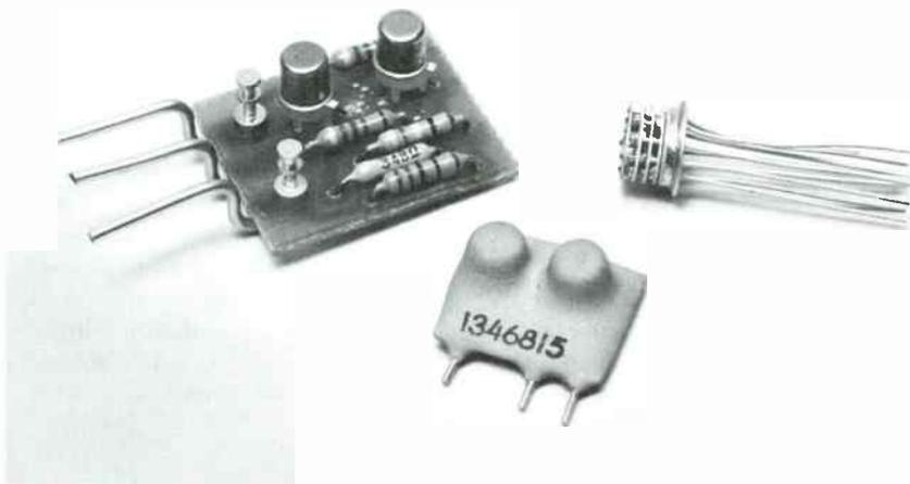
Figure 7. Lenkurt-built negative resistance (left) for channel filter studies compared to Centralab package and Sylvania IC version. About actual size.
