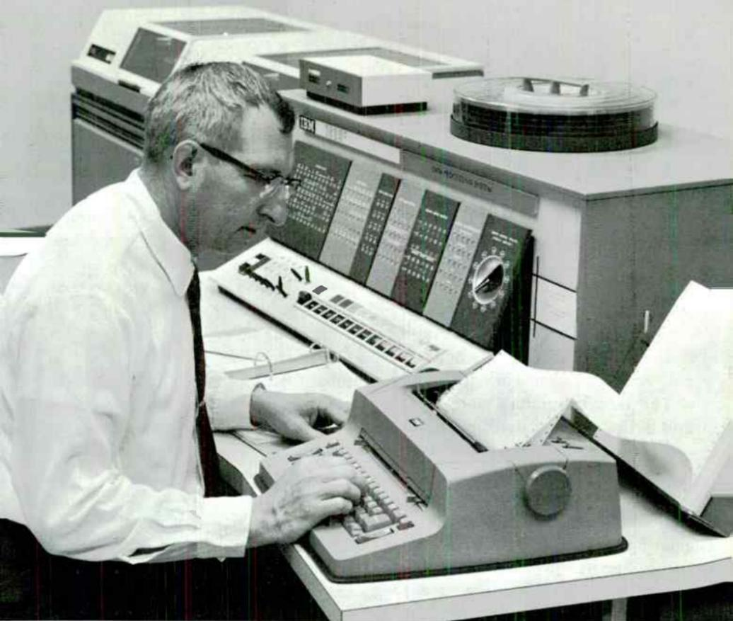
*Figure 1. Typical scientific computer is the IBM 1620 II, used at Lenkurt. Behind the central processing unit is magnetic disc storage drive.*
