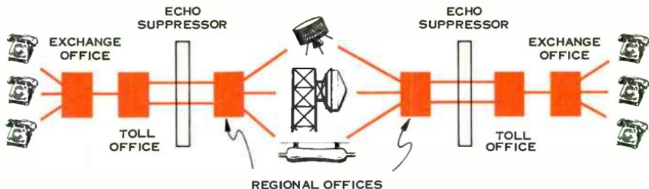
Figure 1. Telephone path through exchange, toll and regional offices. Echo suppressor is located at the beginning of 4-wire toll circuits.
