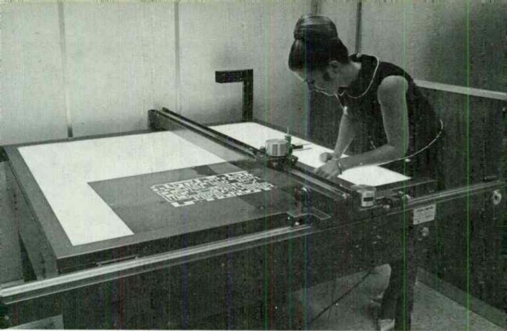
*Figure 1. A precision drafting machine such as a coordinatograph is a “must” for development of microcircuitry. Note the digital light display in the background.*
