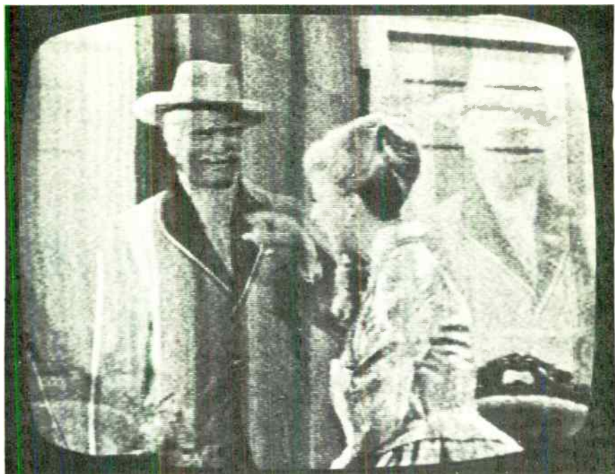
Figure 2. Poor frequency response or other irregularities lead to distortion of various sorts in the reproduced picture. Echoes usually result from non-linearities in baseband frequency characteristic, or from multipath transmission. Since transmission errors are rarely as bad as this exaggerated example, sensitive test methods are required to permit accurate evaluation of quality.
