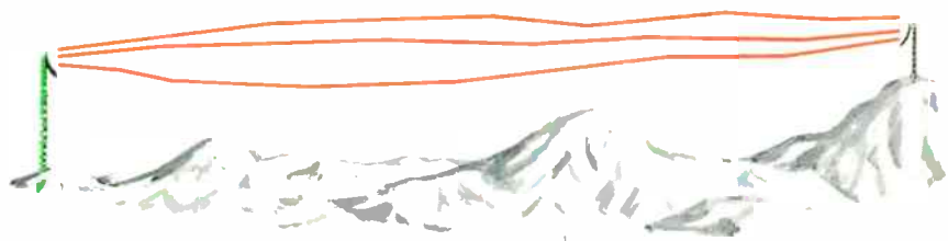
Figure 3. Irregularities in atmosphere cause radio beam to break up into several components traveling different paths. Those which manage to reach receiving antenna will have traveled paths of different lengths, causing phase cancellation.
