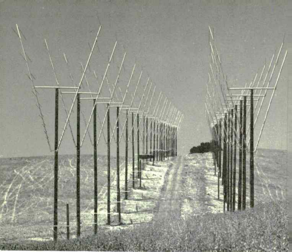
Figure 3. An array of 50 log-periodic antennas used for radar explorations of the sun, moon, and planets.
