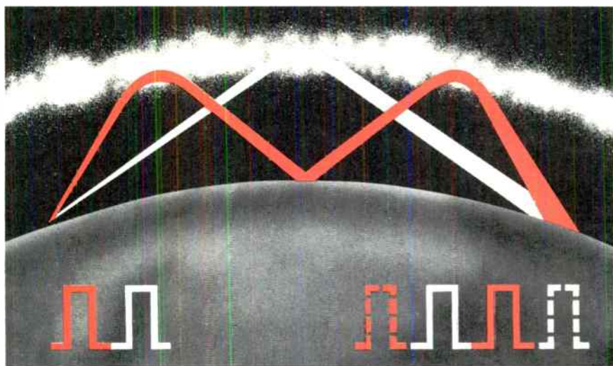
Figure 1. Multipath effect occurs when signals take different paths from transmitter to receiver, arriving in a different time relationship.
