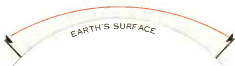
Figure 2. In normal atmosphere, beam is gently deflected toward earth by gradual change in density of atmosphere above the earth's surface.
