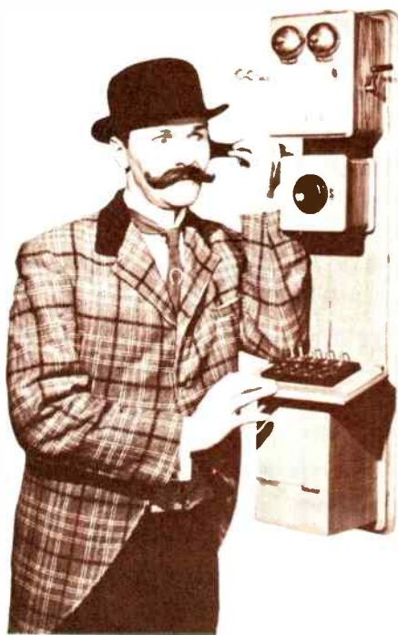
Figure 1. First automatic telephone employed both magneto and push-button signaling for establishing desired connection.
