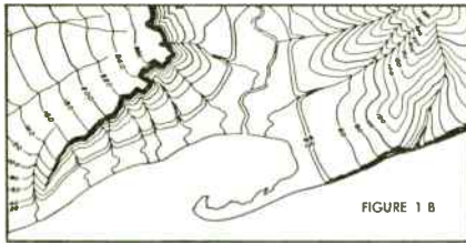
FIGURE 1. Contour maps provide an excellent data source for preparing profile charts. Figure 1B is a contour map of the area sketched in Figure 1A.
