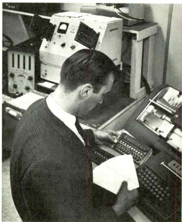
Figure 6. Transistors used in Lenkurt products are life-tested to determine their quality and operating characteristics. At certain intervals the essential parameters of each transistor are measured and recorded. Photograph shows 20 transistors being checked automatically. Analog measurements are fed into analog-to-digital converter and then into a keypunch machine which punches the data into a card for future processing. Punched cards are used in computer programs to predict transistor failure rates or MTBF, and end-of-life.
