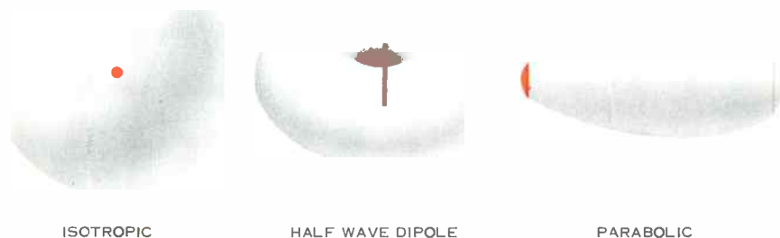
Figure 1. Idealized representation of radiation patterns produced by isotropic, dipole, and parabolic reflector antennas.
