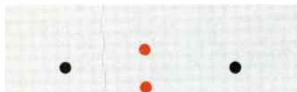
Figure 1. Two pairs arranged so that both conductors of each pair are equidistant from disturbing conductors. Such arrangements are impractical for many pairs.
