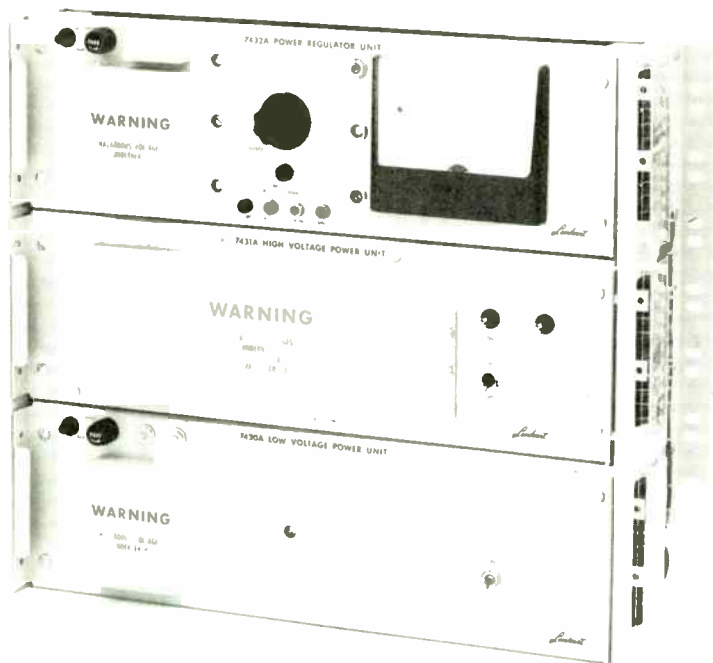
Figure 1. Reliability is the most important consideration in designing communications power supplies, followed by stability, regulation, and freedom from hum and ripple. Microwave power supply shown employs semiconductor rectifiers, magnetic amplifiers for voltage regulation. Plug-in construction permits each unit to be replaced instantly, provides superior access to internal components.
