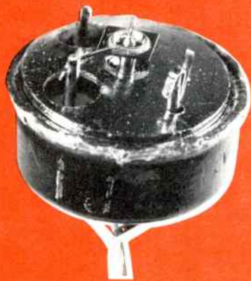
Figure 1. Typical junction transistor (from which upper case has been removed), shown here greatly enlarged. The square plate is only about 1/50 inch (1/2 mm.) on each side; the junctions which comprise the central spot and the ring are extremely small.
