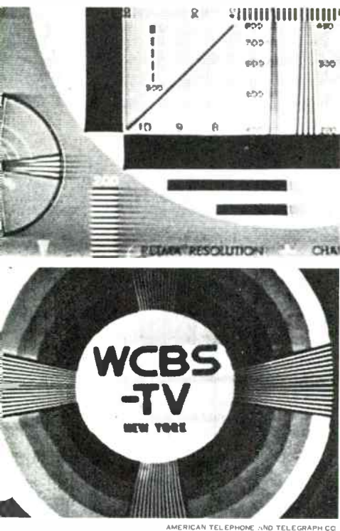
Figure 6. Examples of streaking caused by poor response at the lower frequencies — positive streaking above, negative streaking below.
