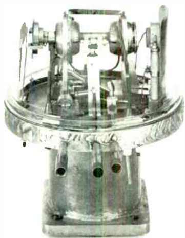
Fig. 1. First successful klystron produced microwave oscillations at about 2300 megacycles. Device incorporated water cooling and an ingenious fluorescent radio frequency detector. Shafts on front are micrometer controls for adjusting resonator positions and coupling between resonators during operation.
