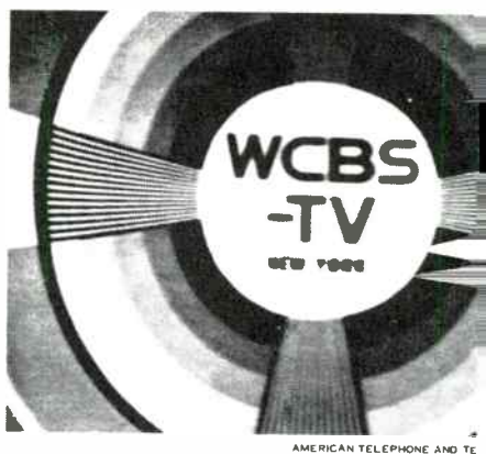
Figure 3. When bandwidth is reduced, horizontal definition is impaired without affecting vertical resolution. Compare the horizontal and vertical converging lines in this example in which bandwidth is limited to about one mc.
