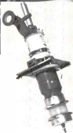
Fig. 6. World's most powerful electron tube. Twenty-one of these klystrons are used in the Stanford linear accelerator. Researchers say that although tubes are each capable of 30 million watts peak power, they are usually operated at "only 20 million watts." Microwave energy from klystrons is used to accelerate particles in evacuated tube on left to speeds approaching that of light. Screened area in background contains pulse network for one klystron.
